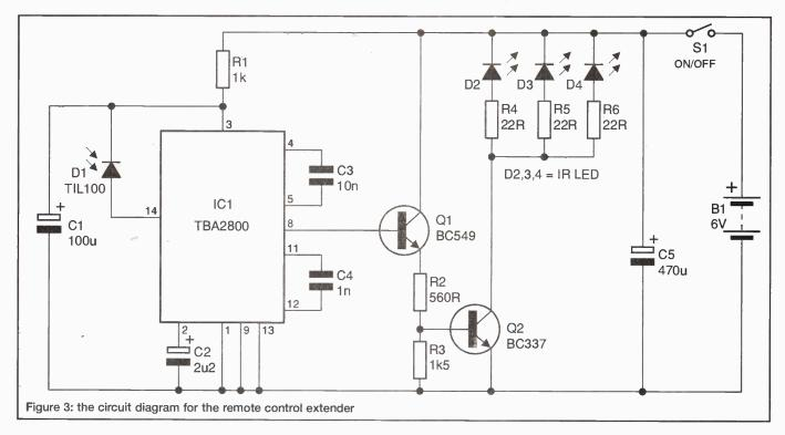
current is strictly limited. A buffer amplifier is therefore used to boost the output current to a level that can drive three infra-red LEDs properly.
