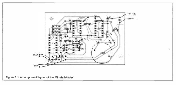
Note that they are all CMOS components and, as such, are liable to damage due to static charge on the body. To avoid any problems, touch something which is earthed - such as a water tap - before handling the pins. Adjust RV1 so that the sliding contact is near the centre of the track. Do this by turning the screw one way until clicking is heard - this happens when the wiper is at the end. Count the number or turns until it reaches the other end then set it about half way between these extremes.
