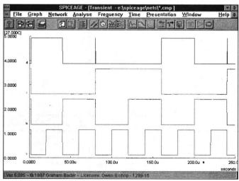
Figure 1: the output of the ripple counter described last month - complete with glitches
