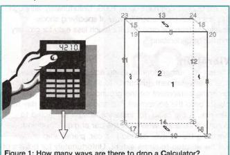
Figure 1: How many ways are there to drop a Calculator? According to Mil Std 810E, there are 26 ways, and equipment must be able to survive drops onto every face, edge and corner.
