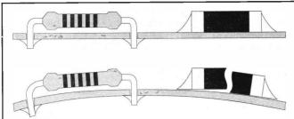
Figure 4: If a surface-mount board does flex, the leadless components may be damaged because, unlike through-hold components, there is no lead to take the strain. But when the pros and cons are evaluated, surface mounting is the clear winner for rugged equipment.
