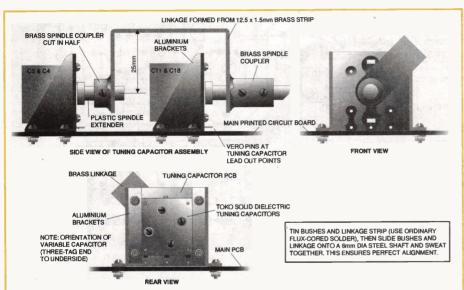
Figure 2: linking two variable capacitors to form a four-gang unit: tin bushes and linkage strip (use ordinary flux-cored solder), then slide bushes and linkage onto a 6mm diameter steel shaft and sweat them together. This ensures perfect alignment.
