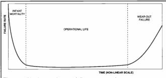
Figure 2: Plotting equipment failure rates against time produces this familiar 'bathtub' curve.
