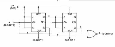
Figure 2: the circuit of a synchronous counter with decoding for state 00
