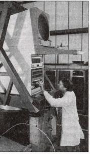
Vibration testing: a sophisticated vibration and shock testing system can take anything from elecronic components to assemblies of up to 2 tonnes in weight. (Seimens Plessey Assessment Services Ltd., Fareham.)
