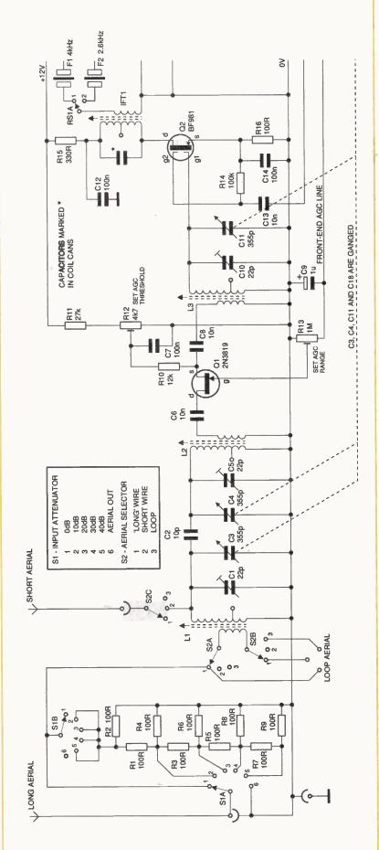
Figure 1a: the aerial selector and input attenuator stages, the RF tuning stage, front-end AGC stage and the mixer stage
