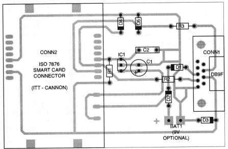
Figure 4: The component layout for the Smart card reader, using the Cannon CCM01-2NO-3 connector.
