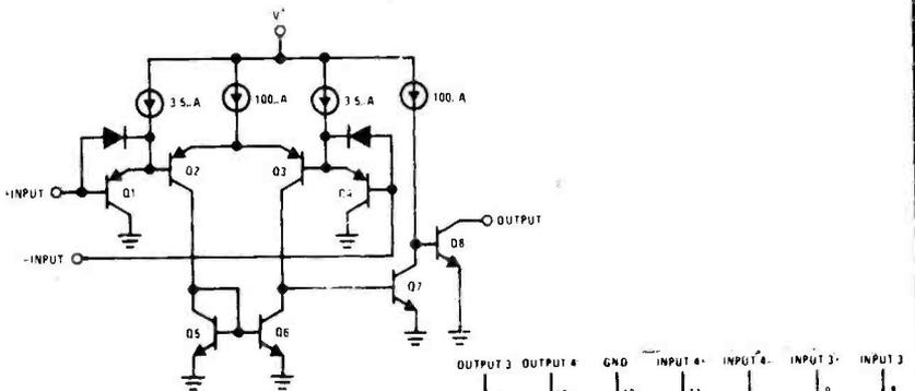
Fig.3. Internal circuitry and pin corrections of the LM339 IC.
