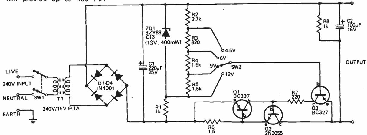
Fig. 1. Circuit diagram of the regulated power supply.
