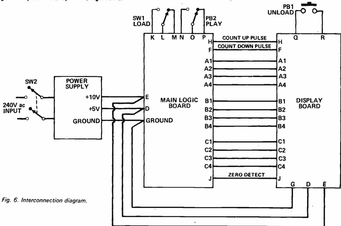
Fig. 6. Interconnection diagram.
