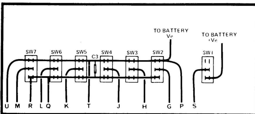
Fig. 5. Switch interconnection diagram. Note that C3 is mounted across one of the switches.
