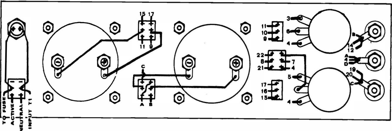
constructed our front panel by sandwiching a line drawing between the chassis and a piece of smoked perspex. This provides a very professional looking appearance. An even better finish can be obtained by using an anodised aluminium panel, and these may be available from parts suppliers.
