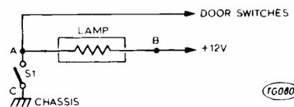
Fig. 3. (Right) Guide to the interior light connections.
