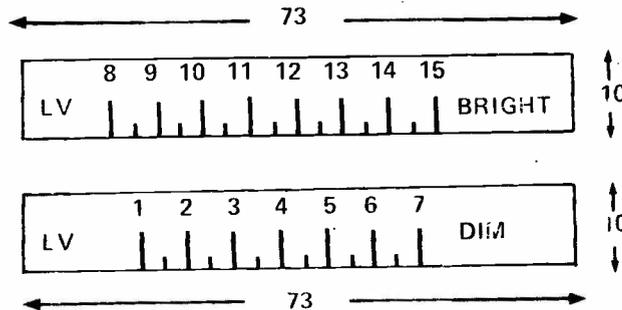
Fig. 8. The scales for calibrating the slider pot.
