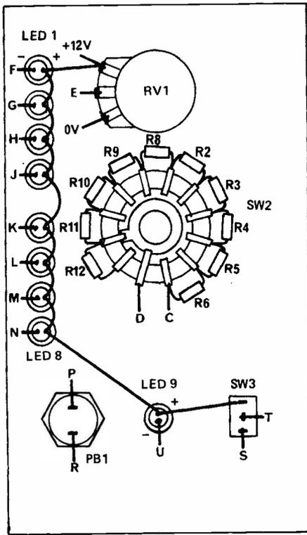
Fig. 3. Front panel wiring details.
