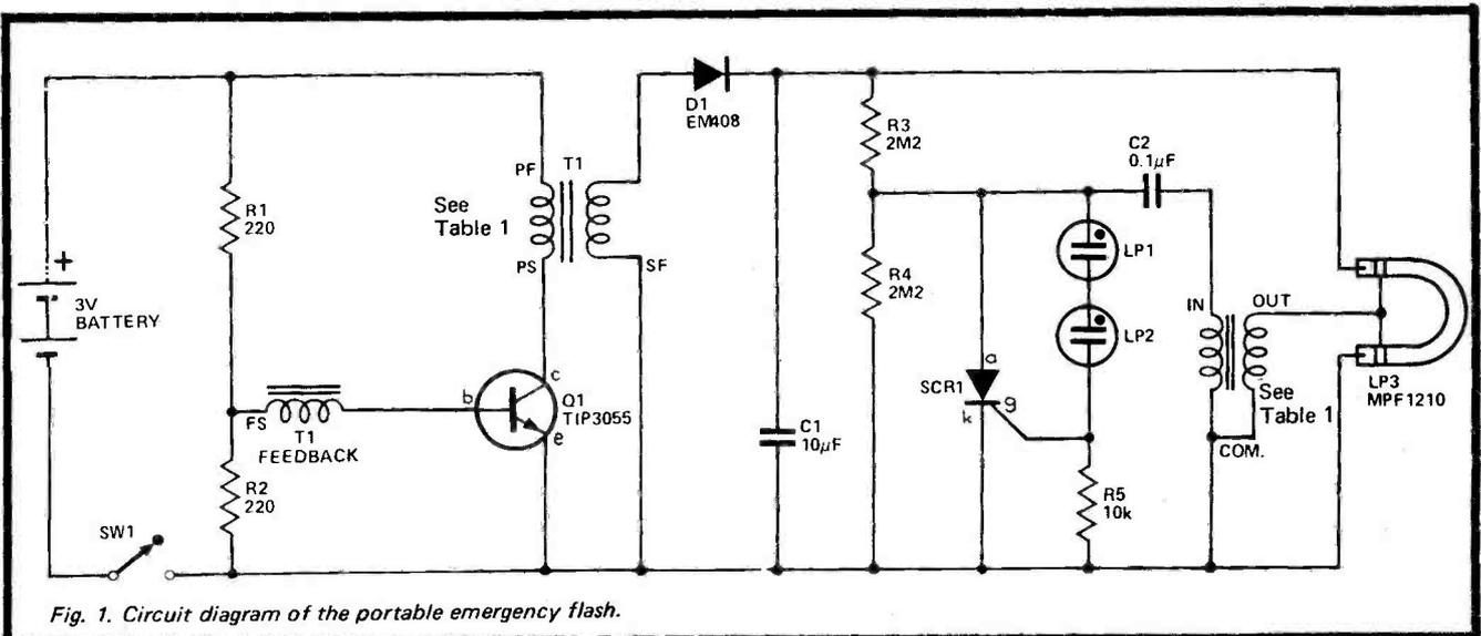
Fig. 1. Circuit diagram of the portable emergency flash.
