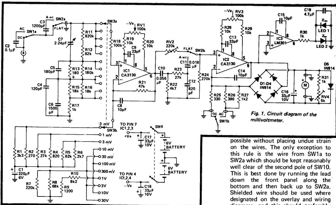
Fig. 1. Circuit diagram of the millivoltmeter.
