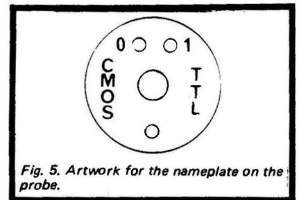
Fig. 5. Artwork for the nameplate on the probe.
