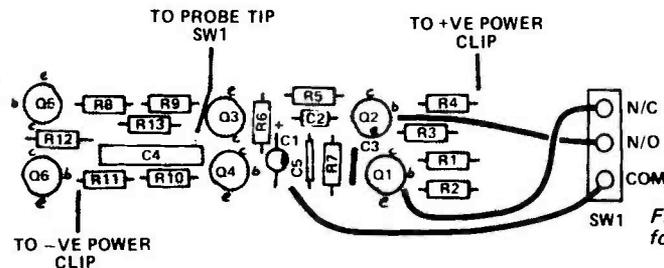
Fig. 3. Component overlay for the pulser.
