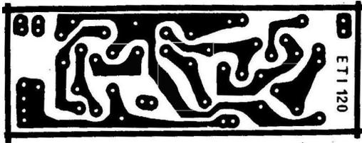
Fig. 2. Printed circuit board for the logic probe (2 required). Full size 23 x 66 mm.
