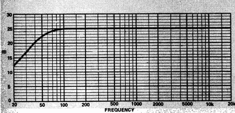
Fig. 4. Response of charge amplifier. Roll off at low end is designed to compensate for rising response of cartridge in this area.
