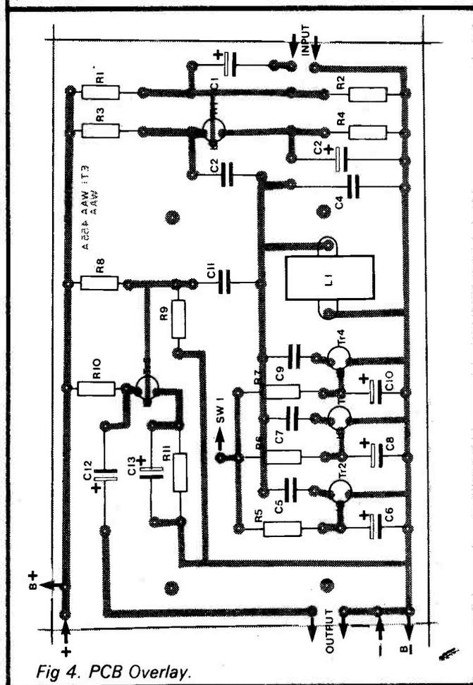
Fig 4. PCB Overlay.
