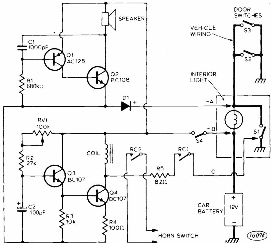
Fig. 1. Complete circuit of the Auto Alarm
