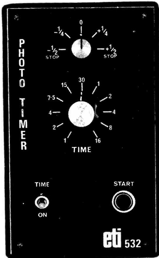
WHEN making multiple photographic prints the repeatability of exposure timing is considerably improved by using an accurate timer.
