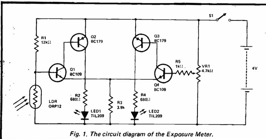
Fig. 1. The circuit diagram of the Exposure Meter.
