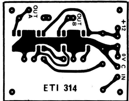
Fig. 2. Printed circuit board. Full size 50 x 65 mm.
