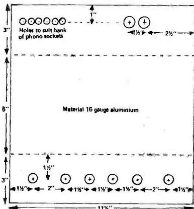
Fig. 7. Metalwork details. The front panel holes are standard  $\frac{3}{16}$ in as are the holes for the bank of phono sockets.  $\frac{5}{16}$ in holes are needed for the DIN speaker sockets.
