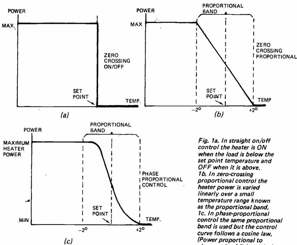
Fig. 1a. In straight on/off control the heater is ON when the load is below the set point temperature and OFF when it is above.
