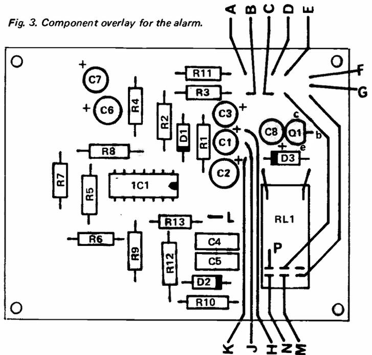
Fig. 3. Component overlay for the alarm.
