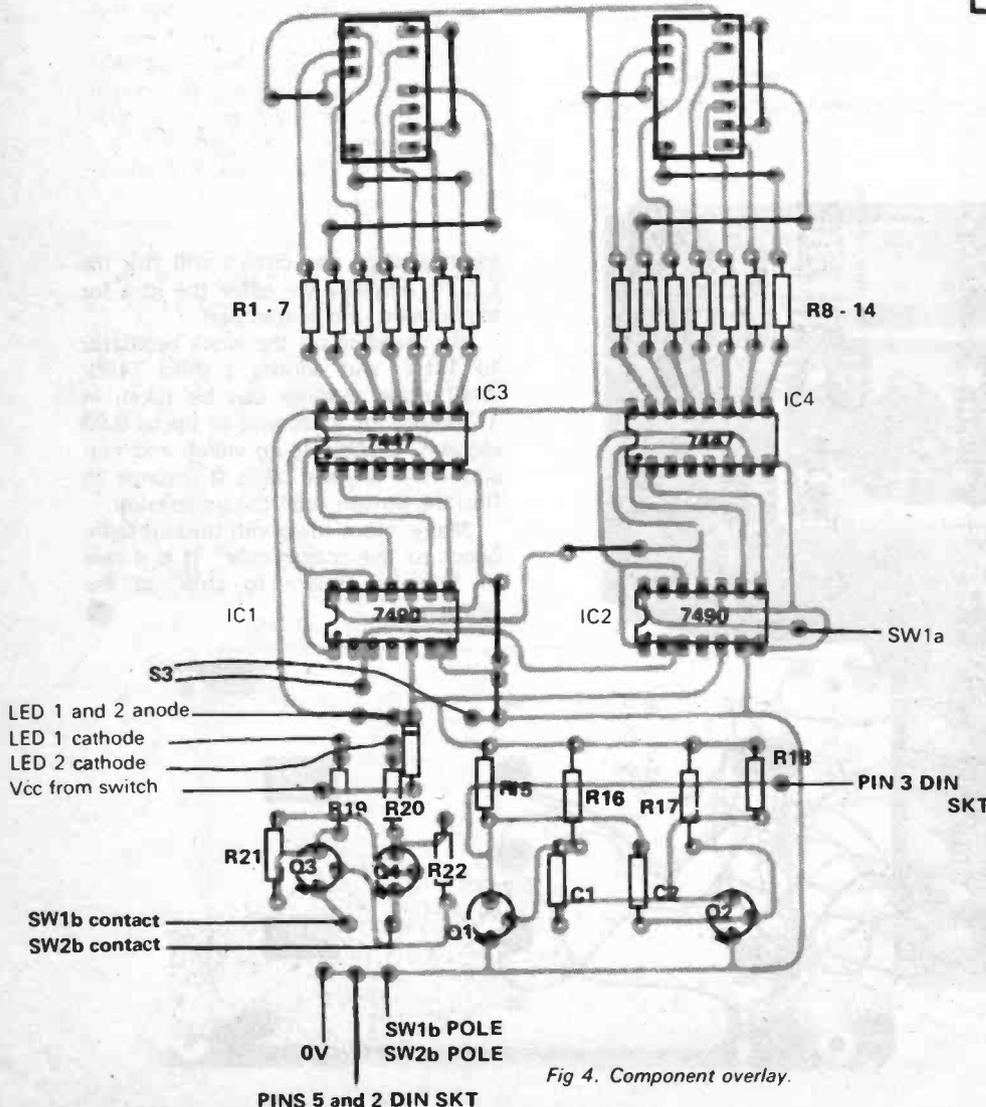
Fig 4. Component overlay.
