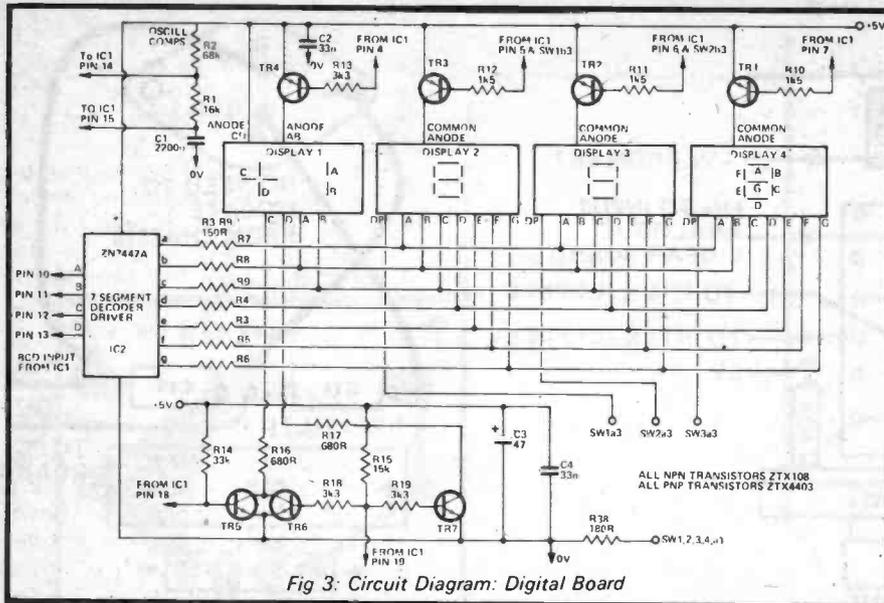
Fig 3: Circuit Diagram: Digital Board
