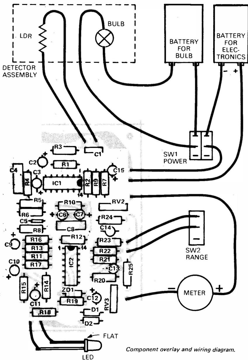
Component overlay and wiring diagram.
