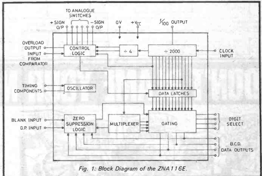
Fig. 1: Block Diagram of the ZNA 116E.
