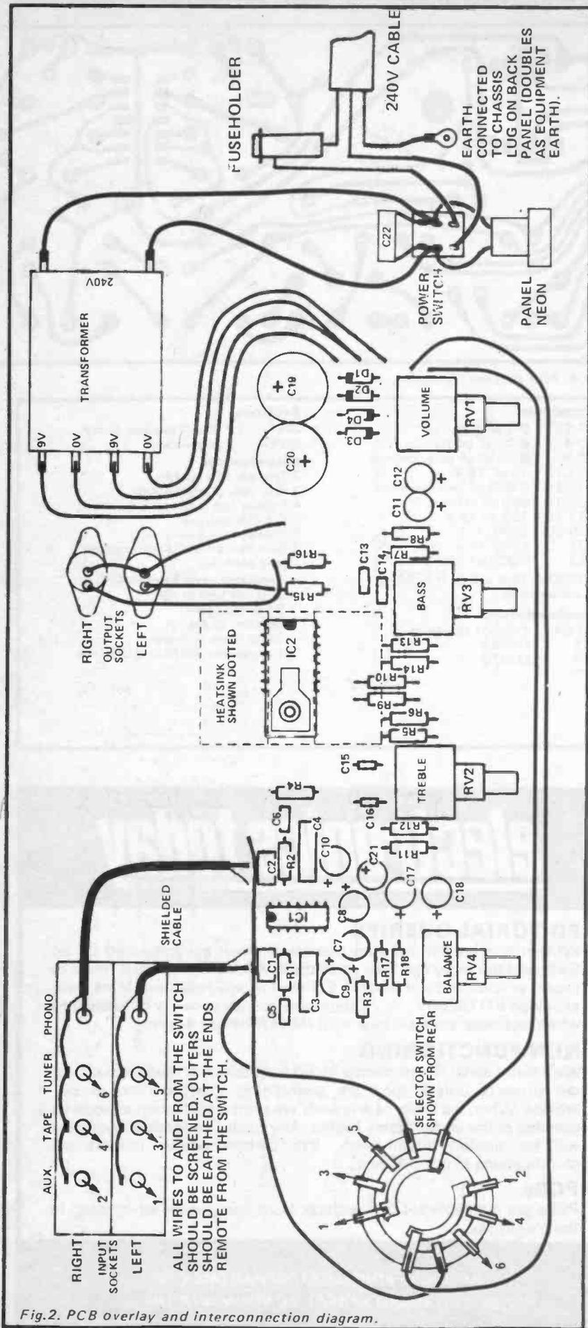
Fig.2. PCB overlay and interconnection diagram.
