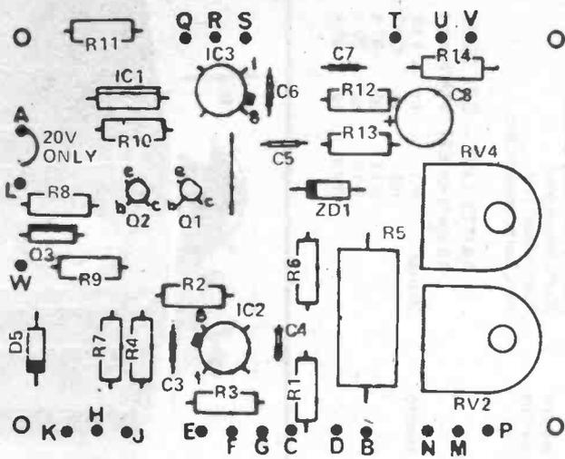
Fig. 3. Component overlay for the printed-circuit board assembly.
