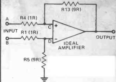
A "balanced" amplifier or differential amplifier has two separate inputs and only the difference between these inputs is amplified. To explain how this works refer to figure, which is a simplified version of the circuit. To make the maths easier we will reduce the gain to nine by making  $R1 = R4 = 1$  and  $R5 = R11 = 9$ . The actual units are not important, only the ratio.
