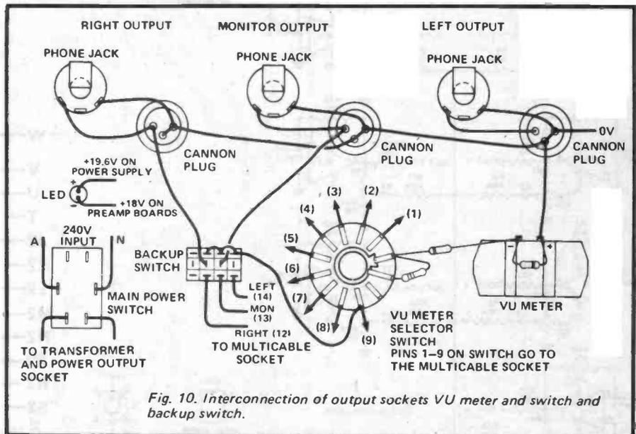
Fig. 10. Interconnection of output sockets VU meter and switch and backup switch.
