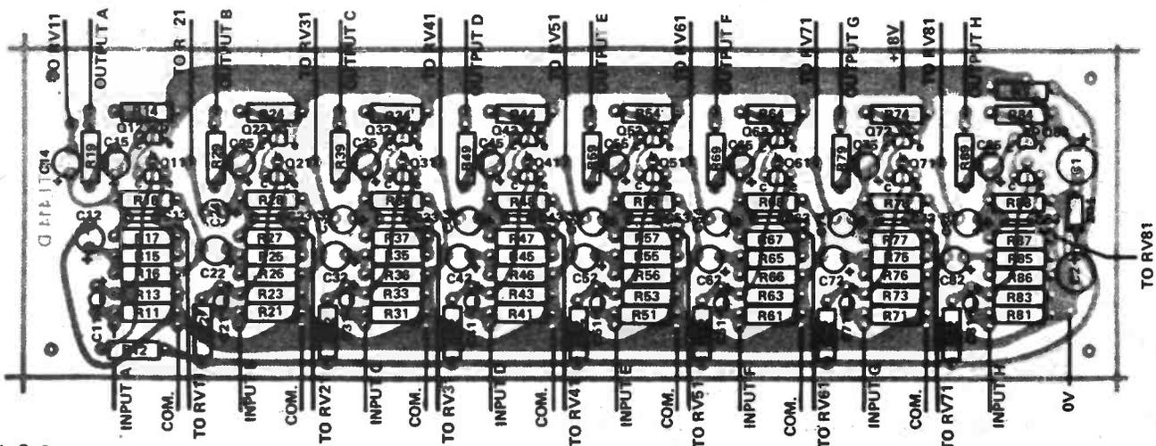
*Fig.2. Component overlay for the preamplifier board.*
