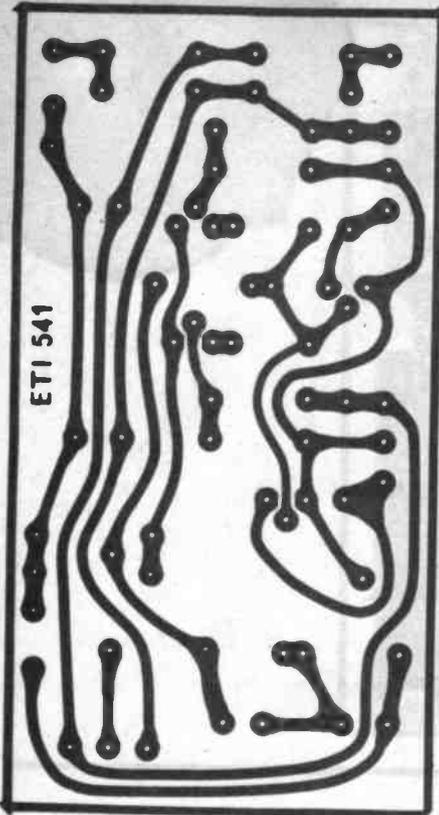
Printed-circuit board layout ETI 541 train controller. Full size 65 x 105 mm.
