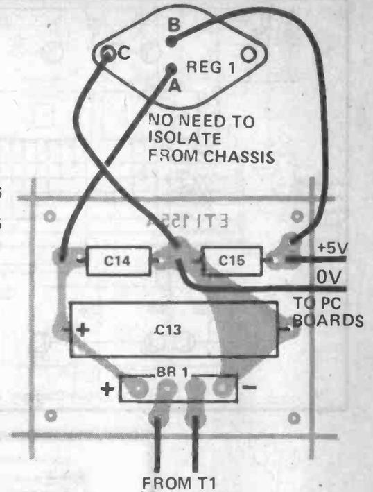
Fig 8: Overlay — Power Supply
