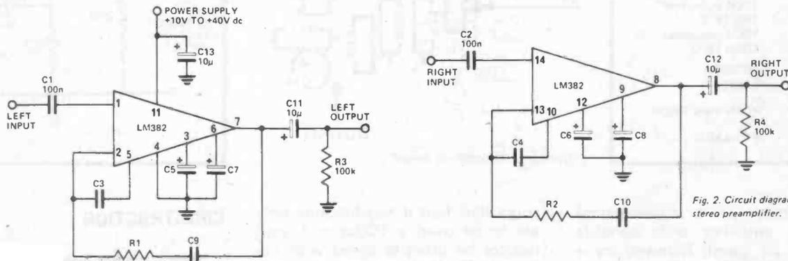
Fig. 2. Circuit diagram of the stereo preamplifier.
