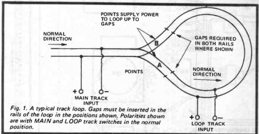
Fig. 1. A typical track loop. Gaps must be inserted in the rails of the loop in the positions shown. Polarities shown are with MAIN and LOOP track switches in the normal position.
