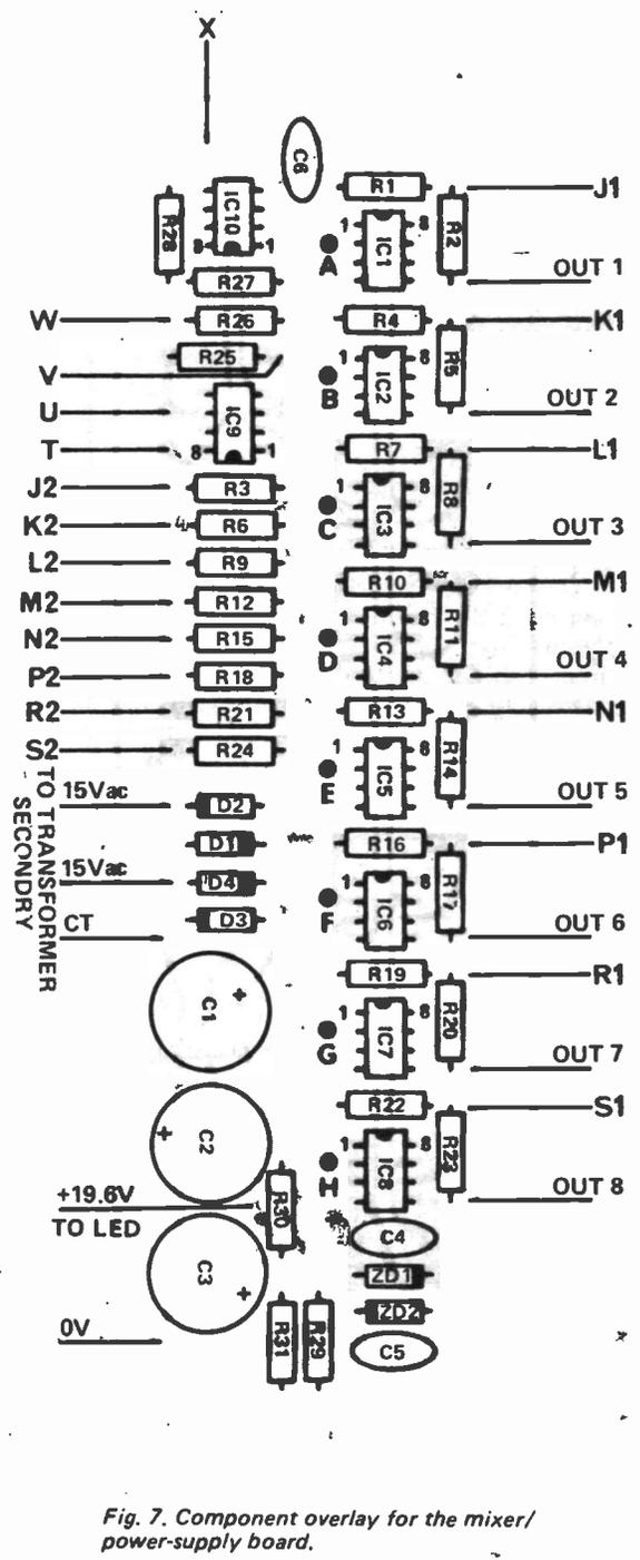
Fig. 7. Component overlay for the mixer/power-supply board.
