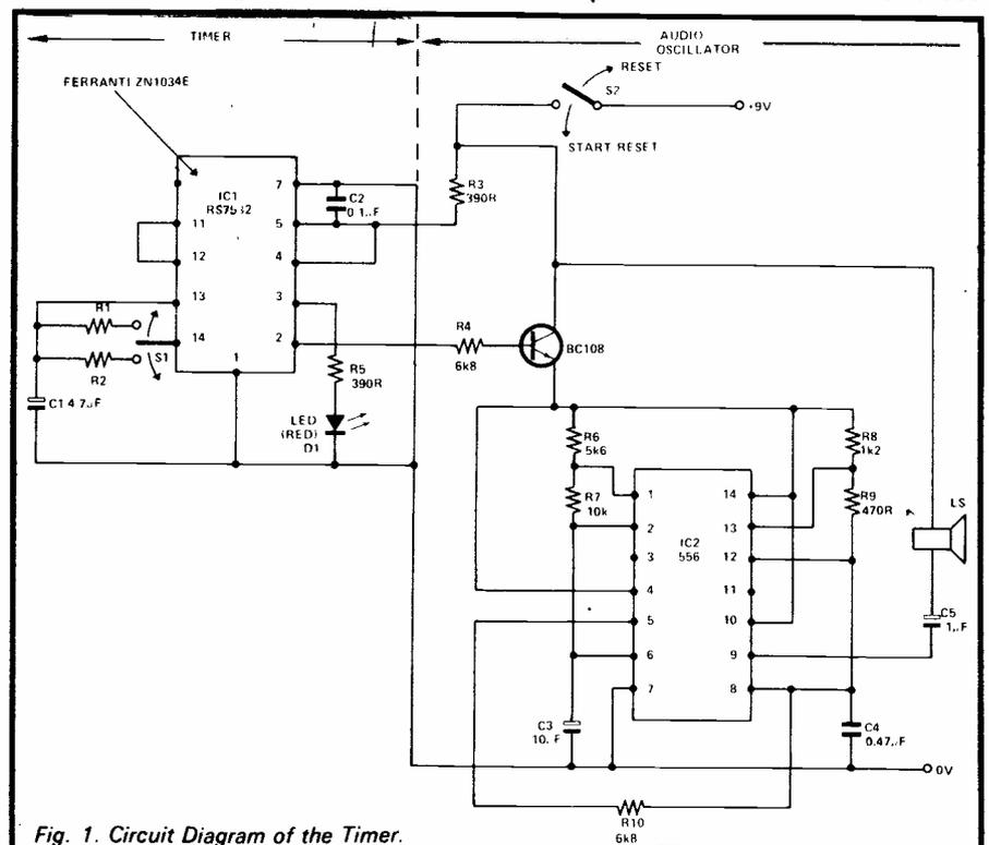
Fig. 1. Circuit Diagram of the Timer.
