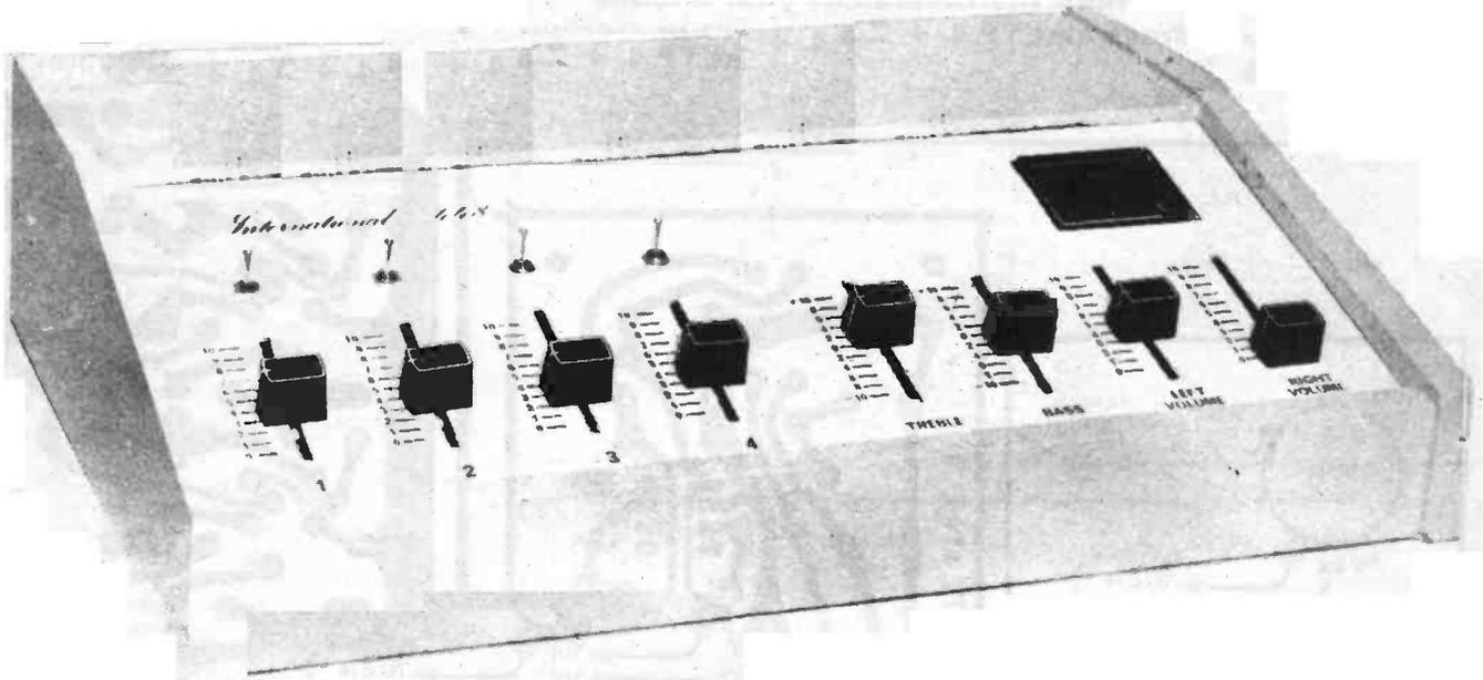
This is a general-purpose mixer project that can be tailored by the constructor, to meet specific needs. Five boards are used in the design; Disco mixer board (448); Mono headphone amplifier (448A); Balanced microphone preamplifier (449); Stereo VU circuit (449A), and General purpose preamplifier (445). Also a simple ceramic cartridge preamp is shown — so simple it can be built on the input sockets!
