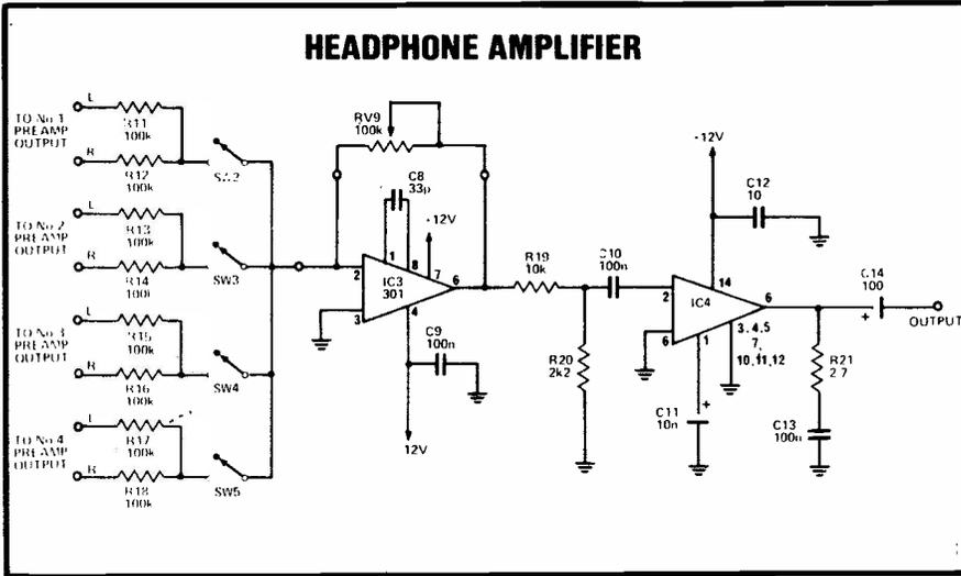
The resistors bridging Left and Right channel outputs are to provide a composite mono signal, without seriously degrading the main mixer stereo separation. The signal is selected by SW2-SW5 and fed to a buffer with variable gain (IC3). The output is then fed to a LM380 power amplifier which drives the monitor headphones.
