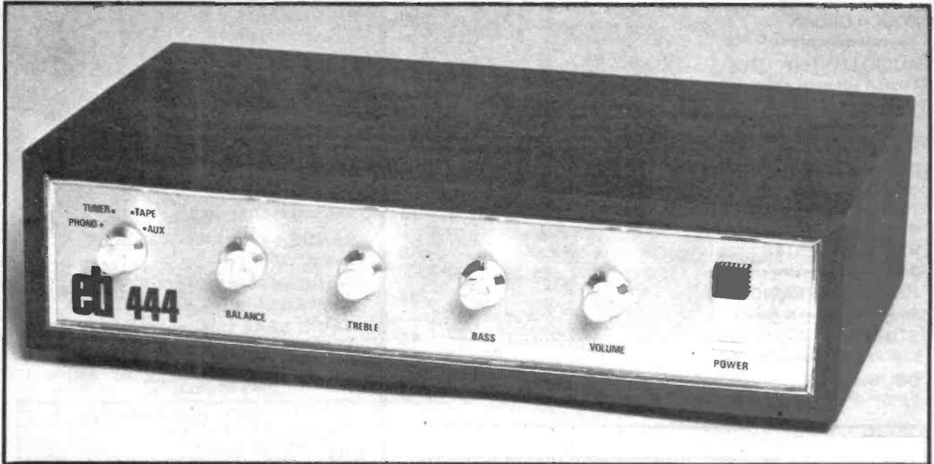
THIS PROJECT UTILISES A NEW advance by IC manufacturers. A few years ago no one would have believed a complete stereo hi-fi amplifier could be made from just two ICs plus a few passive components. Today more and more components are contained within the IC so a power amplifier is as easy to use as an op-amp.
