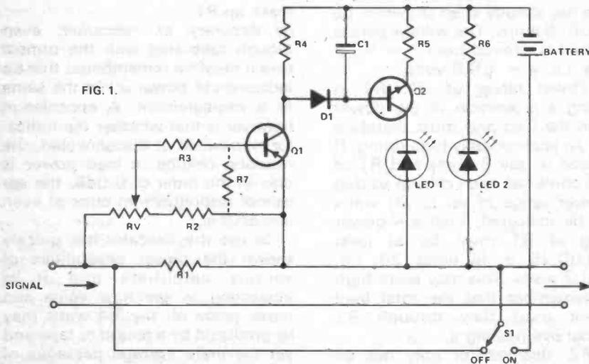
Fig. 1. Circuit of Power Indicator.
