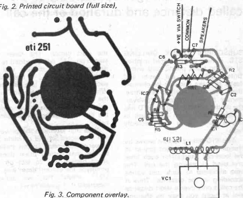
Fig. 3. Component overlay.
