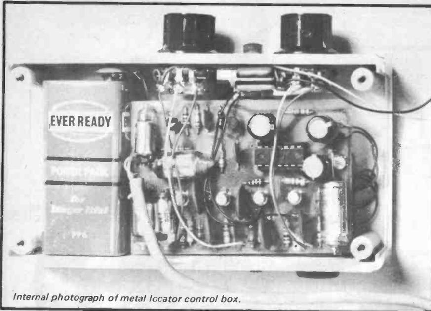
Internal photograph of metal locator control box.
