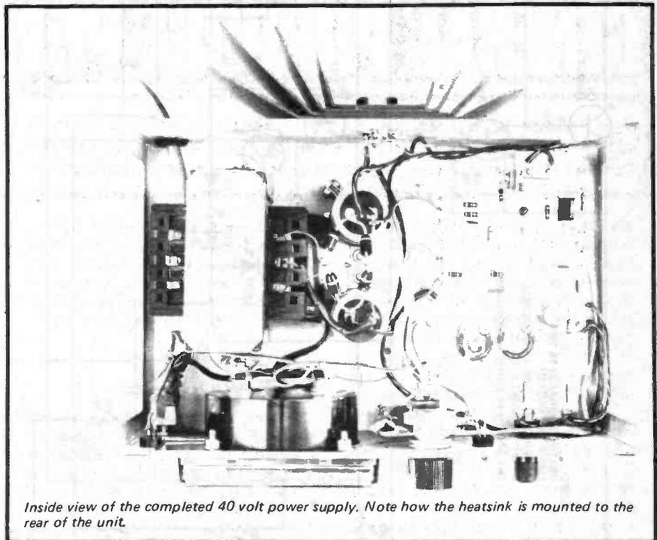
Inside view of the completed 40 volt power supply. Note how the heatsink is mounted to the rear of the unit.
