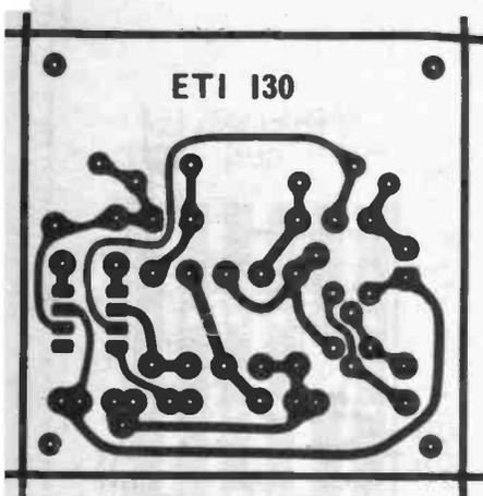
Fig. 4. Printed circuit pattern. Full size 63 x 63 mm.
