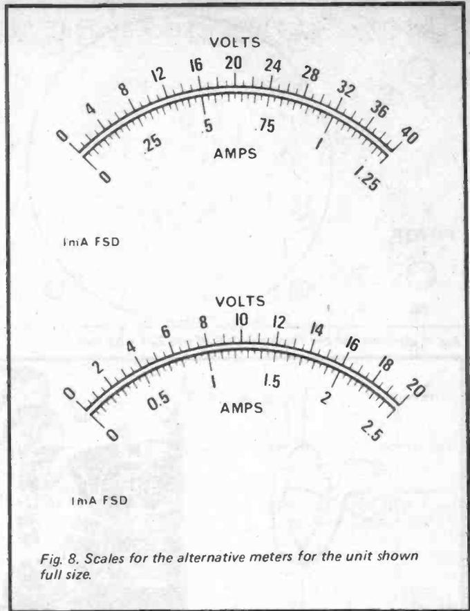
Fig. 8. Scales for the alternative meters for the unit shown full size.
