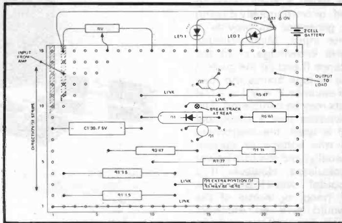
Fig. 3. Veroboard layout to fit Doram module case. Top (non-stripe) side.
