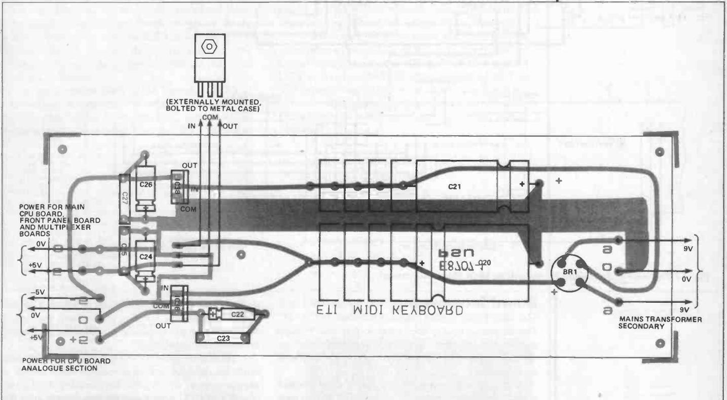
Fig. 15 The component overlay for the power supply board
