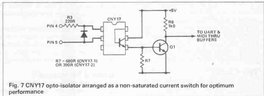
Fig. 7 CNY17 opto-isolator arranged as a non-saturated current switch for optimum performance
