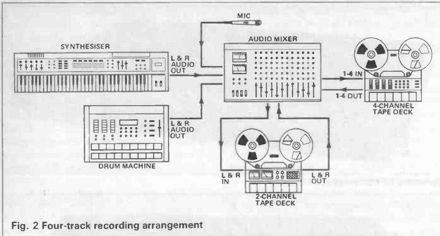
Fig. 2 Four-track recording arrangement
