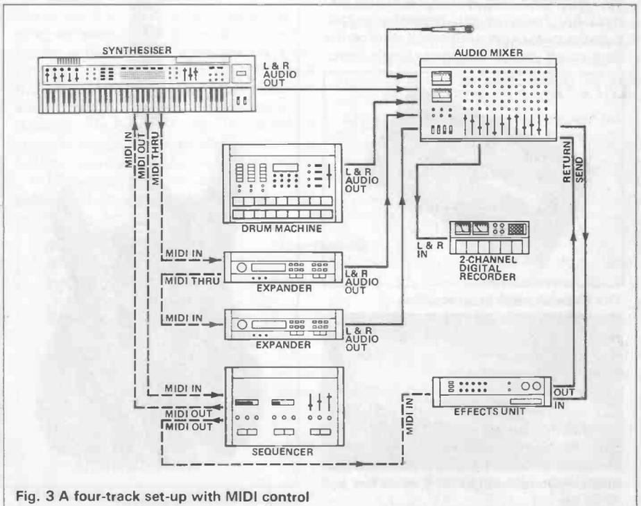
Fig. 3 A four-track set-up with MIDI control
