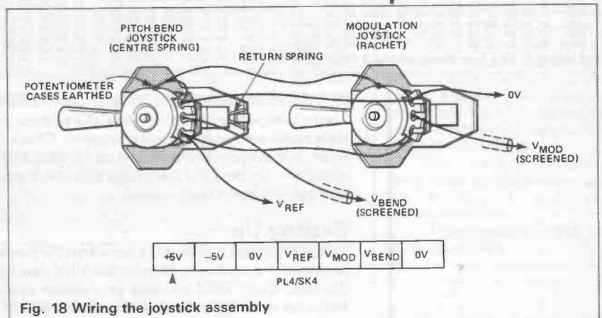
Fig. 18 Wiring the joystick assembly
