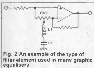
Fig. 2 An example of the type of filter element used in many graphic equalisers
