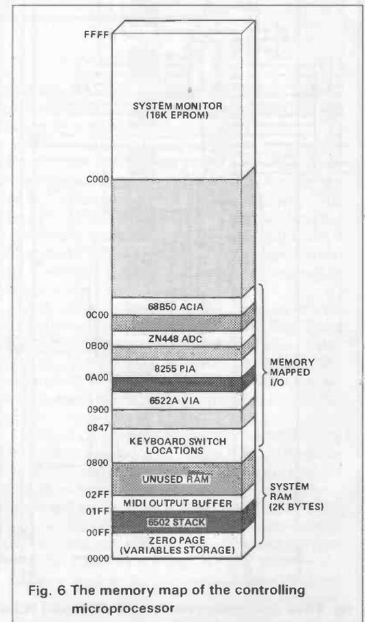
Fig. 6 The memory map of the controlling microprocessor
