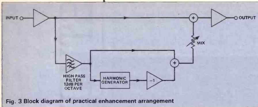
Fig. 3 Block diagram of practical enhancement arrangement
