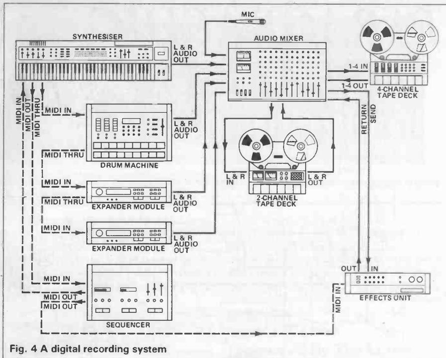
Fig. 4 A digital recording system
