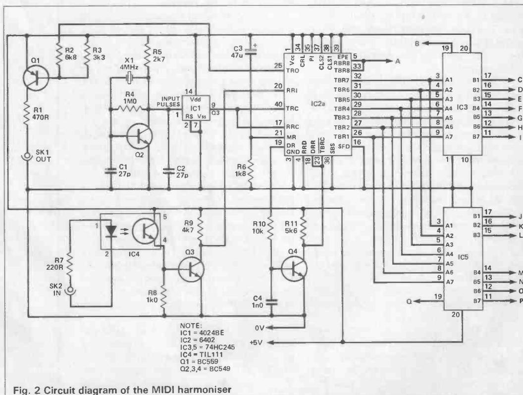
Fig. 2 Circuit diagram of the MIDI harmoniser
