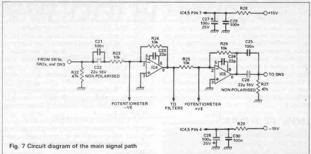
Fig. 7 Circuit diagram of the main signal path
