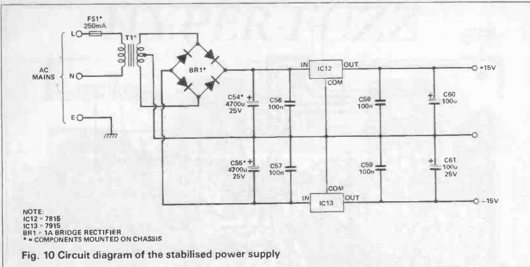
Fig. 10 Circuit diagram of the stabilised power supply
