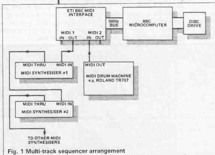
Fig. 1 Multi-track sequencer arrangement
