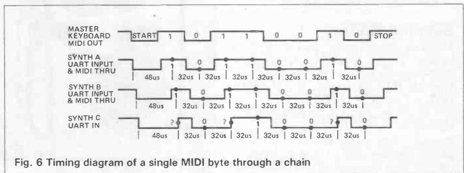
Fig. 6 Timing diagram of a single MIDI byte through a chain
