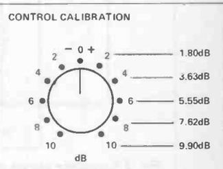
Fig. 15 Calibration of the input level control
