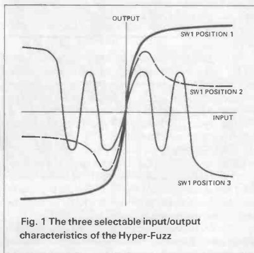
Fig. 1 The three selectable input/output characteristics of the Hyper-Fuzz
