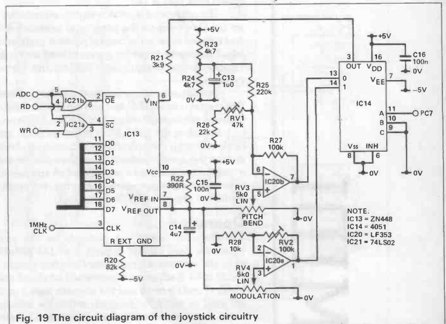
Fig. 19 The circuit diagram of the joystick circuitry
