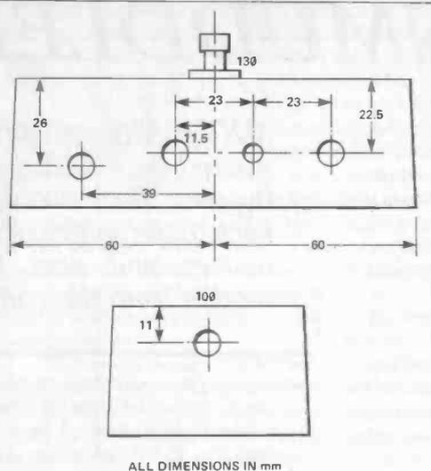
Fig. 3 Drilling the case for the Hyper-Fuzz
