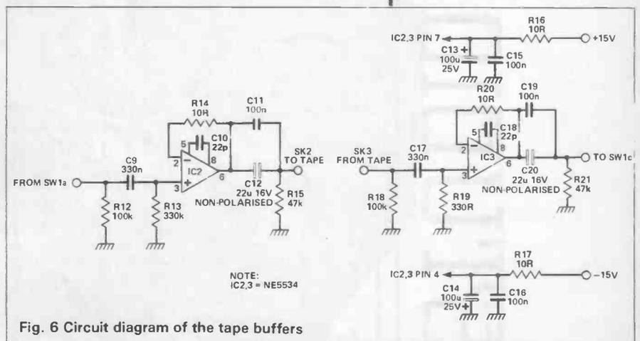
Fig. 6 Circuit diagram of the tape buffers
