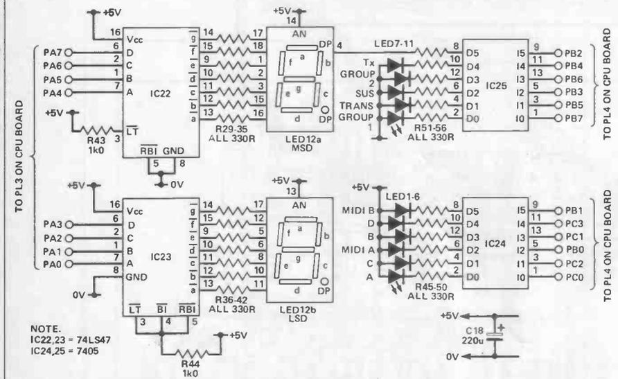
Fig. 12 The circuit diagram for the front panel board
