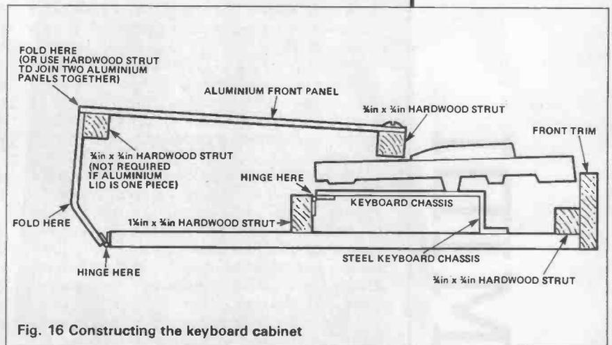
Fig. 16 Constructing the keyboard cabinet
