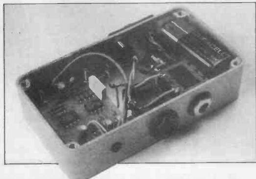
be used for initial testing. Set the power supply to about 4V and connect up. If the LED does not light, then reverse its connections and try again. Once the LED works, increase the voltage until the LED goes off then reduce it until the LED switches on again. Measure the voltage and check that it is about 6.5V. Individual units may vary due to component tolerance, but if the voltage is not acceptable the value of R<sub>13</sub> or R<sub>15</sub> should be changed.
