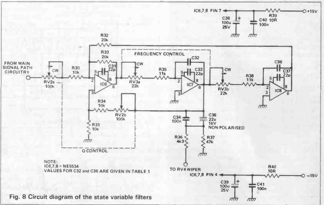
Fig. 8 Circuit diagram of the state variable filters
