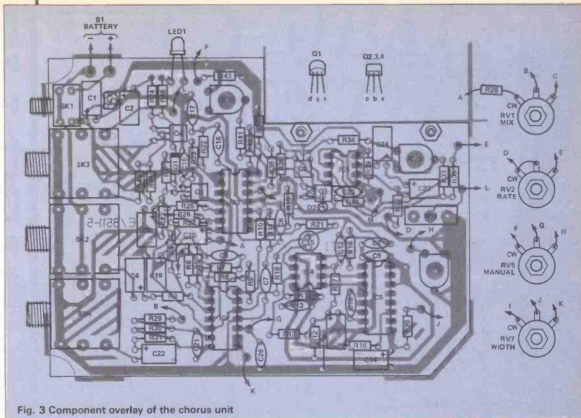
Fig. 3 Component overlay of the chorus unit
