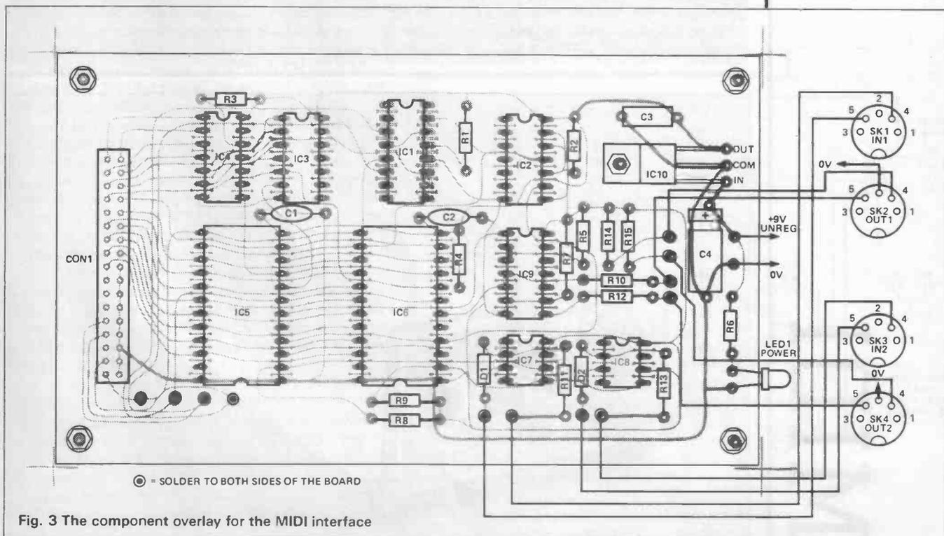
Fig. 3 The component overlay for the MIDI interface
