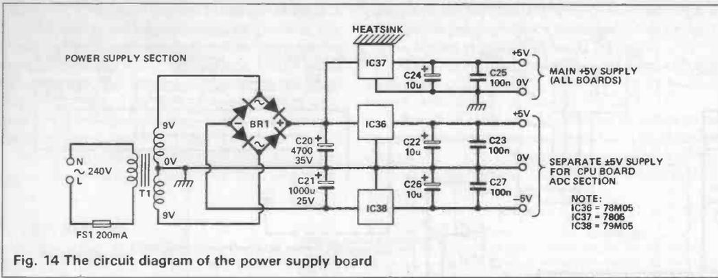
Fig. 14 The circuit diagram of the power supply board
