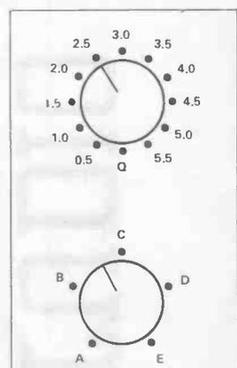
Fig. 16 Calibration of the Q and frequency controls.
