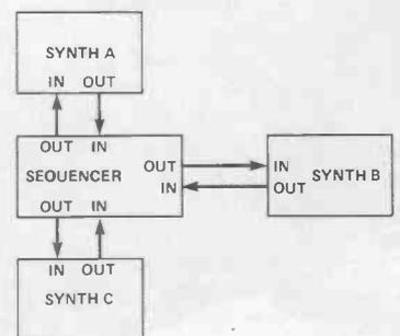
Fig. 3 A multi-socket star connection
