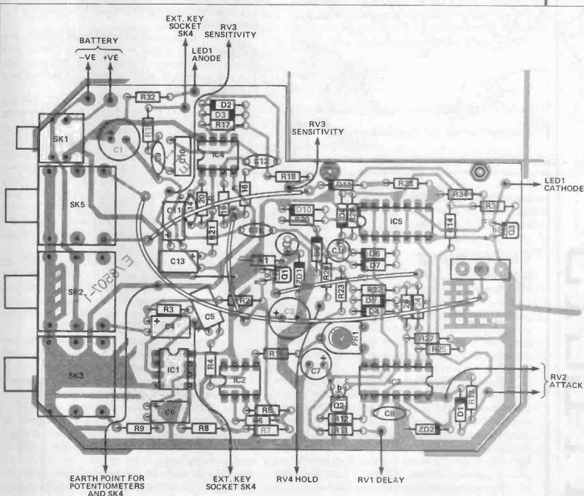
Fig. 3 The component overlay for the noise gate
