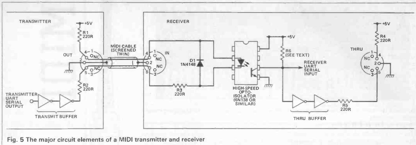
Fig. 5 The major circuit elements of a MIDI transmitter and receiver
