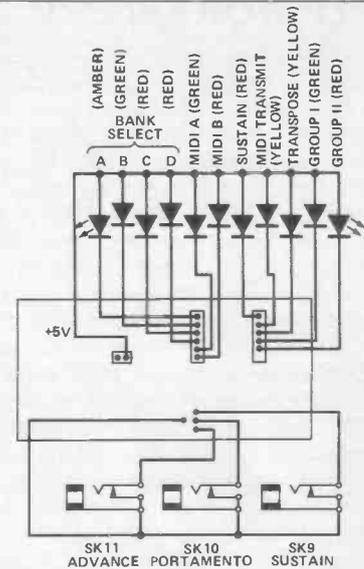
Fig. 13 Wiring the LED indicators and the footswitch sockets
