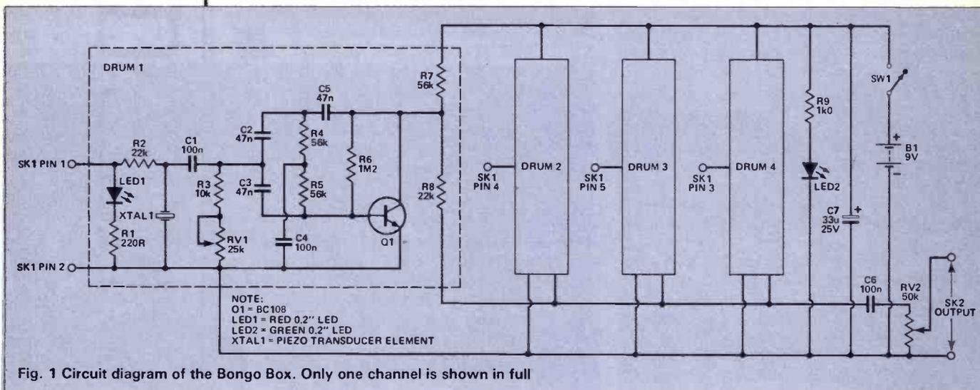
Fig. 1 Circuit diagram of the Bongo Box. Only one channel is shown in full
