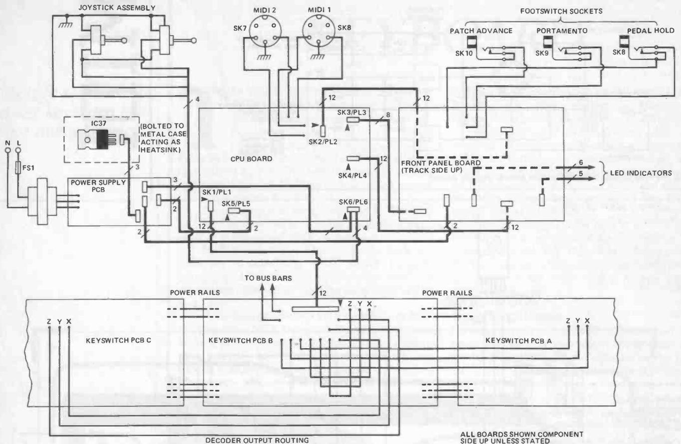
Fig. 17 The inter-board wiring for the whole MIDI Master Keyboard
