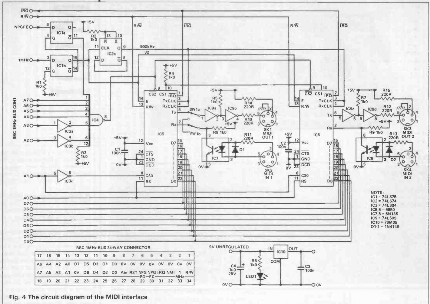
Fig. 4 The circuit diagram of the MIDI interface
