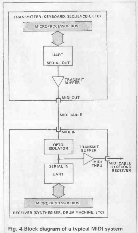
Fig. 4 Block diagram of a typical MIDI system
