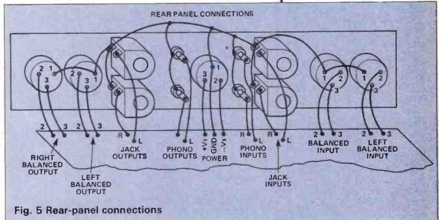
Fig. 5 Rear-panel connections
