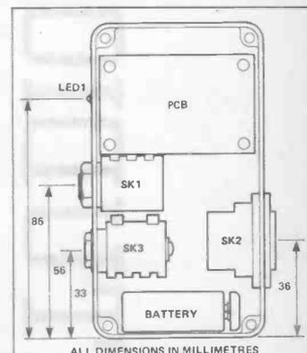
Fig. 4 Layout of the major components within the case
