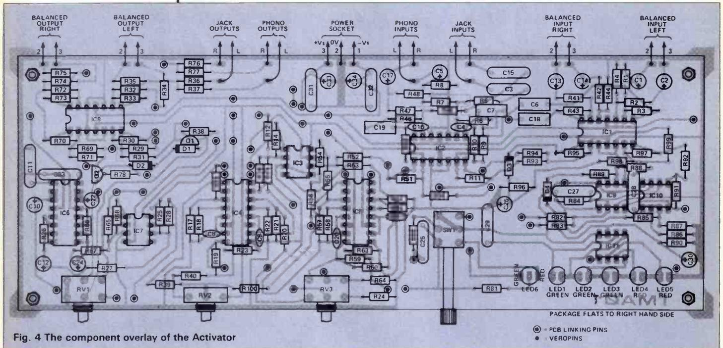
Fig. 4 The component overlay of the Activator
