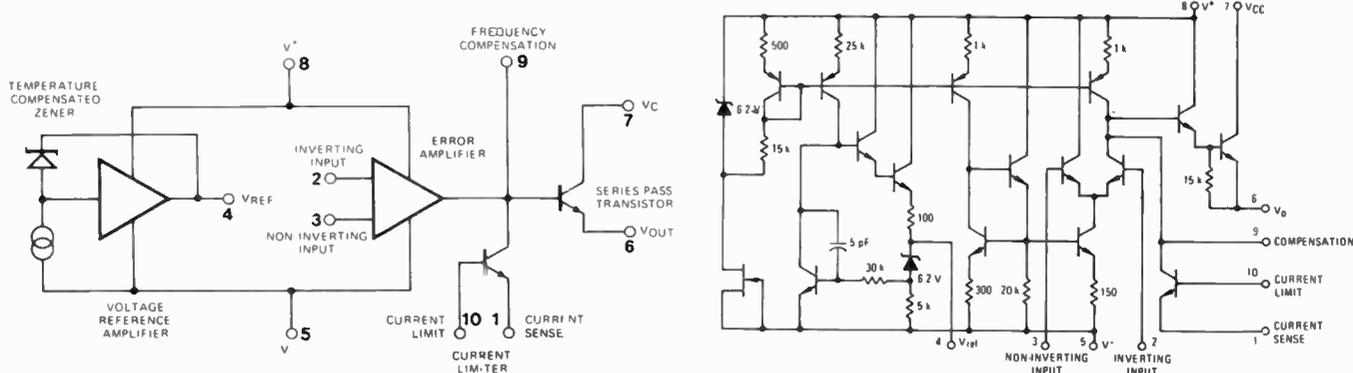
Fig. 2. Simplified schematic of  $\mu A723$ .
