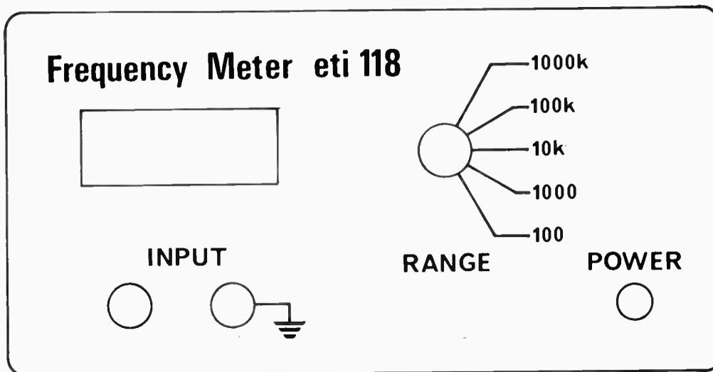
Fig. 5. Front panel of the frequency meter.
