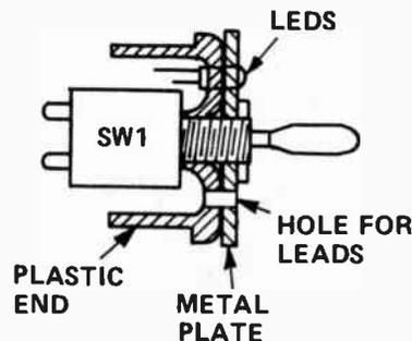
Fig. 6. How the probe ends are constructed.
