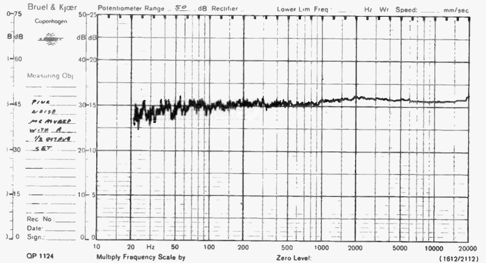
*Amplitude of pink noise versus frequency as measured with a one-third octave filter set.*
