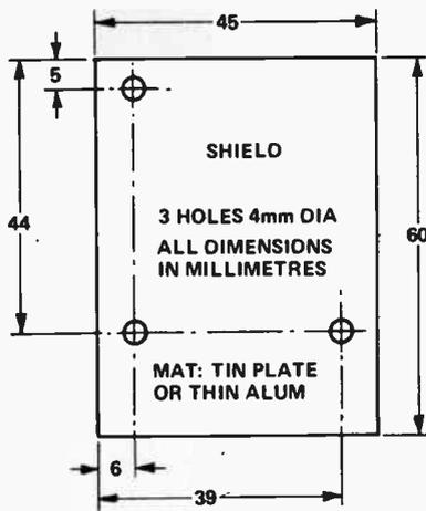
Fig. 7. Drilling details of the shield plate.
