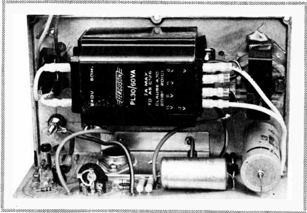
WHILST the introduction of CMOS has lowered the power requirements of digital equipment using it, many large scale systems, because of cost and availability, are still designed around TTL logic. For such systems a five-volt supply having a capability of up to 10 amps is often required.
