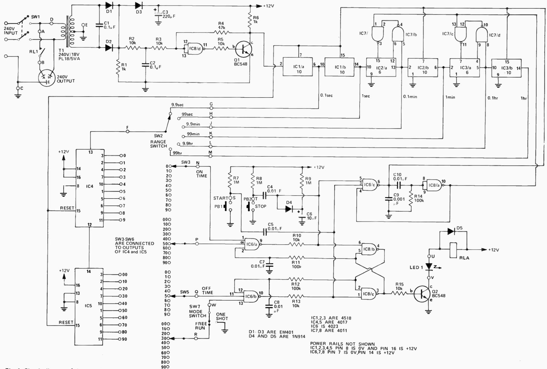
Fig. 1. Circuit diagram of the complete timer.
