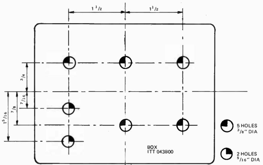
Fig. 4. Drilling details for the diecast box.
