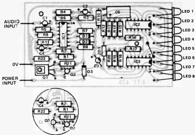
Fig. 2. Component overlay using BD140 for Q1. Circled diagram shows use of alternative BC640
