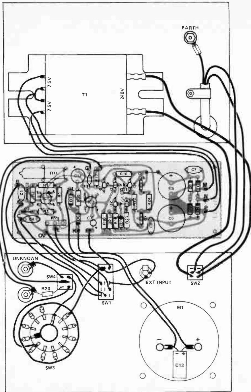
Fig. 4. Component overlay and wiring diagram for the impedance meter.
