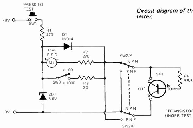
Circuit diagram of the ETI transistor tester.
