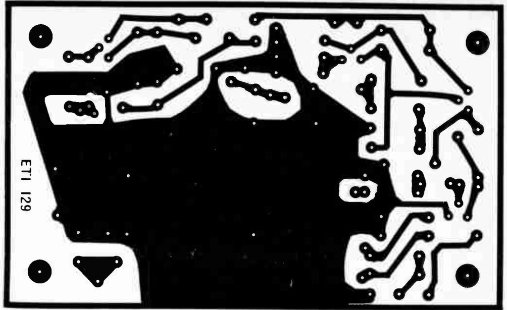
Printed-circuit board layout. Full size 129 x 80 mm.
