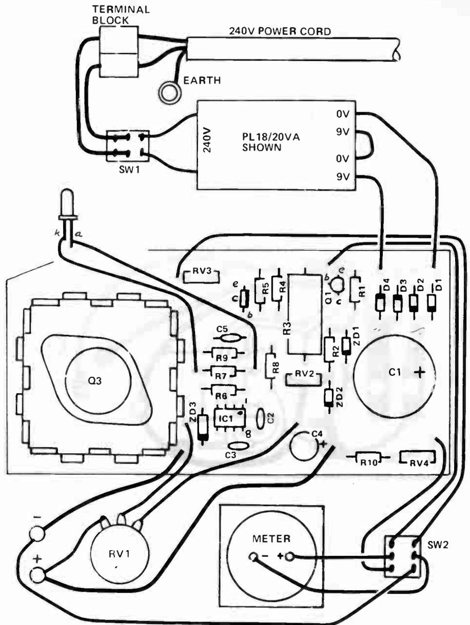
Fig 3. The component overlay and interconnection diagram.
