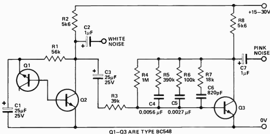
Fig. 1. Circuit diagram of the noise generator.
