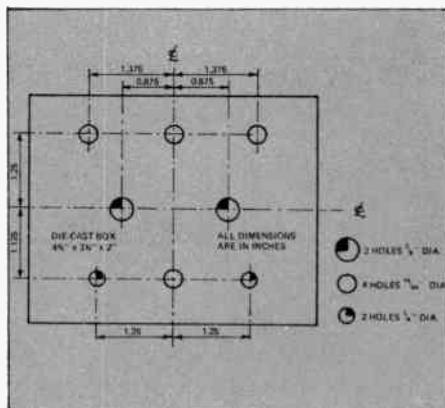
Fig. 2. Drilling details for the die cast box.
