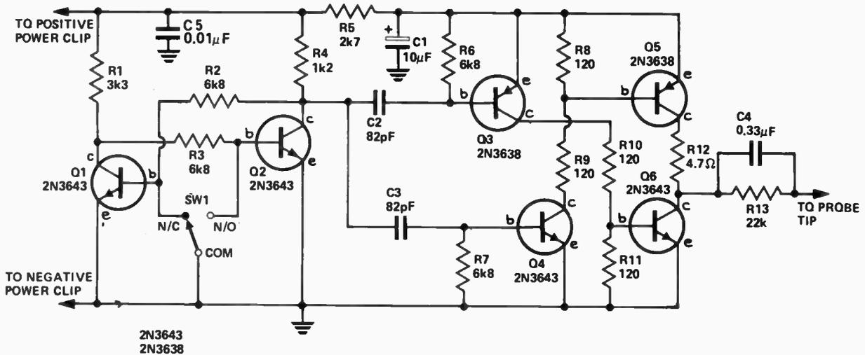
Fig. 1. Circuit diagram of the pulser.
