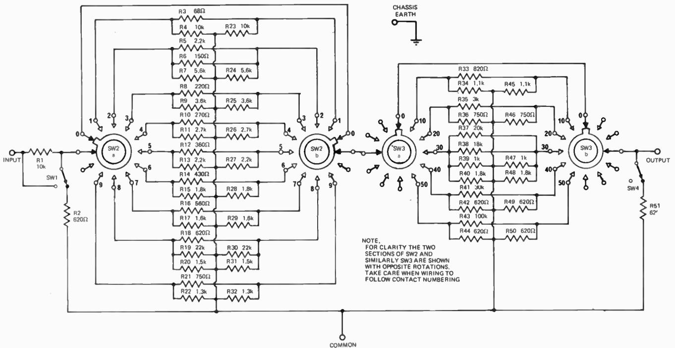
Fig. 1. Circuit diagram of the attenuator.
