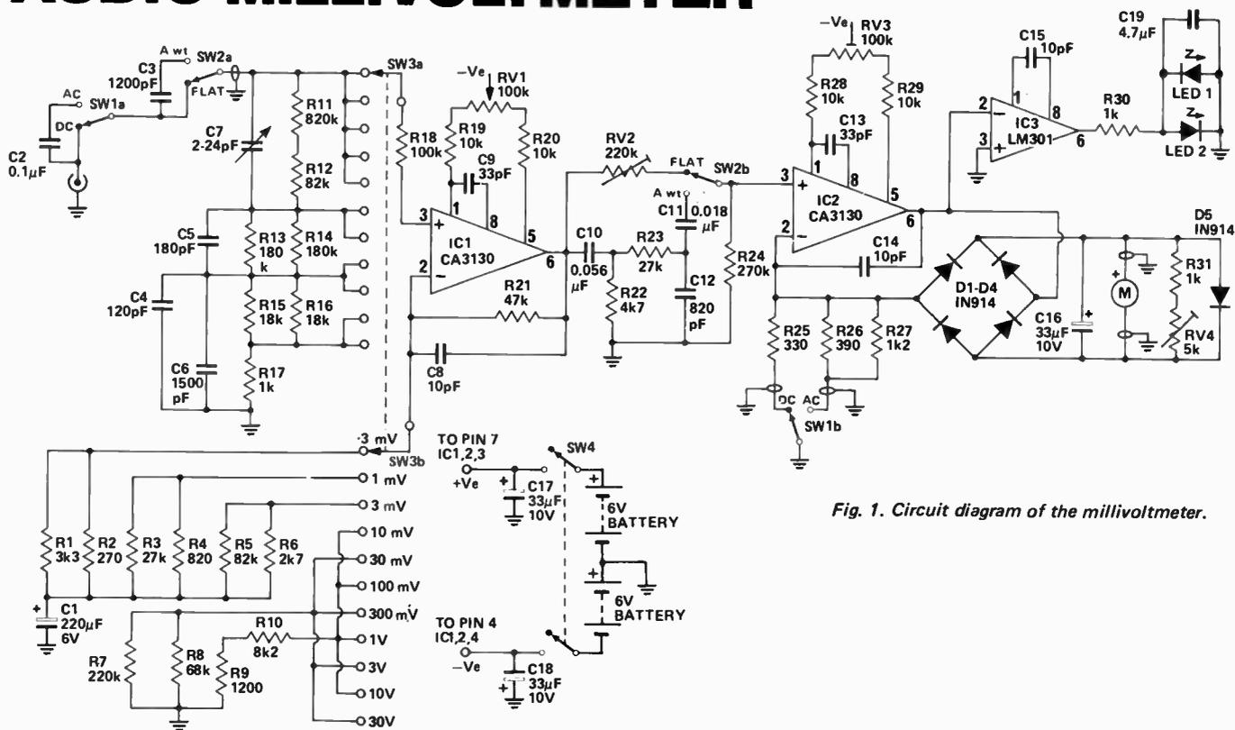
Fig. 1. Circuit diagram of the millivoltmeter.
