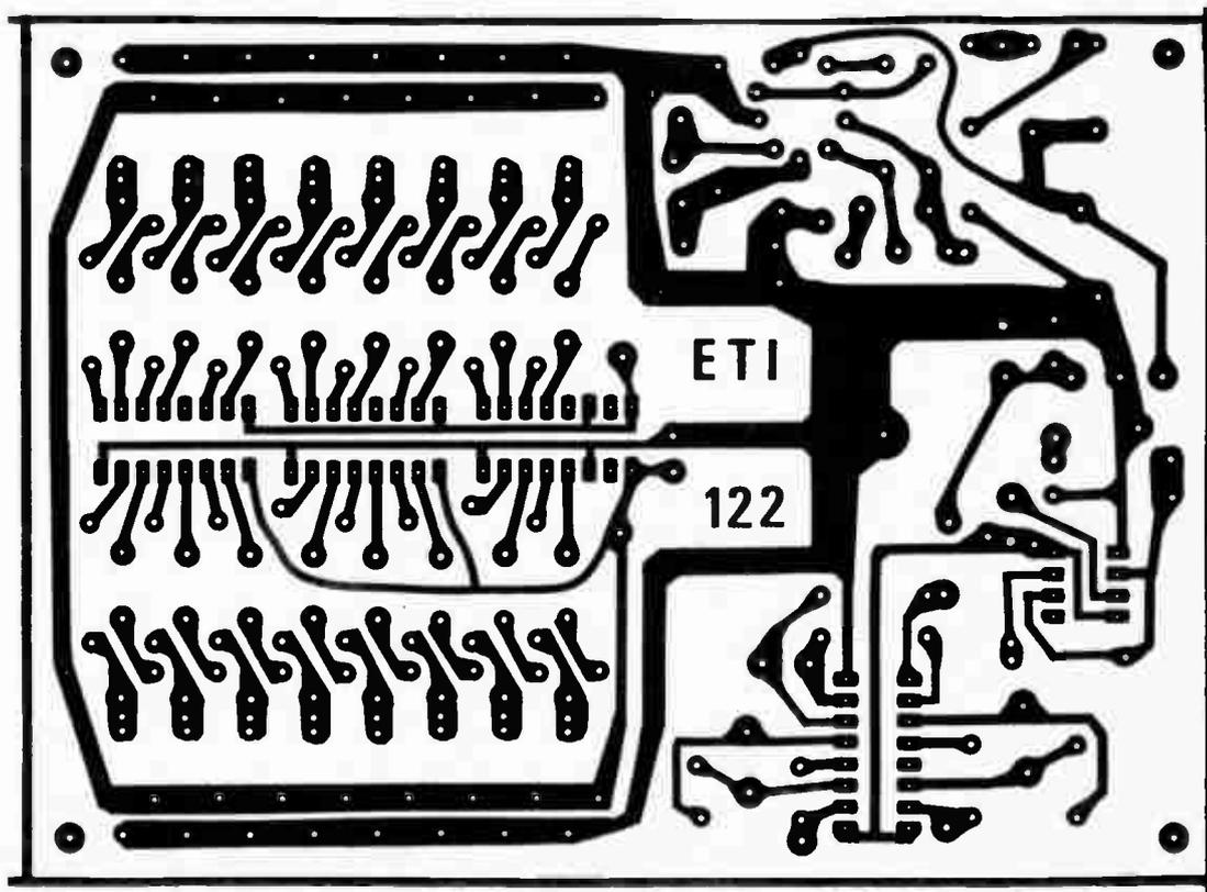
Fig. 7. Printed circuit-board artwork. Full size 142 x 104 mm.
