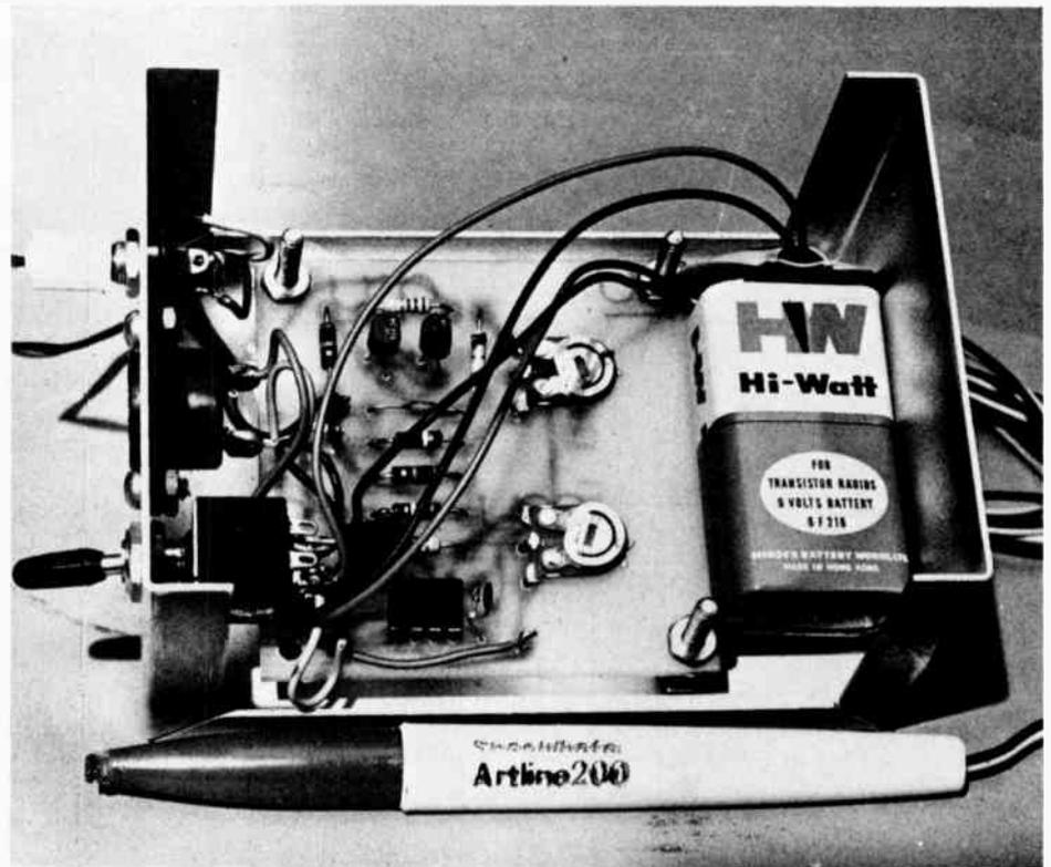
Internal view of the completed temperature converter. Note also the probe at front.
