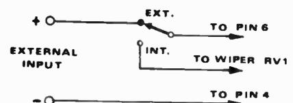
Fig. 2. Circuit modifications for externally programming positive rail (see text).
