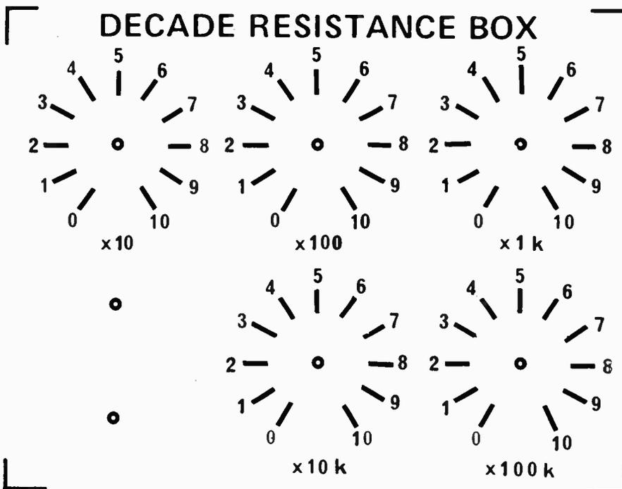
Fig. 3. Front panel overlay (full size).
