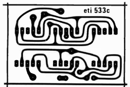
Fig. 5 Printed circuit layout of the d:display board. Full size 53mm x 36mm.
