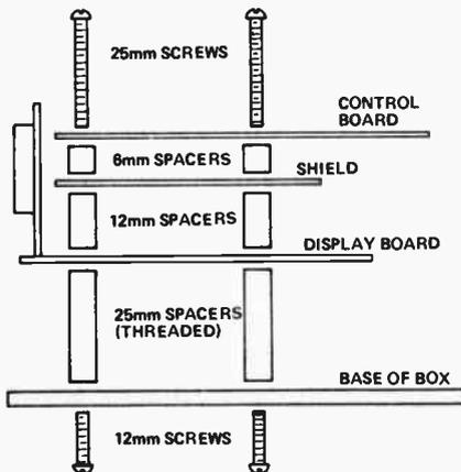
Fig. 8. Assembly of the counter display boards.
