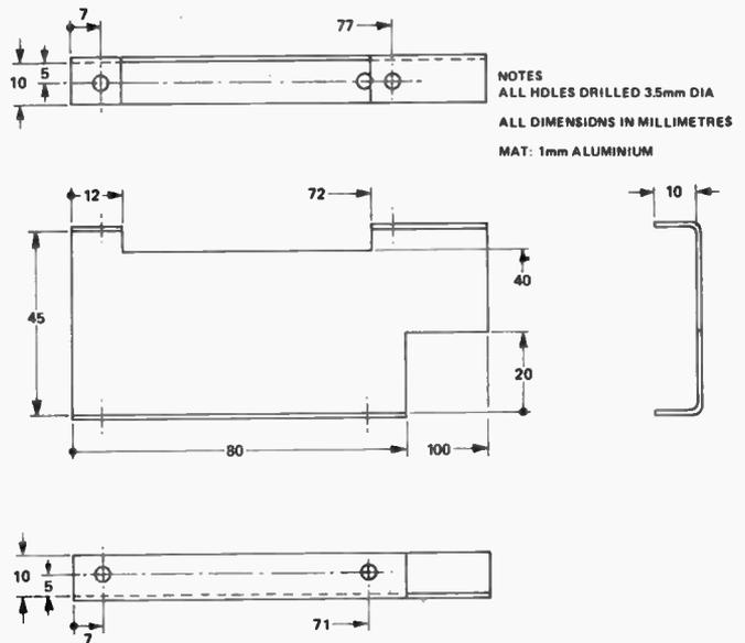
Fig. 7. Details of shield-support bracket.
