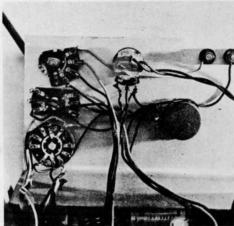
Simply constructed audio signal generator provides adequate performance for home and shop use.
