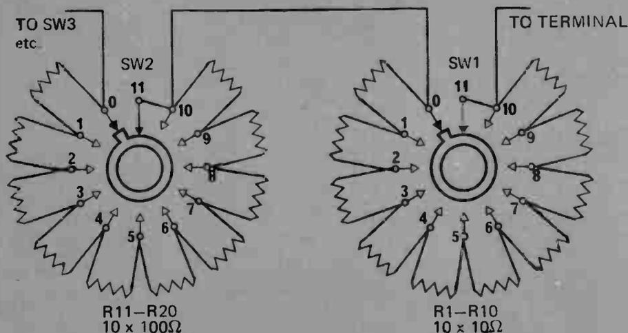
A DECADE resistance box is an extraordinarily useful device – enabling the user to select precisely the resistor value needed when that breadboard mock-up doesn't quite match the theoretical calculations: there being nothing more time consuming than the 'unsolder and try another' technique.
