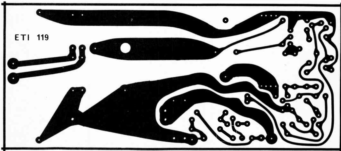
Fig. 5. Printed circuit-board layout. Full size. 178 x 78 mm.
