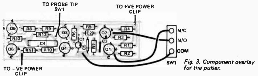
Fig. 3. Component overlay for the pulser.
