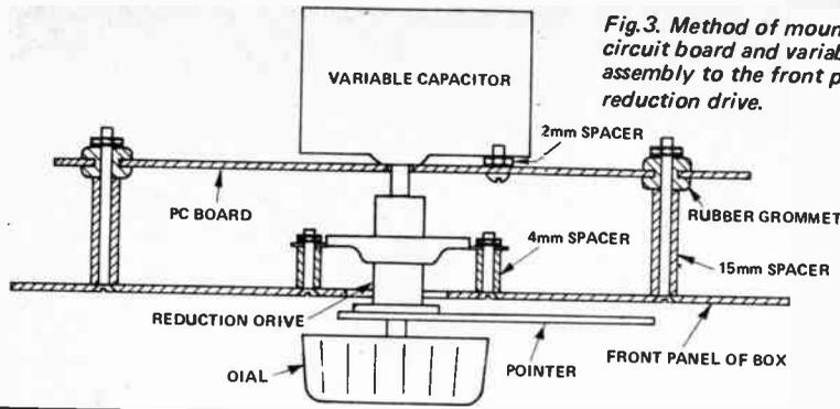
Fig. 3. Method of mounting printed-circuit board and variable capacitor assembly to the front panel and reduction drive.
