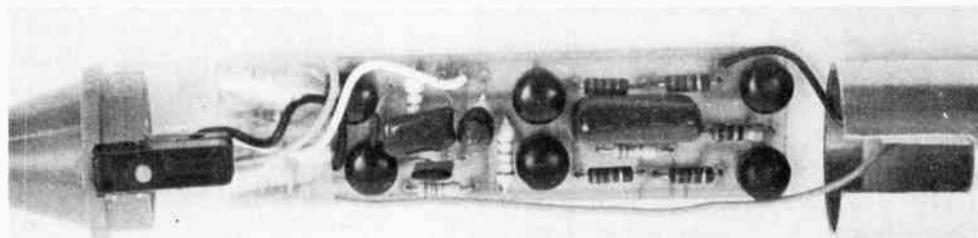
*Internal construction of the pulser.*
