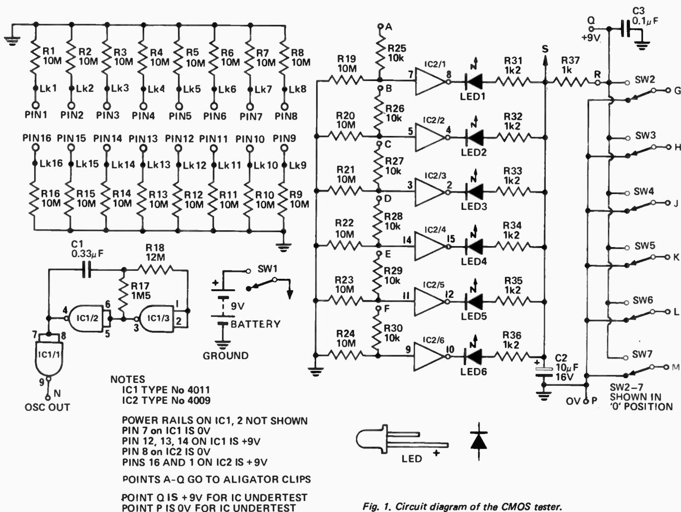
Fig. 1. Circuit diagram of the CMOS tester.
