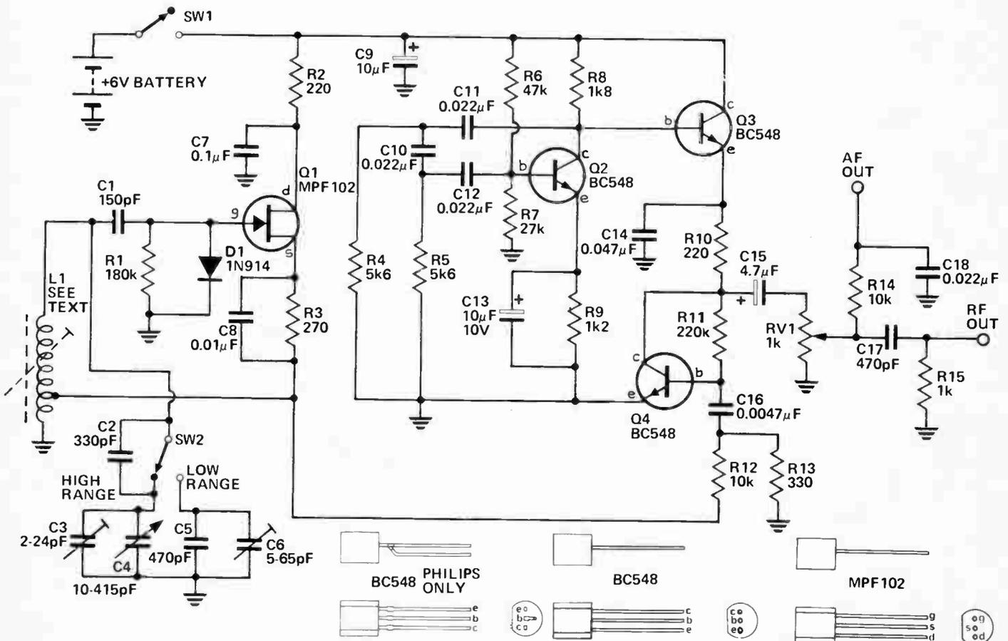
Fig. 1. Circuit diagram of the modulated RF generator.
