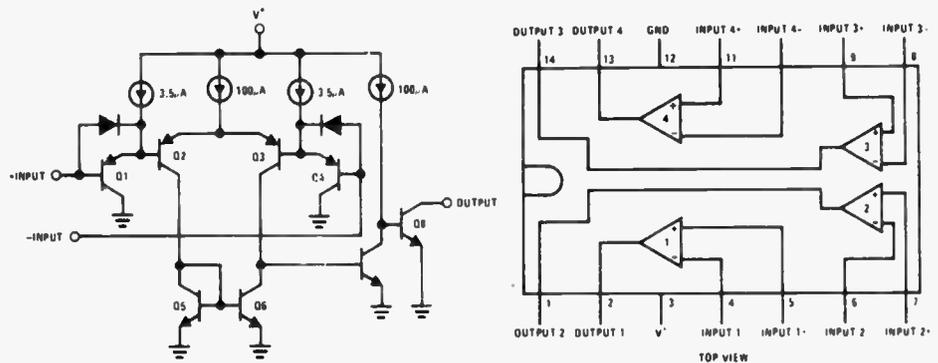
Fig. 3. Internal circuitry and pin connections of the LM339 IC.
