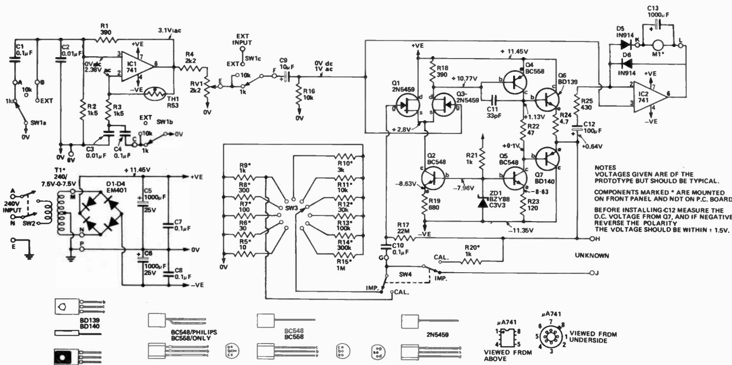
Fig. 2. Circuit diagram of the complete impedance meter.
