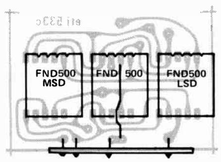
Fig. 3 Component overlay of the display board.
