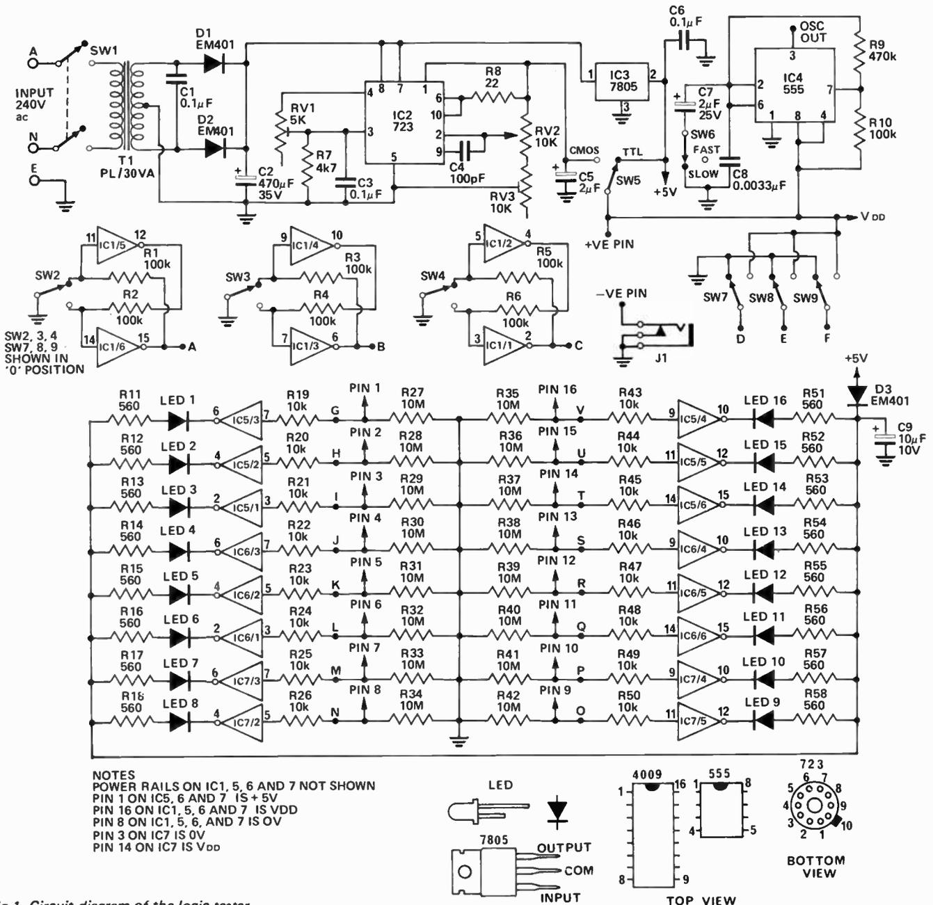
Fig. 1. Circuit diagram of the logic tester.
