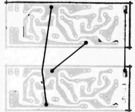
Fig. 4. Linking required between the two boards.
