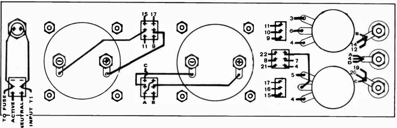
Now mount the transformer and the filter capacitors onto the chassis. Locate diodes D1 – D4 on top of the filter capacitors as shown in Fig. 5.
