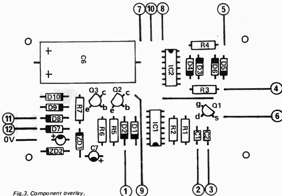
Fig.3. Component overlay.
