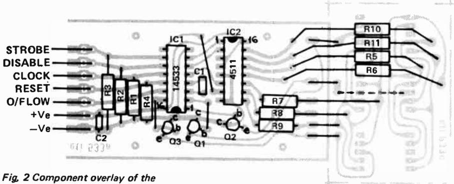
Fig. 2 Component overlay of the logic board.
