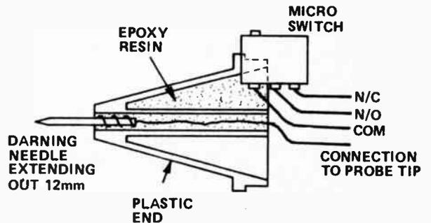
Fig. 4. Construction of the tip for the pulser probe.
