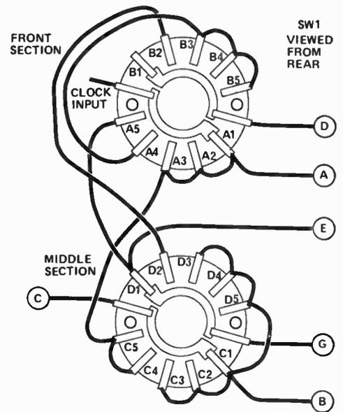
Fig. 3. Wiring of the range switch.
