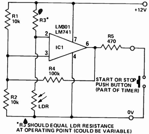
Fig. 6. For triggering timer from a change in light level this circuit will be found suitable.
