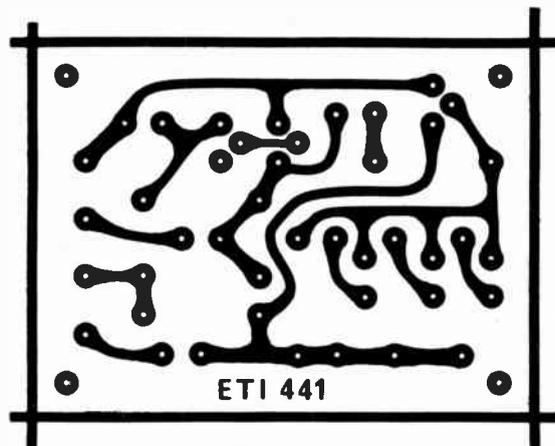
Printed circuit layout. Full size 67 x 49 mm.
