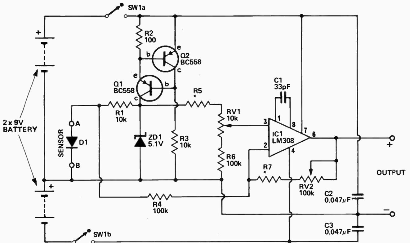
Fig. 1. Circuit diagram of the temperature meter.
