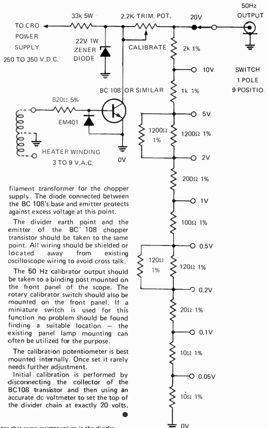
filament transformer for the chopper supply. The diode connected between the BC 108's base and emitter protects against excess voltage at this point.
