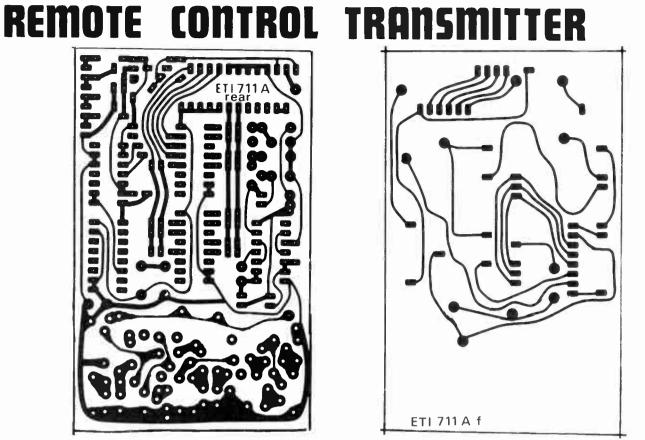
Fig. 8. Printed circuit layout for the rear side of the transmitter board, Full size 100 x 62mm
