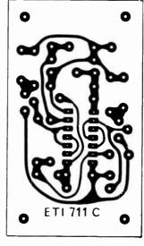
Fig. 6. Printed-circuit layout for the double-control relay driver.
