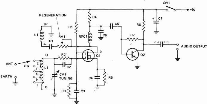
Fig. 1. Circuit diagram of the receiver.
