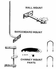
Commonly available TV antenna mounting components are inexpensive and provide a range of mounting options for the antenna described here.
