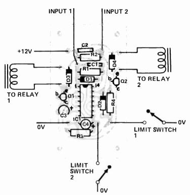
Fig. 4. Component overlay and interconnection diagram for the doublecontrol relay driver.
