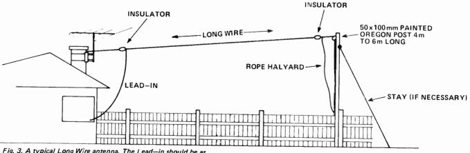
Fig. 3. A typical Long Wire antenna. The Lead-in should be as short as possible
