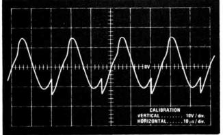
Fig. 3a. Waveform across the transducer on the the transmitter.
