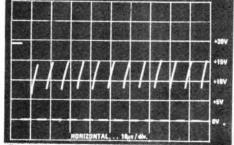
Fig. 4. An expanded view of the transformer drive waveform showing the collector voltage of Q1.
