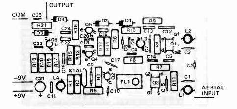
Fig. 4. Component overlay for the receiver.
