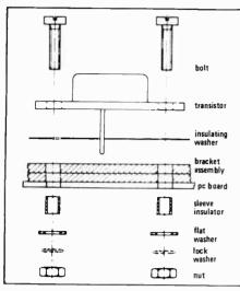
Exploded view of how the TO3 output transistors are assembled to the angle brackets and pc board.
