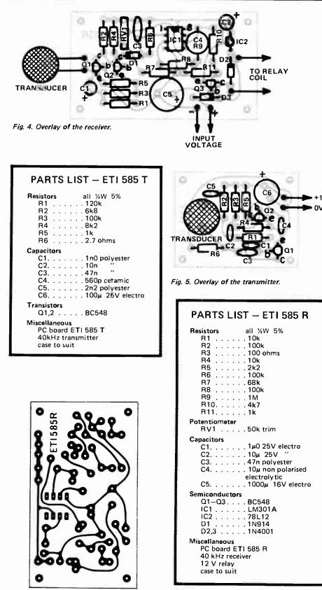
Fig. 6. Printed circuit b**oar**d of receiver. Full size 70 x 40.
