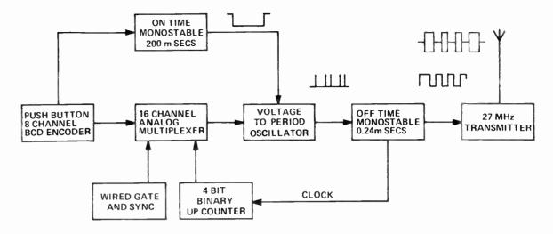
Fig. 3. Block diagram of the transmitter showing basic operation of unit.
