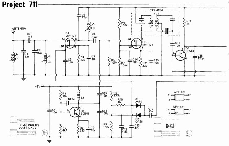
Fig. 3. Circuit diagram of the receiver.
