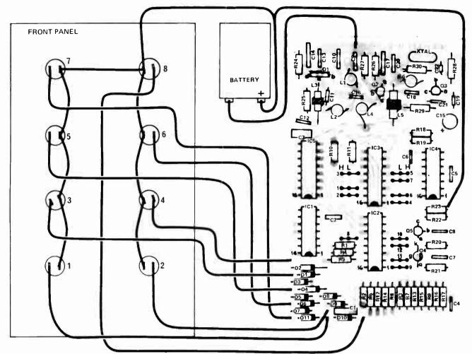
Fig. 7. Component overlay and wiring diagram. Note the links from IC2 and IC3 to the 'H' or 'L' lines. You must decide on the code word to be used and link to one or the other as detailed in the text. Overlay is shown larger than full size for clarity.
