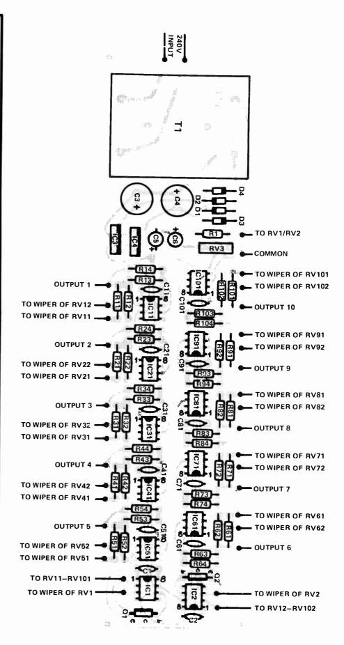
Fig. 2. Component overlay for the controller board, ET1588C. Printed circuit board pattern is on page 159.
