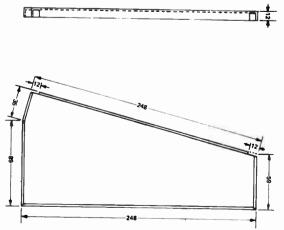
Fig. 4. The end pieces for the box. These should be fitted into the ends of the box as shown in Fig. 3. The two ends should be of opposite hends.
