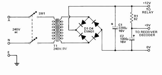
Fig. 3. Circuit diagram of the power supply for the complete receiver decoder. ETI 711P
