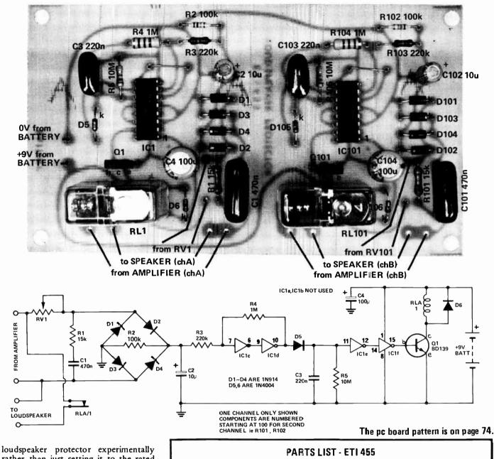
rather than just setting it to the rated power handling of your loudspeakers. Your ears are the best indication that the system is being strained. Set the loudspeaker protector so that it trips just below that volume where distortion starts to occur.
