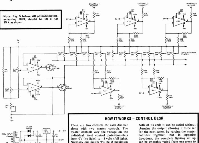
Fig. 5. The circuit diagram of the control desk.
