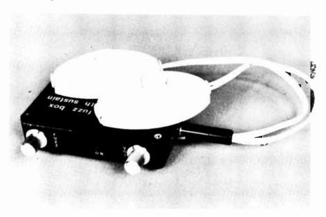
with a fixed compression ratio of 2:1. This compression effectively halves the dynamic range of the incoming signal by attenuating high level signals and boosting low level ones; thus the signal hangs on – "sustains" – for much longer than it otherwise would. The compression also provides a constant
