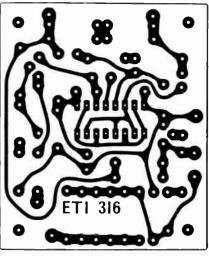
Fig. 3. Printed circuit board. Full size 65 x 55 mm.
