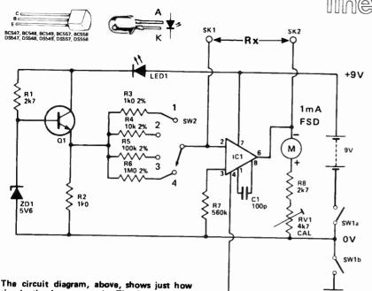
simple the instrument is. The internal view simple the instrument is. The internal view at left illustrates placement of the major components. We secured the pc board with a strip of double-sided tape, available in hardware stores.
