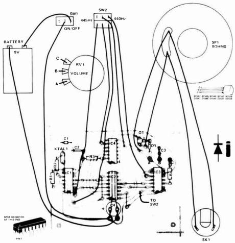
Component overlay. The pc board pattern is reproduced on page 158.
