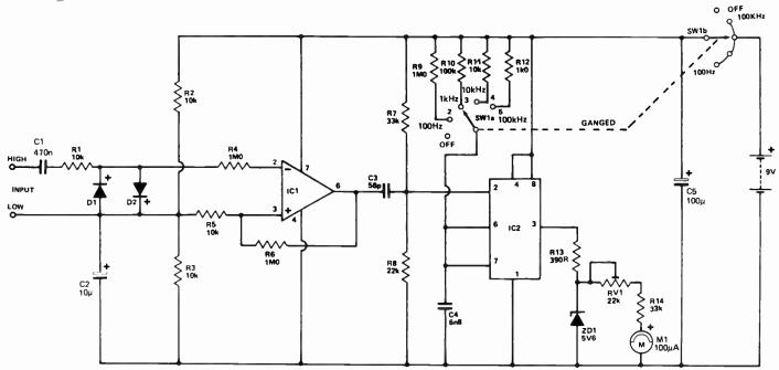
microamp movement for convenience as it does not have to be re-scaled. The lowest range is 100 Hz full-scale deflection, the highest, 100 kHz.
