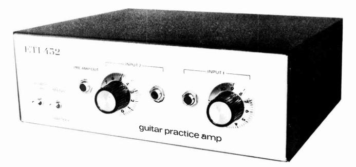
THIS PROJECT has been designed to enable guitarists to put in long hours of practice and still keep that high power amp in the cupboard, where it belongs! It is a compact amp capable of about 7W into a 4 ohm load. This is enough power for practice purposes and just think of the greatly improved relations you will have with your neighbours.
