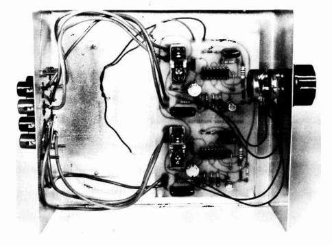
Internal view of the speaker protector. We mounted the unit in a 'Deluxe Metal Cabinet'' from Dick Smith measuring 184 x 160 x 70 mm, but you can choose any similar size cabinet to suit your equipment or even mount single units in your loudspeaker enclosures with preset controls.
