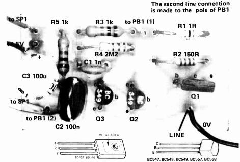
Overlay for the pc board. Take care with the orientation of the capacitor C3 and the transistors.
