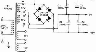
Complete circuit diagram of the amplifier. Note that L1, not listed in the parts list below, is wound on a 1 W resistor – see text. Voltage readings are included as a guide.
