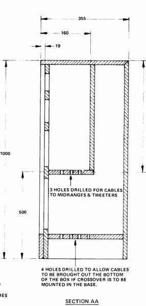
Complete cutting and assembly details for the four-way loudspeaker box. It is important that all joints be well sealed.
