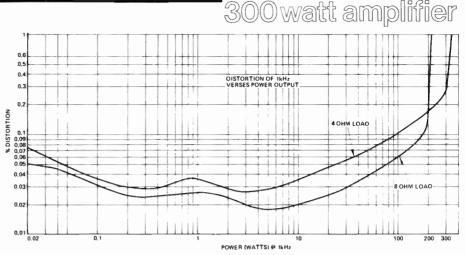
Total harmonic distortion versus power output at 1 kHz. The 'bump' at around 1 W is due to the output stage changing from Class A operation to Class AB operation.
