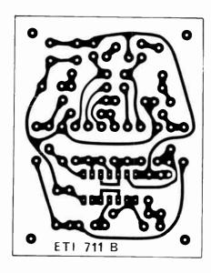
Fig. 7. Printed circuit layout for the single-control relay driver.
