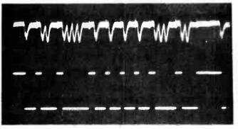
1a input to decoder b output of IC1
