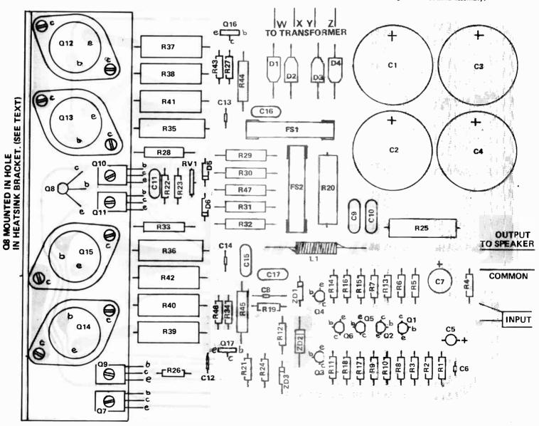
The complete amplifier, including the power supply components and output transistors, is assembled on a single pc board. An aluminium bracket holds the output transistors conducting heat from the output stage to the heatsink. Only three sets of external connections are made to the pc board; input, output and power supply ac input from the transformer.
