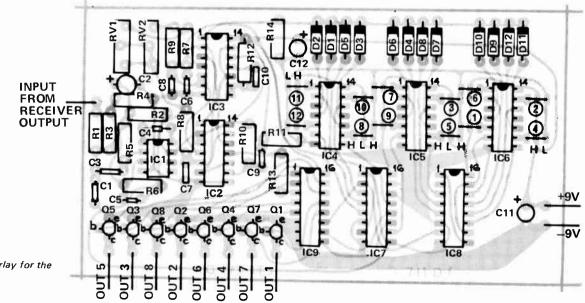
Fig. 7. Component overlay for the decoder.
