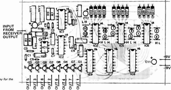
Fig. 7. Component overlay for the decoder.
