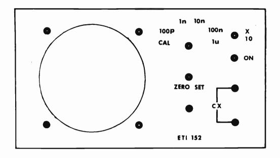
the x10 range resistor, are mounted on the front panel. Mount the smaller switches and terminals first, followed by the potentiometers and last of all the meter. The resistor R14 is wired from the positive meter terminal to one of the contacts on the range switch, SW3.
