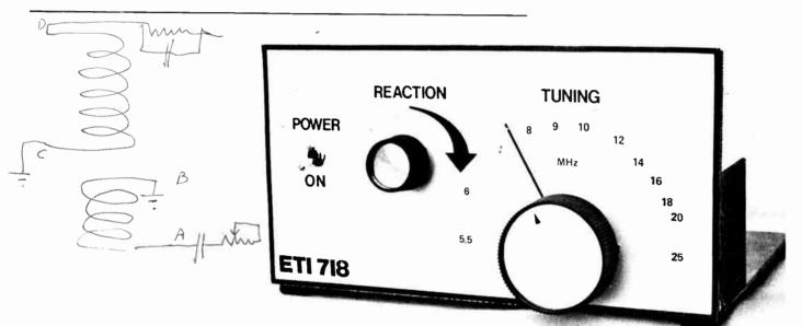
APART FROM THE very early sets, which were based upon coherers and other devices you never hear of today, the first radios were very straightforward designs totally unlike today's sophisticated superhets. The early Tuned Radio Frequency (TRF) sets were simply a tuning circuit with some gain and a detector circuit, but later designs used positive feedback, in the form of reaction, to increase the performance. It is still possible to get a lot of fun from sets of this type.
