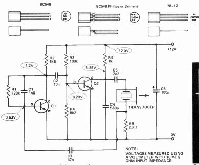
Fig. 2. Circuit diagram of the transmitter.
