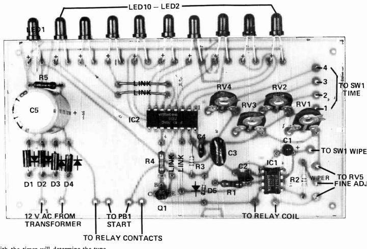
with the timer will determine the type of relay you use. This unit is capable of driving quite large relays, however, we used a commonly available Omron type having contacts rated at 10 amps.
