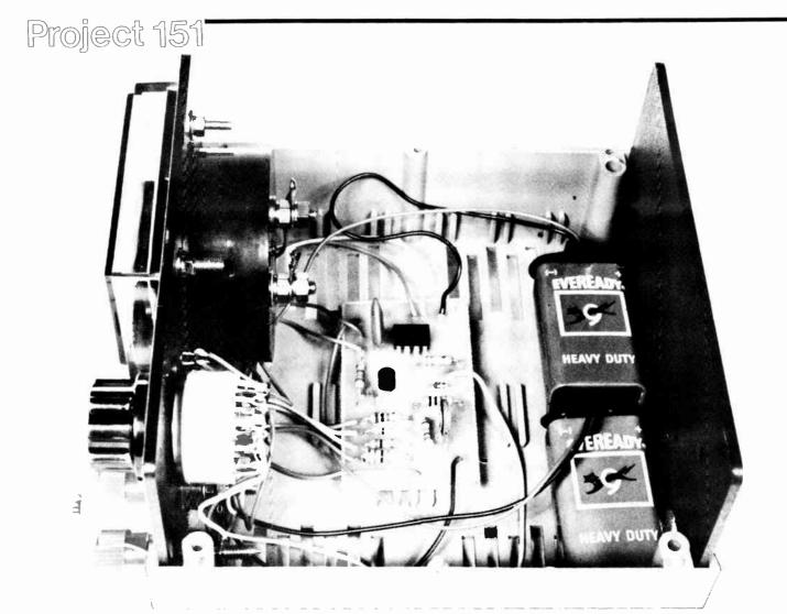
741 as it has been selected for its low input current. The overall accuracy of the instrument is determined by the tolerance of the range resistors (R3 to R6) and the accuracy of the meter. If 1% or 2% resistors are used the accuracy of the instrument will be about two percent. See Shoparound for a list of suppliers with close tolerance resistors.
