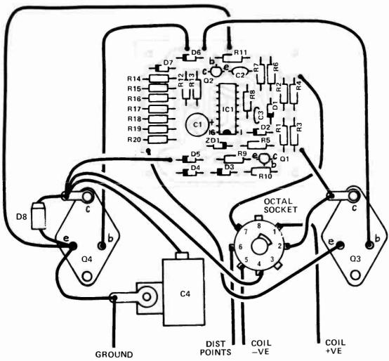
Fig. 2. Overlay and wiring diagram.
