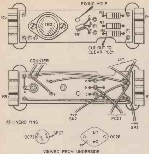
Fig. 2. The layout of the components on both sides of the Paxolin board. Veropins are used for attachment.
