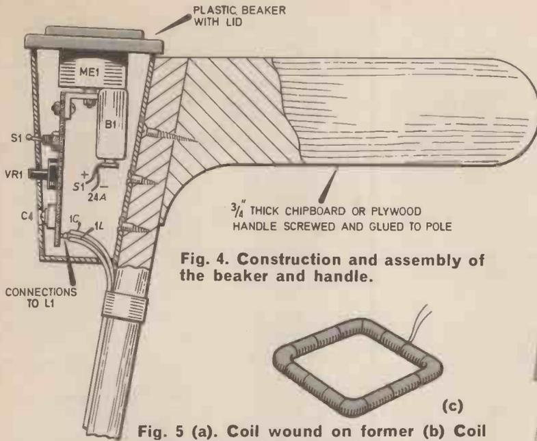
Fig. 4. Construction and assembly of the beaker and handle.
