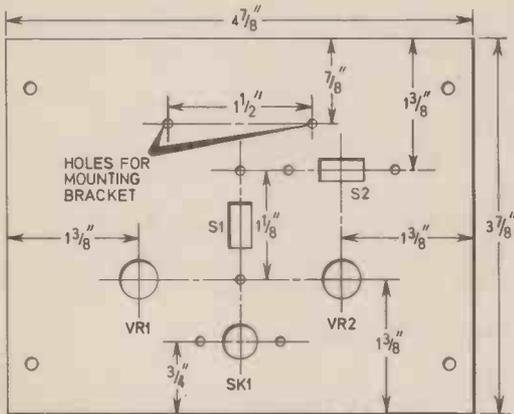
Fig. 5. Front panel drilling details.
