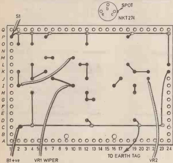
Fig. 6. Top and underside views of the component board. The transistor connections between the two diagrams are viewed from the underside.
