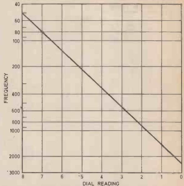
Fig. 8. Approximate output frequency for various control settings.
