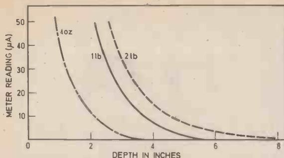
Fig. 2. Response curves of the Metal Locator.
