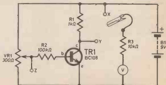
VR1 is a 300 ohm potentiometer working as a potential divider giving us a variable supply at its wiper.
