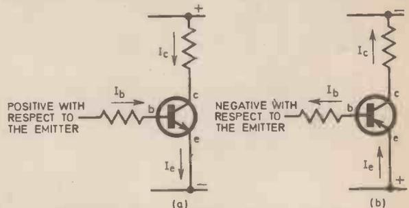
**Fig. 5. Circuits showing major current flow directions for (a) *nnp* and (b) *pnnp* transistor.  $I_b$ —base current,  $I_c$ —collector current,  $I_e$ —emitter current.**
