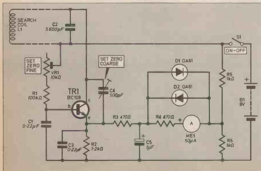
Fig. 1. Circuit diagram of the Metal Locator. The search coil L1 is mounted in the locator head and the dotted lines are the connecting wires to the circuitry.
