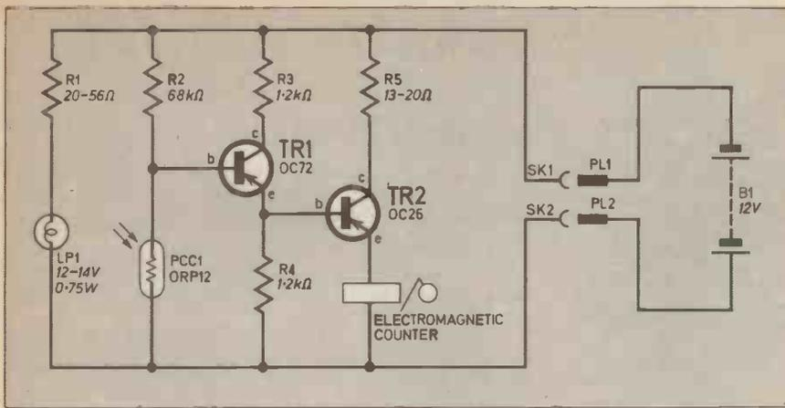
Fig. 1. The complete circuit diagram of the Bee Counter.
