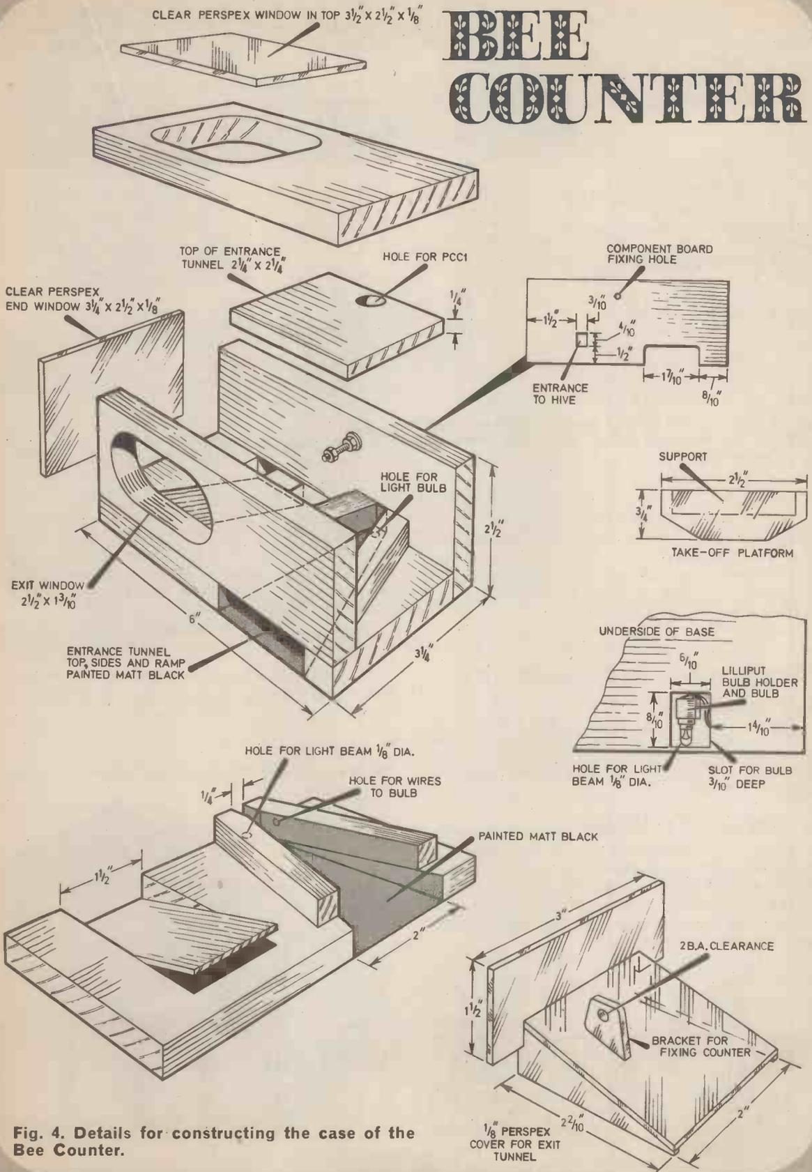
Fig. 4. Details for constructing the case of the Bee Counter.
