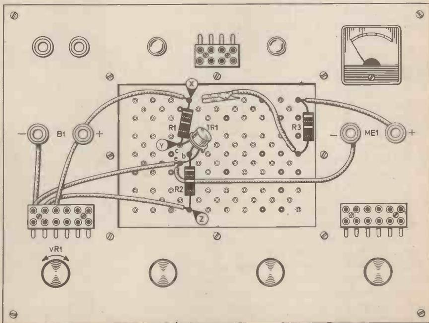
and any internal resistance between base and emitter. The latter is small and can be neglected at this stage. We must, remember, however, that the base must be made at least 600mV positive with respect to the emitter before any current can flow (this is the usual forward voltage drop for any silicon junction).
