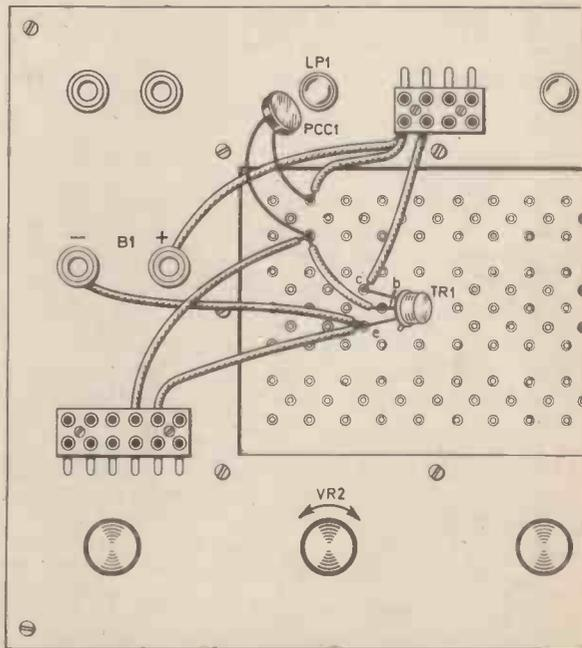
Break the light path between the bulb and the cell and the bulb goes out and stays out. Now use a match or lighter to provide a stimulus of light. Bring it close to the bulb/cell assembly and the bulb lights up; you can now remove the match and the bulb will stay on because its own light output is holding the transistor on. This is called "positive feedback" and in this circuit will provide an amusing party trick—especially if assembled to look like a candle.
