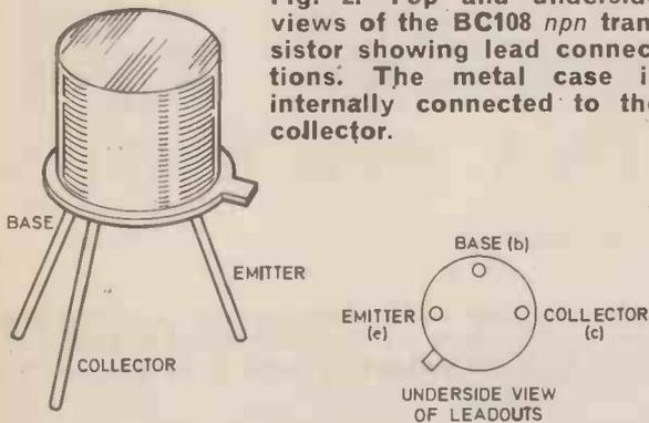
Fig. 2. Top and underside views of the BC108 *npn* transistor showing lead connections. The metal case is internally connected to the collector.
