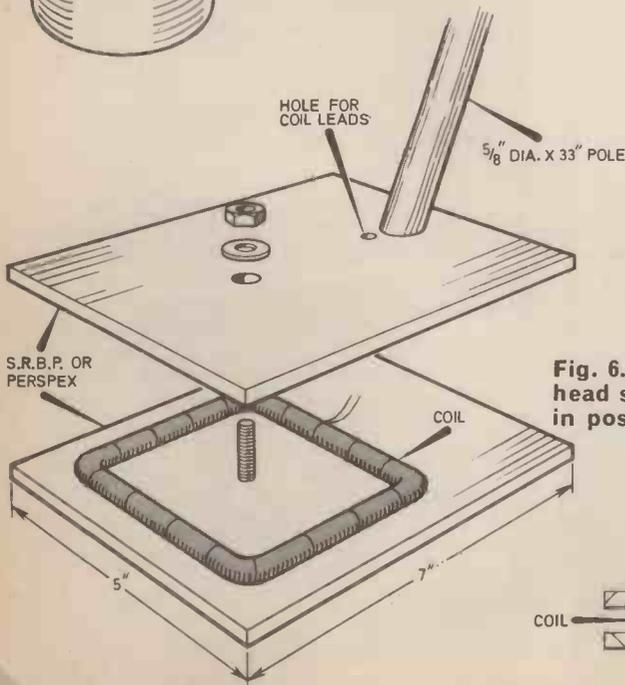
Fig. 6. Construction of the locator head showing how the coil is held in position.
