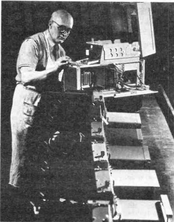
Final check-out of a Marconi v.h.f. TV transmitter.
