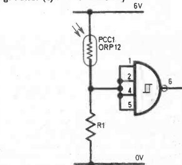
Fig. 7.10. The light operated switch described in an earlier part may be used to drive the Schmitt
