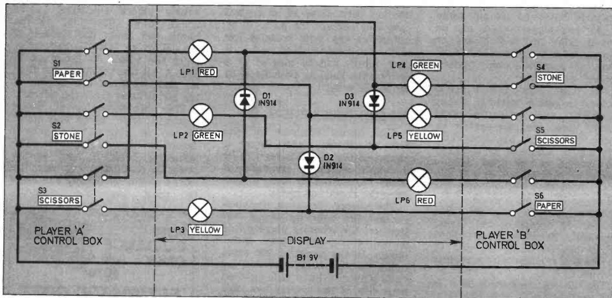
Fig. 1. The circuit diagram of the Scissors-Stone-Paper Game.
