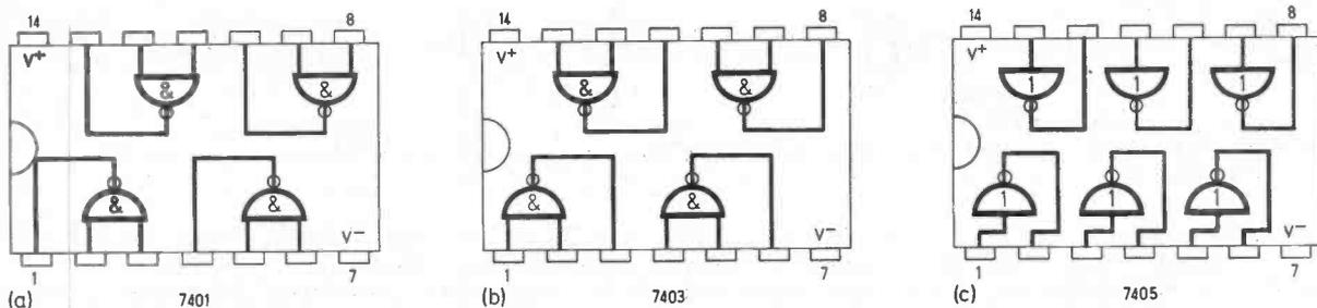
Fig. 7.4. Pin connections for three types of open collector i.c.s. (a) the 7401 quad two-input NAND gate (b) the 7403 quad two-input NAND gate and (c) the 7405 hex INVERTER.
