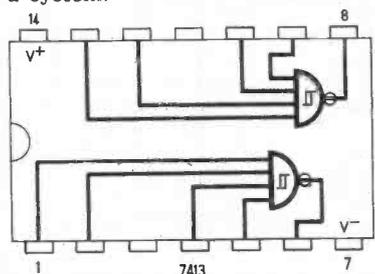
Fig. 7.6. Pin connections of the 7413 four-input Schmitt NAND.
