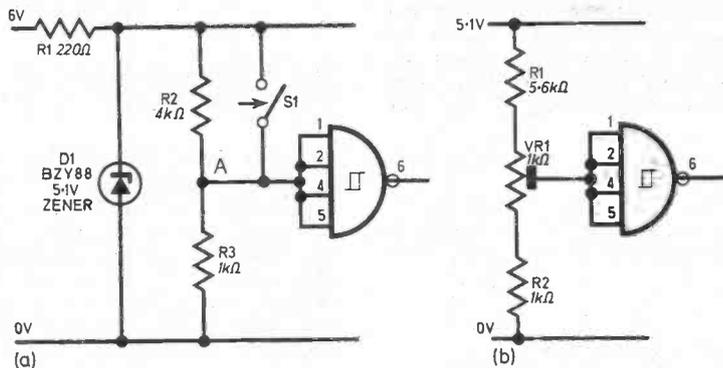
Fig. 7.11.(a) Circuit for a low battery indicator. The potential divider can be made from a preset and two resistors for setting the switching point, as at (b).
