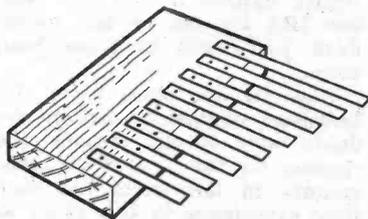
Fig. 2. The construction of a Kaffir Piano.
