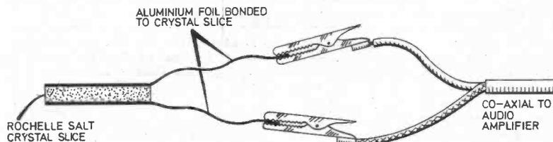
Fig. 1. The crystal pick-up constructed by Bob.
