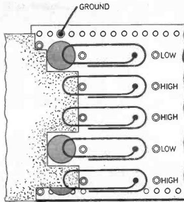
As with the keyboard, join the drawing pins together and to a terminal pin at the side. If the keyboard is on the same piece of board as the card reader, make sure the cuts in the copper strips are made as shown.
