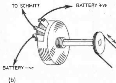
Fig. 7.9.(a) The input to the Schmitt can be from a potentiometer connected across a 6V battery. The potentiometer can be part of a working model as shown in (b).
