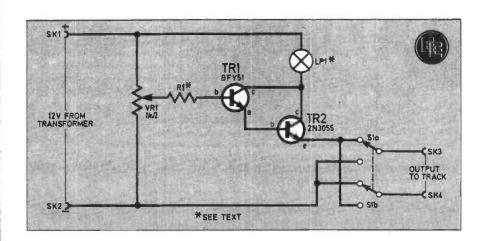
Fig. 2. The complete circuit diagram of the Train Controller.
