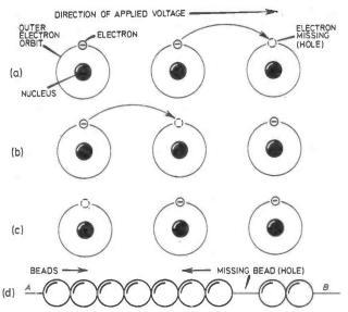
Fig. 1.3. Steps (a) (b) and (c) show that the effect of electrons hopping from atom to the next is equivalent to a hole (missing electron) moving in the opposite direction. This can be demonstrated by moving beads along a wire one at a time from A to B. The "hole" moves from B to A.
