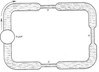
Fig. 1.4. The flow of current in a circuit can be likened to water being pumped through pipes. The battery can be thought of as a pump, and the resistors narrow sections along the pipe.
