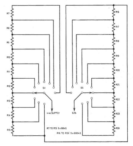
Fig. 2. The range switching circuitry for the Enlarger Timer.
