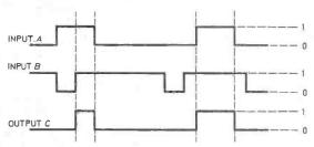
Fig. 3. The output is high only when both inputs are high.
