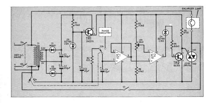
Fig. 1. Complete circuit diagram of the Enlarger Timer. The range circuitry is shown in more detail in Fig. 2.
