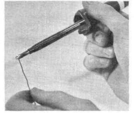
Tinning the bit of a soldering iron.
