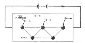
Fig. 1.2. Electron current flow in a metal. It is the electrons that become detached from their atoms and move under the influence of an applied voltage (the battery) that form this current. Note that "conventional" current flow I, is in the opposite direction.
