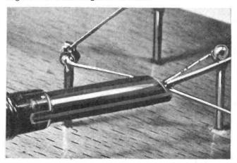
Soldering a piece of wire to a nail. Note carefully how the iron and solder are applied.
