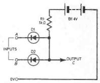
Fig. 2. Experimental AND gate.
