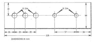
Fig. 5. Dimensions and drilling details for the front panel.
