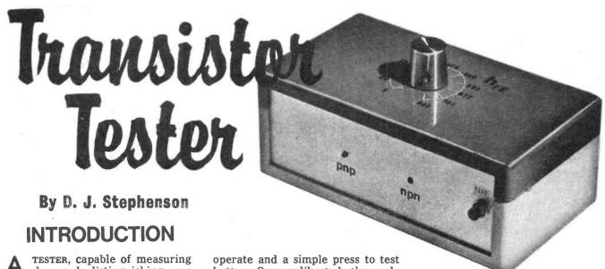
hfe and distinguishing pnp from npn transistors, will always remain a useful item in the work-
