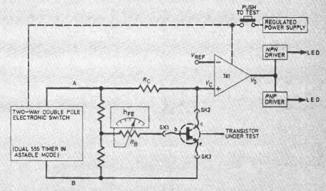
Fig. 3. Functional diagram to illustrate the working of the Transistor Tester.
