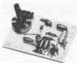
**KS100 MINIATURE V.H.F./A.M./F.M. RECEIVER.** Varicap tuned, 88-108 MHz earphone output 240mV, sensitivity 1uV, operates from 9V D.C. (PP3) 2.5mA semiconductors EET/E300 & BC205-G. £5.31 inc VAT
