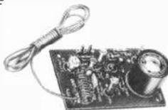
**KS200 MINIATURE F.M. TRANSMITTER.** 88-108MHz complete with dynamic microphone, operates from 9V D.C. (PP3), semiconductors 2N708 & BC208-8. Not Licenceable in U.K. £7.37 inc VAT
