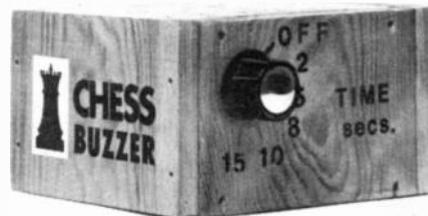
Finished unit with suggested lettering around timing switch S1.
