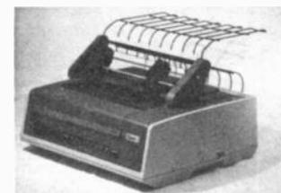
This machine incorporates an 18-needle printhead giving a print matrix of up to 18 × 25 dots per character on a single pass. With such high resolution it is not only possible to print characters practically as good as "fully formed" ones, as with a daisy wheel printer, but by using a semi-graphics font it is claimed to be possible to print forms, bar-codes, logos and so on.
