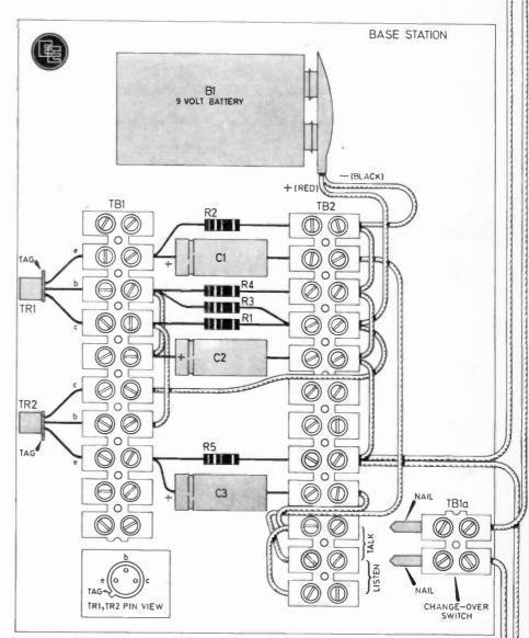
Fig. 1. Actual size layout and interconnection diagram of the Two Way Intercom. This may be used as a template.
