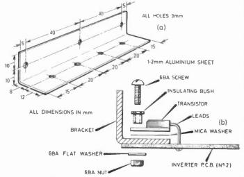
Fig. 3.3. Mounting bracket for inverter p.c.b. (a) constructional details (b) cross section showing method of mounting the Darlington transistors which also provides the means for securing bracket to board.
