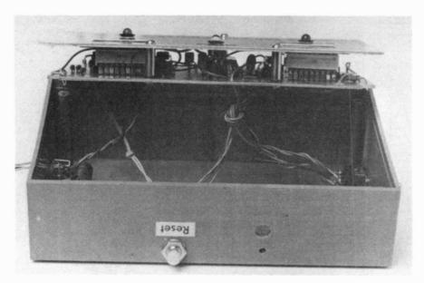
View inside the console showing the p.c.b. mounted beneath the lid.
