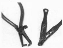
Fig. 2. Wire strippers. The pair on the left are of superior quality but as such, can be considerably more expensive. Both types are adjustable for different size wires.
