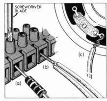
Fig. 3. Fixing component lead and two wire links to one block position (a) and (b); (c) shows wire connection to speaker eyelet.
