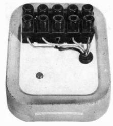
The terminal block is mounted onto the base of the "lozenge" tin as shown.
