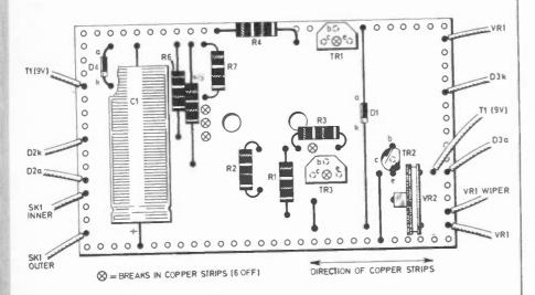
Fig. 2. Stripboard layout for the Comparator Voltmeter. Note the positions of the six track breaks.
