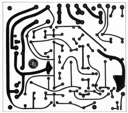
Fig. 3.4. Public Address System: Power Amplifier printed circuit board No. 1 (Main Board), actual size. NOTE: One side of C13 goes to terminal pin 14 (0V line), not to 12 (-42.5V line) as shown on circuit diagram.
