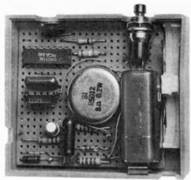
Full size prototype of the Pitch Pipe.
