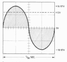
Fig. 1.1b. C.R.O. display for the 12 volts a.c.
