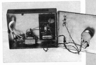
View inside the finished prototype unit. Note that the mains cable "p" clip is not shown, however it is important that it is included.
