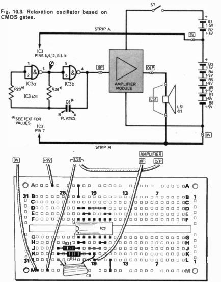
Fig. 10.4. The circuit of Fig. 10.3 wired up on the Verobloc.
