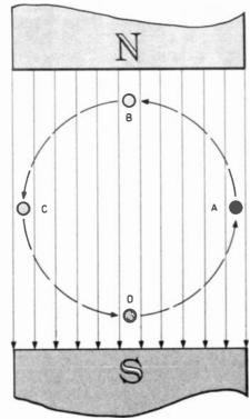
Fig. 1.2. Simple a.c. alternator. Magnetic field shown as parallel lines.
