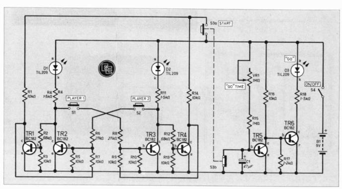
keeps TR6 on and D3 alight. As C1 slowly charges up via VRI and R15, the voltage at TR5 base gradually rises. When it reaches approximately 0.6V TR5 switches on. TR5 collector goes low, TR6 goes off and D3 is extinguished. The time it takes for this process to be executed can be varied by VR1.
