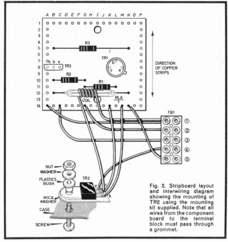
Most of the circuit is built on a piece of 0·lin pitch stripboard, 16 strips by 13 holes as shown in Fig. 2, with the exception of TR2 and the terminal block.
