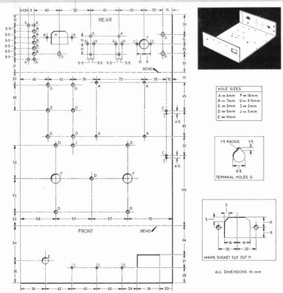
Fig. 3.1. Public Address System: Power Amplifier chassis drilling and bending details.
