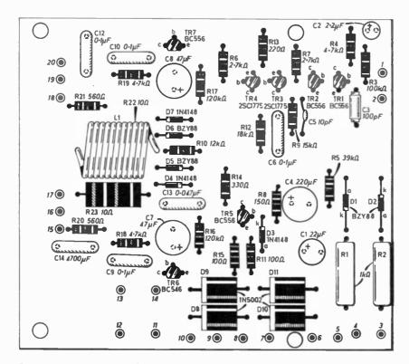
Fig. 3.5. Public Address System: Power Amplifier printed circuit board No. 1 (Main Board), topside with components in position.
