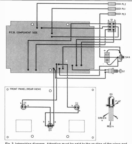
Fig. 3. Interwiring diagram. Attention must be paid to the routing of the wires and this will depend upon the positions of the switches, i.e.d.s and sockets.
