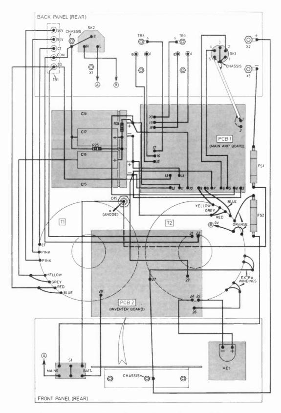
Fig. 3.13. Public Address System: Power Amplifier final assembly and wiring details.
