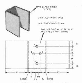
Fig. 3.2. Heat sink constructional details.
