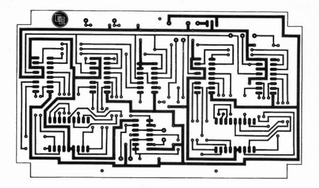
Fig. 2. Full size printed circuit board artwork and component layout for the Lap Counter and Judge.
