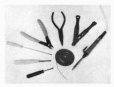
Fig. 4. The basic tool kit with, clockwise left to right, small cross-head screwdriver, spot-face cutter, small plain screwdriver, wirecutters, long-nosed pliers, wire strippers, mains soldering iron and in the centre, a reel of solder.
