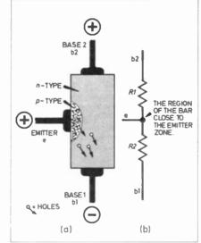
Fig. 10.2. (a) Construction of a unijunction transistor (b) equivalent circuit of a unijunction—it acts as a potential divider.
