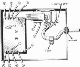
Fig. 3. Wiring diagram showing view inside case. Transformer and case must be earthed via the earth point on the tag strip.
