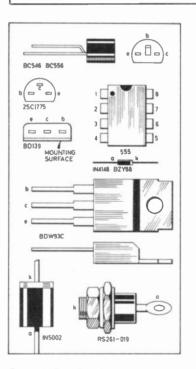
Fig. 3.9. Details of semiconductors used in power amplifier (for power f.e.t.s see Fig. 3.10).
