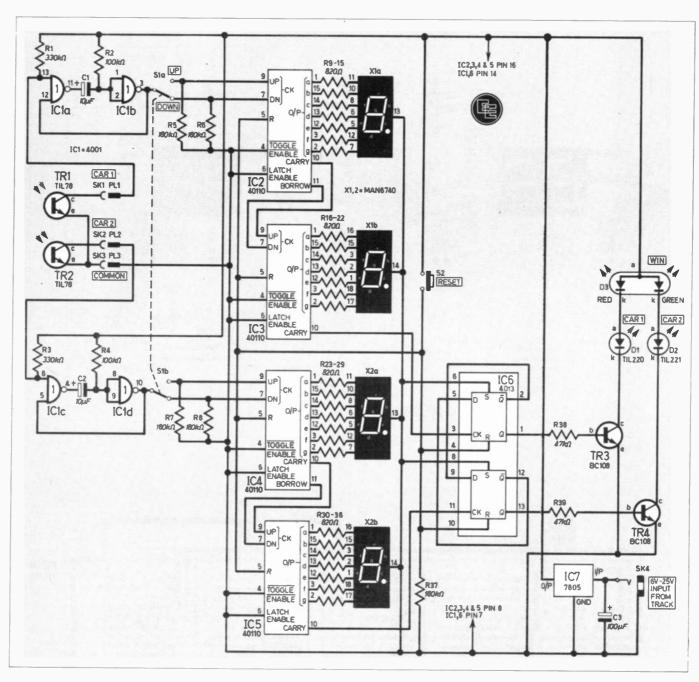
Fig. 1. Complete circuit diagram of the Model Car Lap Counter and Judge.
