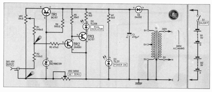
Fig. 1. Circuit diagram for the Comparator Voltmeter
