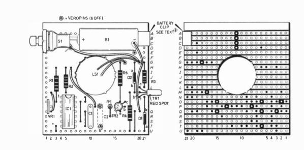
Fig. 2. Stripboard layout for the Pitch Pipe housed in the small transistor radio case shown in the photograph above. Note that this model employs the 15V battery (B1) and also has the speaker hole in the board. If a larger case is used, the layout may need to be modified accordingly to accommodate the larger PP3 battery and the new speaker position.
