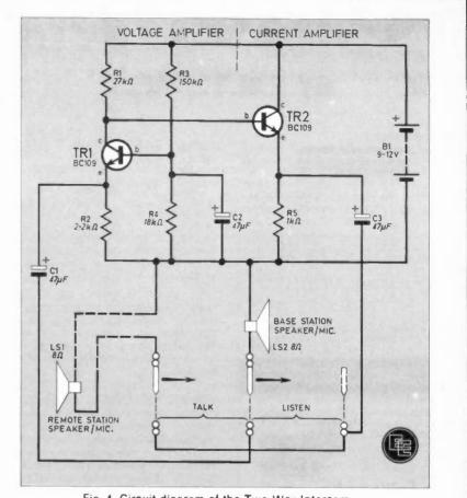
Fig. 4. Circuit diagram of the Two Way Intercom.
