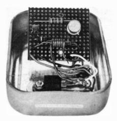
View inside the finished prototype showing the circuit board and power transistor mounting.
