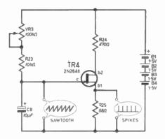
Fig. 10.1. Relaxation oscillator based on a unijunction transistor.
