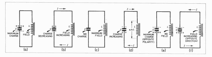
Fig. 10.5. An LC oscillator in various operational stages.
