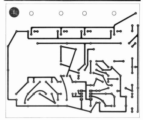
Fig. 3.6. Public Address System: Power Amplifier printed circuit board No. 2 (Inverter Board), actual size.
