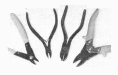
Fig. 1. A selection of wire cutters (these are also referred to as side cutters). The pair on the left are lap-jointed, the others all being the box-jointed type, the heavy duty pair in fact having two joints for extra leverage.
