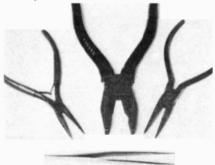
Fig. 3. A range of pliers with the electricians pliers in the centre, flanked by two pairs of long-nosed pliers. A pair of fine tweezers are also shown.
