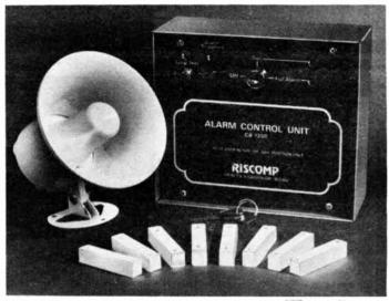
The Control Unit requires a limited amount of mechanical assembly with a little wiring to the key switch and I.e.d. indicators. Full constructional details are provided. Where required the system may be extended at a later date according to needs, and can be linked to both ultrasonic and infra red sensors. It provides two modes of operation with timed alarm and entry and exit delays.
