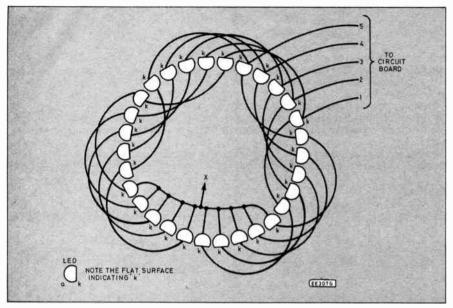
Fig. 4. Wiring to the display l.e.d.s D6 to D35. The polarity of the l.e.d.s can be ascertained by referring to the pinning diagram.
