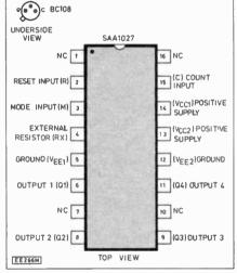
Fig. 2. Pinning details for the BC108 and SAA1027.
