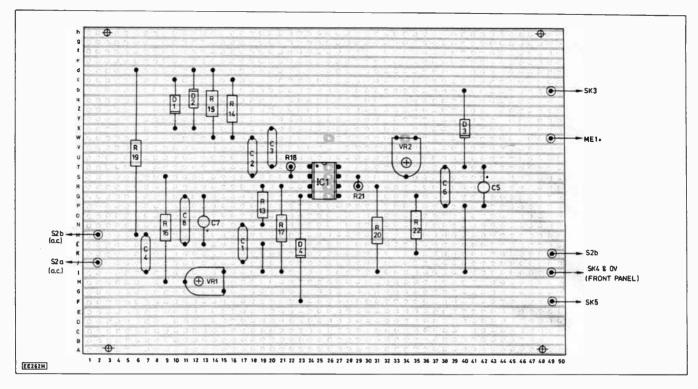
Fig. 4. Circuit board component layout and details of breaks to be made in the copper strips on the underside of the board. Breaks are required at Q26, R26, S26, T26, W26 and W34.
