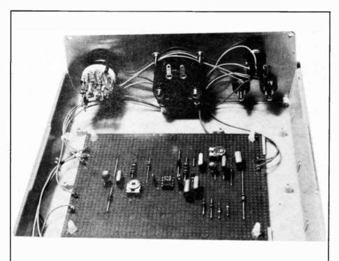
Wiring to the front panel range switch, meter, mode switch, input terminals and the solder pins on the circuit board.
