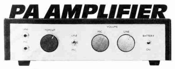
Twenty watts r.m.s. for around £20. Designed for the home constructor using just three i.c.s and a handful of discrete components. This unit is capable of a respectable performance while still being inexpensive to build.
