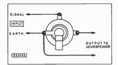
Fig. 2. The 3-5mm jack sockets normally have a break contact which can be used in this fasion. In many applications the switched output is not required, and the third tag is left unused.
