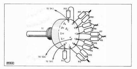
Fig. 7. Range selector switch S1 detailed assembly. The "free ends" of the resistors should be twisted together in pairs and soldered.
