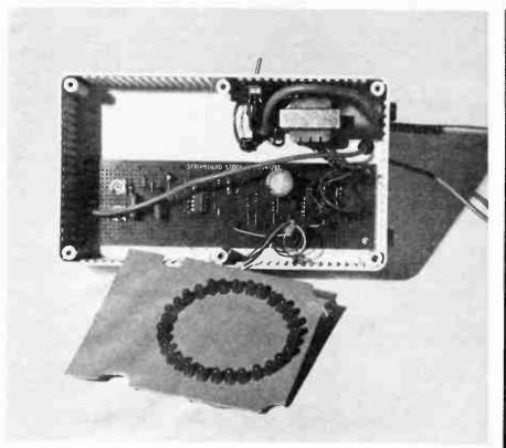
The completed Circle Chaser with the display card removed
