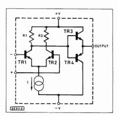
Fig. 7.3. Simplified internal circuitry of an operational amplifier.
