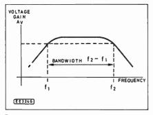
Fig. 7.16. Frequency response for the arrangement shown in Fig. 7.15.
