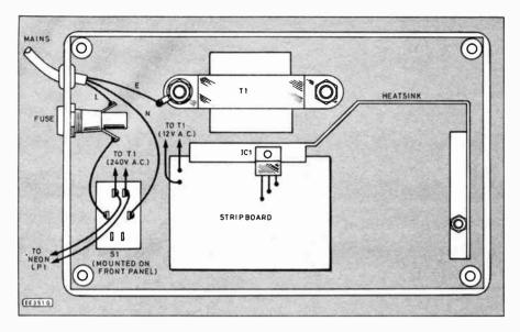
Fig. 5. Layout of components inside the case and wiring to the power supply section.
