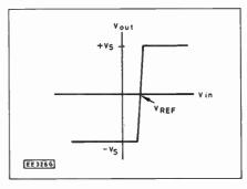
Fig. 7.18. Transfer characteristic of the arrangement shown in Fig. 7.17.
