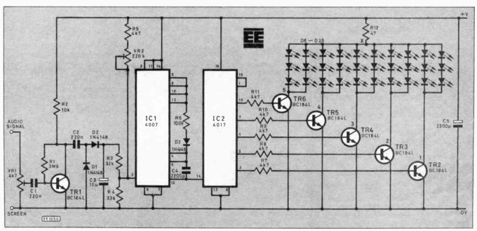
Each transistor is connected to two of these groups, wired in parallel with each other. Thus with the value of R12 shown, a total of about 40mA is used by the six l.e.d.s lit at any one time.
