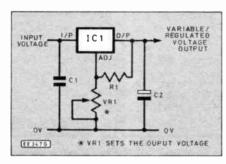
Fig. 1. Basic regulated voltage circuit.
