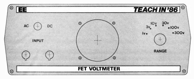
Fig. 5. Front panel layout (full size).
