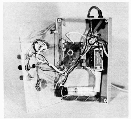
be shaped and positioned to avoid touching other components or wires. One end is fixed to the i.c., and the other end bolted to the plastic case. A small piece of stripboard may be fixed between the aluminium and plastic, to prevent heat damage.
