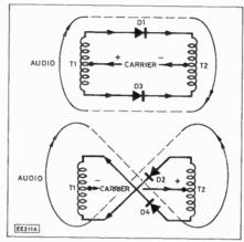
Fig. 3 (top). The diodes conduct in pairs. One half cycle of the carrier makes D1 and D3 conduct. On the other half cycle (Fig. 4 above) D2 and D4 conduct.
