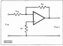
Fig. 7.4. A practical inverting amplifier.
