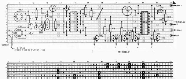
Fig. 3. Component layout, underside showing breaks (44 off) in the copper strips and interwiring details. Use screened cable for the input signal lead.
