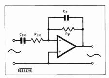
Fig. 7.15. Bandwidth limited amplifier.
