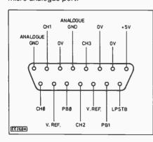
to it are accordingly made by way of a matching 15-way "D" type plug, although I have found it possible to use one millimetre plugs as a cheaper solution in cases where only two or three connections are to be made. Fig. 1 gives connection details for the analogue port.
