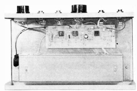
Completed Stereo Reverb showing positioning of printed circuit board, springline and wiring to front panel components.
