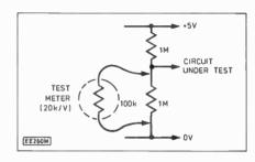
Fig. 1. Voltmeter impedance effects.
