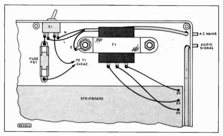
Fig. 5. Wiring details for the mains power supply. The mains lead should be held in position by a plastics P-clamp.
