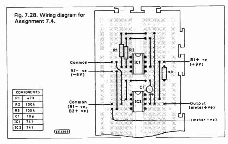
The output consists of a triangular waveform of approximately 9V pk-pk and frequency 0.5Hz. At the low operating frequency, the nature of this waveform can readily be recognised by simply observing the meter deflection. If time permits, readers may like to experiment with a range of values for C1 (say, 1µ, 100n, 10n and 1n). If a square, rather than triangular, output is required this may be obtained simply by taking the output from the first stage (i.e. pin-6 of IC1).
