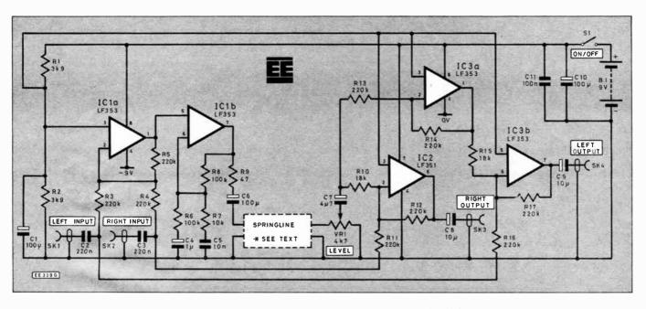
Fig. 2. Full circuit diagram of the Stereo Springline Reverberation Unit.
