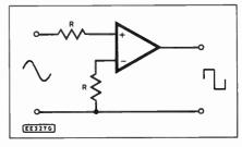
Fig. 7.19. Square wave converter.
