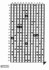
Fig. 4. Veroboard layout and wiring for the Freeloader. The board is mounted by SK1 and SK2.
