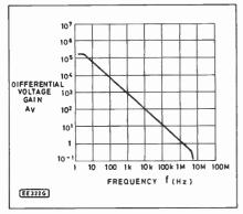
Fig. 7.14. Typical frequency response of a 741.
