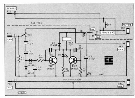
Fig. 1. Complete circuit diagram of the Freeloader when powered by the cassette recorder.
