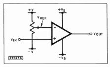
Fig. 7.17. An operational comparator.
