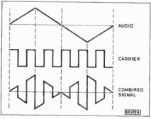
Fig. 4. The effect of combining the audio and carrier waves.
