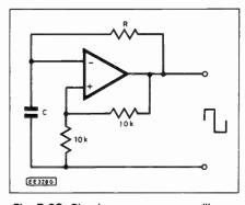
Fig. 7.20. Simple square wave oscillator.
