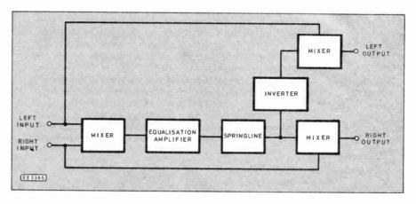
Fig. 1. Block diagram of the Stereo Reverb.
