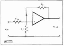
Fig. 7.5. A practical non-inverting amplifier.
