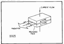
Fig.14. Schematic diagram of a semi-conductor laser.
