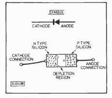
Fig.1. The diode
