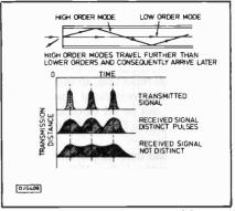
Fig.12. Signal dispersion caused by multiple ray paths.
