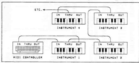
Fig.1. The "chain" method of connection
