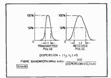
Fig.11. Measurement of dispersion
