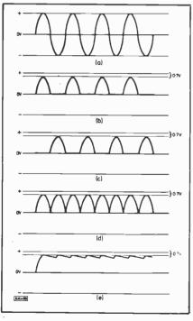
Fig.5. Full wave PSU output waveforms. (a) At T1. (b) At D1. (c) At D2. (d) At D1/D2, without C1. (e) At D1/D2 with C1.
