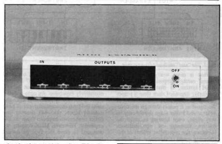
the chassis tags of the plugs. With five outputs the unit should be adequate for most systems, but if necessary a few additional sockets and current limiting resistors could be driven from TR1, or two expanders could be wired in series to give nine outputs. Another alternative would be to use a mixture of "star" and "chain" connection.
