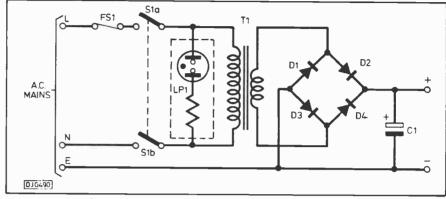
Fig.6. Basic bridge rectifier circuit (mains version)
