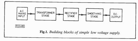
by connecting a load to the secondary coil, the energy being drawn must be supplied from the primary coil and therefore from the mains input. The transformer operates by converting the electrical energy from the current in the primary coil into an alternating magnetic field in and around the core of the transformer.
