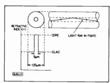
Fig.6. Monomode transmission
