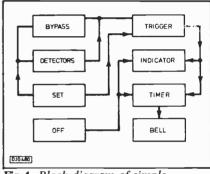
Fig.4. Block diagram of simple controller.
