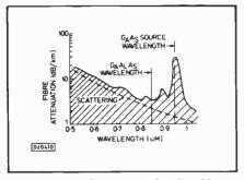
Fig.10. Spectral response of a silica fibre
