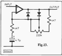
To illustrate this, consider the circuit shown in Fig. 13. This is a stage from Robert Penfold's "Bright Fuzz" design (PE May 1987). The diodes are used to clip the audio signal and produce the well known fuzz sound. The maximum reverse voltage which the diodes experience is about 0.6V. The peak current is
