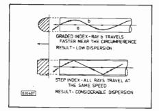
Fig.9. Transmission of graded and stepped index fibres
