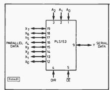
Fig.14. FPLA 8:1 bidirectional multiplexer/demultiplexer
