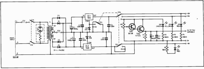
Fig.14. Final design with  $\pm 9V$ , +5V, and variable 0V to +7.5V outputs.
