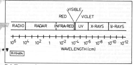
Fig.1. Electromagnetic spectrum
