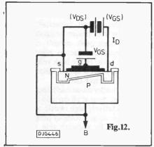
ideal for transistor action, but under some circumstances this "parasitic transistor" can conduct and cause trouble. For this reason, some f.e.t.s. of this type have a connection to the substrate, which should be connected (in the case of an N channel f.e.t.) to a point in the circuit more negative than the source (0V or the negative power supply). This biases off the parasitic transistor and allows the f.e.t. to work as expected.
