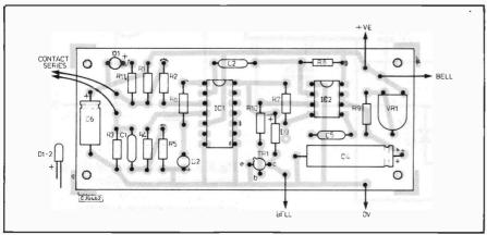
Fig.6. PCB details for simple alarm controller.
