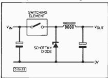
Fig.16. Part of switched mode power supply
