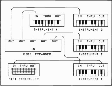
Fig.2. The "star" method of connection.
