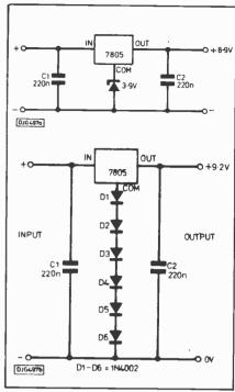
**Fig.13.** Two methods of increasing +5V output to approximately +9V.
