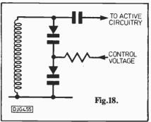
has no harmonics anywhere near the frequency of BBC 1 can totally obliterate reception of said channel. The interfering harmonics are being produced in the television tuner itself, because it uses varicap diodes to provide electronic tuning. This effect can be minimised by using back to back varicaps as illustrated in Fig. 18.
