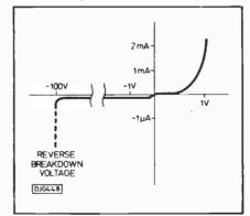
Fig.2. Diode characteristics.
