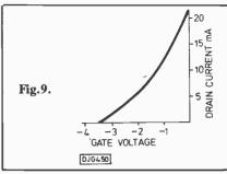
It is also possible to produce a f.e.t. which is normally in the non-conducting state, and which can be made to conduct by application of a gate voltage. In this case, the gate must be insulatated from the channel, or else the gate-channel junction would be forward biased and gate current would flow.
