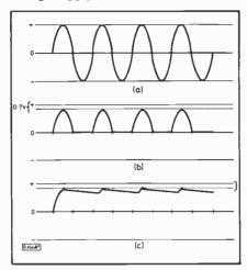
Fig.3. Half wave PSU waveforms (a) a.c. output at T1. (b) Output after D1. (c) Output at C1.
