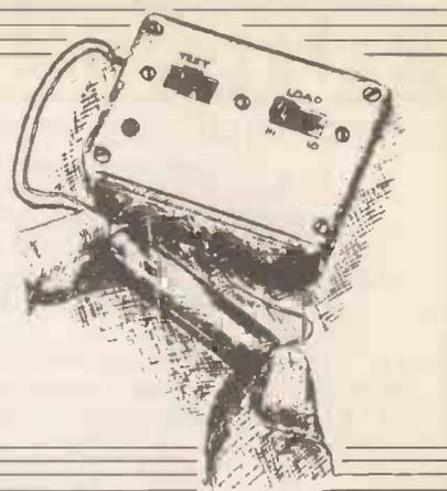
**T**HIS circuit checks 1.5V cells of all sizes and types apart from the nickel-cadmium (rechargeable) variety. By using an l.e.d. indicator, the cost of a meter is avoided and this reduces constructional costs.
