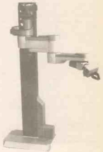
from which an arm, a plotter and a buggy can be made as well as a number of other devices, which can be controlled by computer. Servos with optical encoders are available as are programs and interface for BBC, and a battery-powered controller. Special kits for secondary and primary schools. Prices vary.
