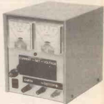
A superb design giving 0-25V and 0-2.5A. Twin panel meters indicate Voltage and Current. Voltage is variable from zero to 25V. Current-Limit control allows Constant Current charging of NICAD batteries, and protects circuits from overload. A Toroidal transformer MOSFET power output device, and Quad op-amp IC design give excellent performance.
