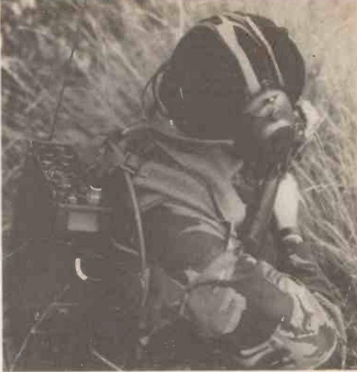
*The Scimitar communications system made by Marconi is actually a family of several radio products, from pocket size up to vehicle-mounted systems. Digital data and voice communications can be transmitted on up to 284,000 channels and the system can automatically hop between channels at great speed to evade jamming.*
