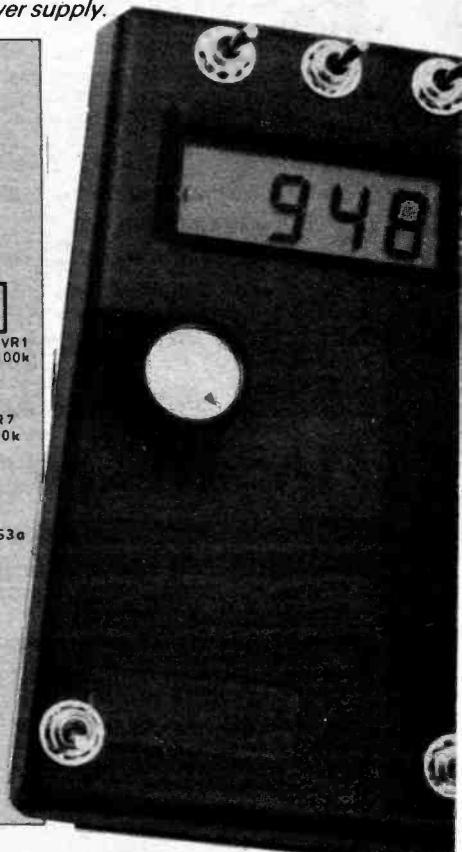
when VR5 and VR6 have been set to the relative span ranges for their mode scales, a common increase or decrease to the altitude and barometer mode gains can be effected by adjusting VR8.
