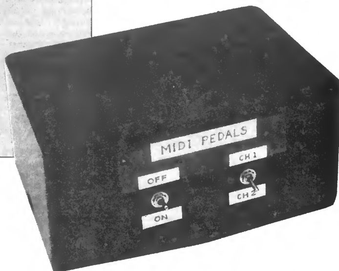
The completed keyboard scanner unit showing the MIDI Channel select switch and On/Off switch. These switches could be mounted on one of the side panels, away from any "flying feet."
