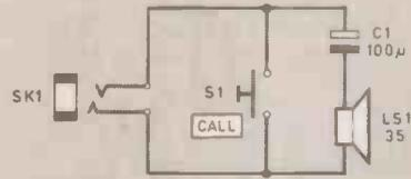
little comment other than that S1 (a normally open push button switch) places a short-circuit across the line whenever it is operated. Such a short-circuit causes TR1 to conduct and thus enables the d.c. supply to the tone oscillator circuit of TR4 and TR5.
