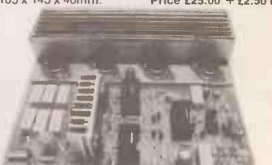
TA 3600 Mono power amplifier for professional/domestic applications requiring high output power. Output Power 300 Watts sine wave into 8 Ohms. Frequency response 10Hz-20KHz (-3dB). T.H.D.0.05%. Sensitivity 1.4V for rated output. Requires only D.C. supply of +/-60 to 75V at 8 Amps and a case to complete a really good quality high power slave amplifier. Size Approx. 225 x 180 x 57mm.
