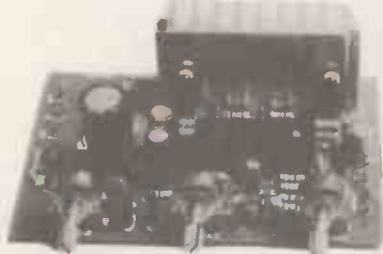
TA 300 mono pre/power amplifier. Output power 30 Watts R.M.S. into 8 Ohms. Frequency Response 20Hz-20KHz (-3dB). Two band tone controls. Dual input sensitivity 50mV and 150mV. Harmonic distortion 0.1%. Size approx 125 x 85 x 40mm.
