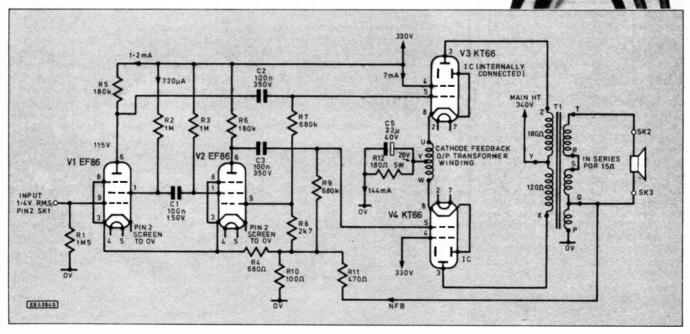
Fig. 2. Complete circuit diagram for the Quad II Power Amplifier. (Courtesty Quad.)
