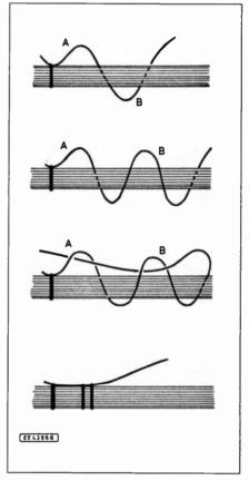
Fig. 14. Basic technique for lacing up the wiring loom.
