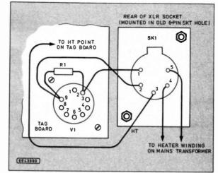
Fig. 15. Wiring to the new 5-pin ''female'' XLR socket.
