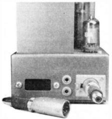
Photo. 9. Adding a 5-pin XLR to phono socket. Only pins 1 and 2 are connected.
