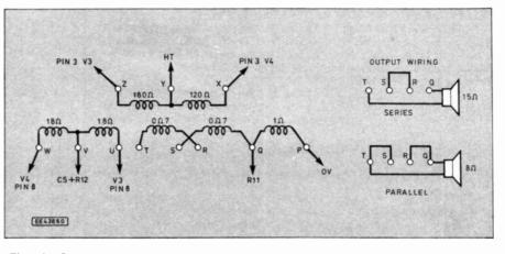
Fig. 4. Output transformer pinout details and typical d.c. resistances of the windings. Bottom view of output transformer. Check also for interwiring shorts, especially between Y and P.
