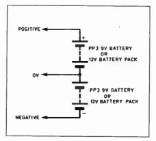
Fig. 6. Using two sets of PP3 batteries or battery packs to power the preamplifier p.c.b. (excluding the 48V supply).
