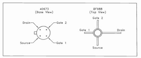
Fig. 1. Connections for the 40673 and BF988.
