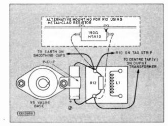
Fig. 11. Biasing components wiring. Resistor R12 can be, replaced with a metal-clad type (shown dotted) if desired.
