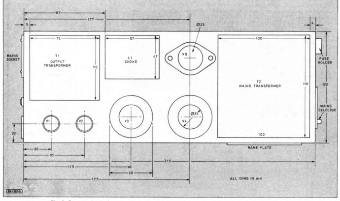
Fig. 3. Chassis dimensions and layout of the inductive components and valves on the topside.
