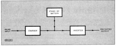
Fig. 1. Block diagram of on-line U.P.S.
