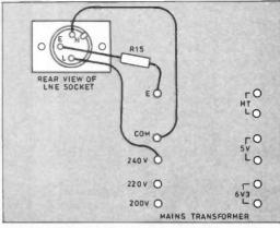
Fig. 6. New mains wiring to the Cannon connector.
