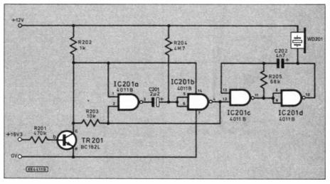
Fig. 6. Mains failure alarm circuit.
