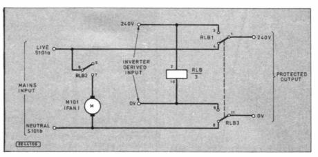
Fig. 5. Failsafe switching circuit.
