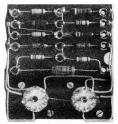
Photo. 6. Rebuilt tag board ready for installation into the chassis.
