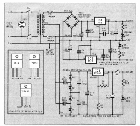
Fig. 7. Circuit diagram for a mains powered dual-supply and a 48V supply.
