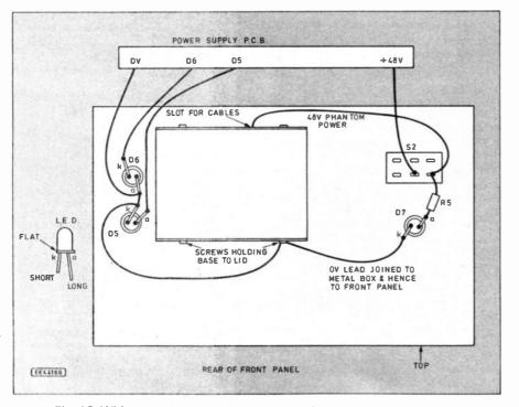
Fig. 12. Wiring to components mounted on the rear of the front panel.
