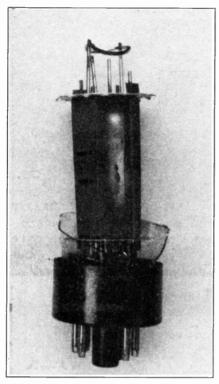
Photo 3. "Spotted" anode on an EL34 valve, a result of excessive dissipation.
