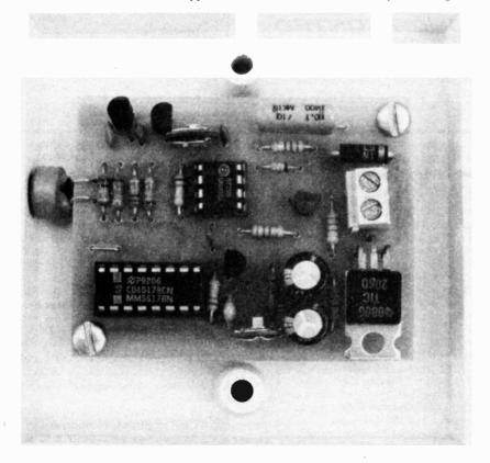
soldering low profile components such as resistors and diodes first, paying particular attention to component orientation where this is important (i.e. with diodes, electrolytic capacitors etc). Make sure also that components are pushed down onto the board and not left standing on long leads which could touch adjacent components or even the wall box with potentially disastrous consequences.
