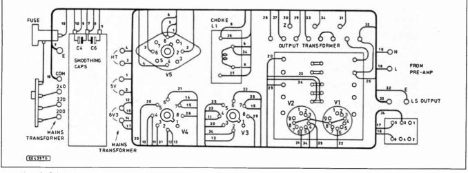
Fig. 13. Original wiring loom for the Quad power amplifier. If a new loom is made up use multi-coloured wires wherever possible, see Fig. 6 for new mains input wiring.
