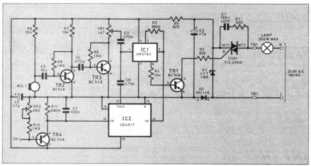
Fig. 1. Complete circuit of the Whistle Controlled Light Switch.
