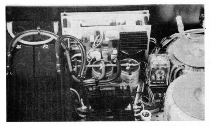
Layout and mounting of the U.P.S. components; batteries and TR105 heatsink are on the left.
