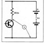
Fig. 2.10. What is the voltage at the collector?
