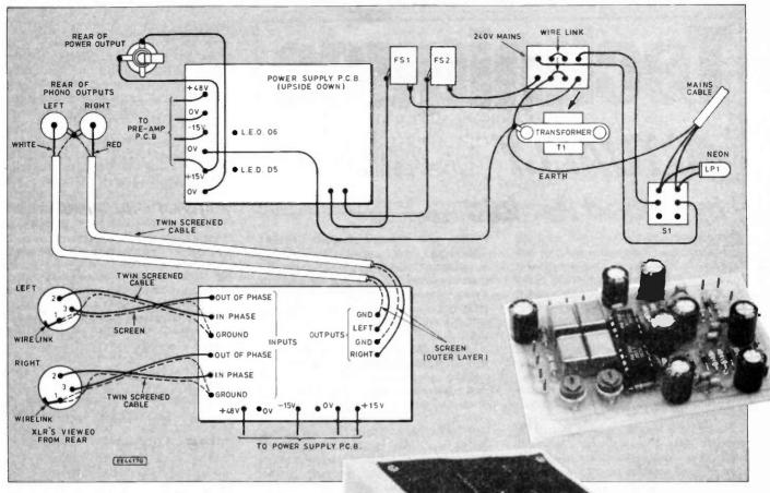
Fig. 13. Interwiring between boards.
