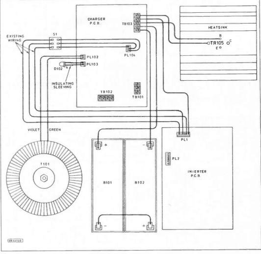
Fig. 9. Signal wiring for the U.P.S.
