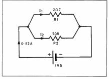
Fig. 2.3. How does the current divide in this circuit?
