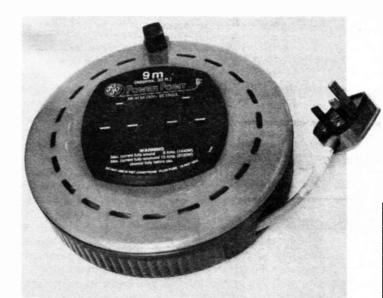
A commercial extension lead showing the coiled (6A) rating and the fully unwound (13A) rating inscribed on the cable housing.
