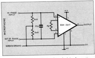
Fig. 3. Simplified circuit showing principle of operation.
