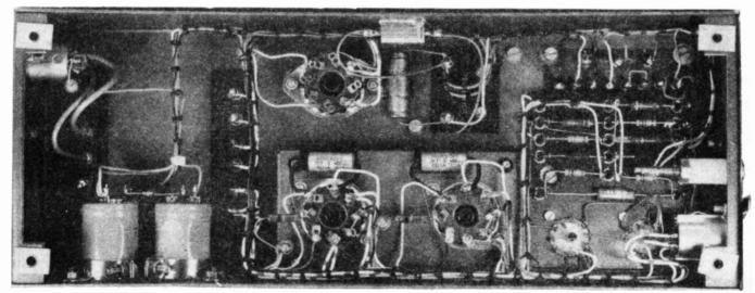
Photo. 7. Underside view of a completely rebuilt Quad showing new wiring loom, tag board and metal-clad resistor.
