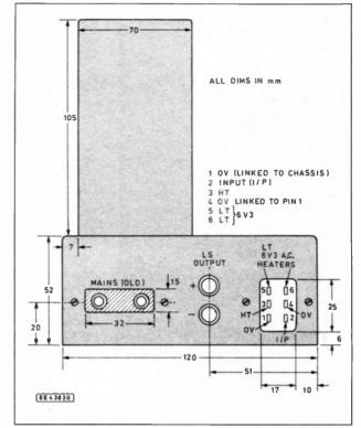
Fig. 1. Pinout details for the original six-pin Quad II connector.
