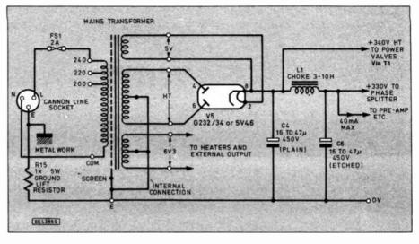
Fig. 7. Circuit diagram for the valve Power Supply. Note that the "ground-lift" resistor R15 is a 5W wirewound type.
