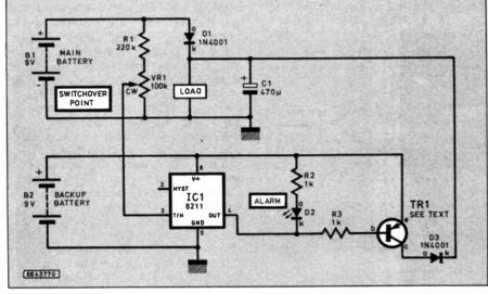
Fig. 2. The automatic battery back-up circuit.
