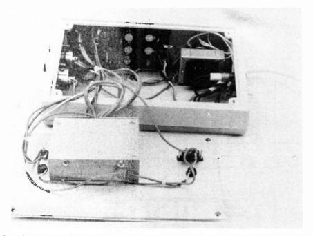
Completed preamplifier showing wiring to front panel l.e.d.s and on/off switch. The position of the "screening box" is also shown.
