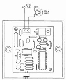
Fig. 5. Wiring to the mains supply and the load.
