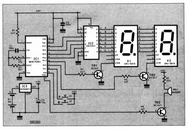
Fig. 1. Complete circuit diagram of Timeout. IC1 is the microcontroller.
