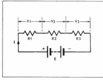
Fig. 2.1. A series circuit where I flows through each resistance and  $E = V_1 + V_2 + V_3$ .
