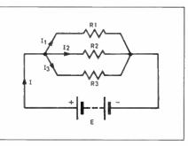
Fig. 2.2. A parallel circuit where E volts is applied to each resistance and  $|=|_1+|_2+|_3$ .
