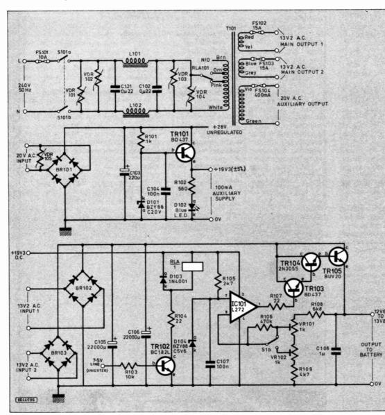
Fig. 4. Battery charger circuit for the U.P.S. R103 is connected to D2 cathode in the Inverter circuit.
