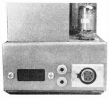
Photo. 8. Blanking of the old mains input socket cutout.
