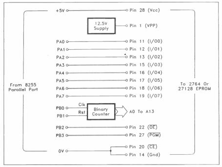
Fig. 3. Suggested method of controlling an EPROM via an 8255 or similar PIA.
