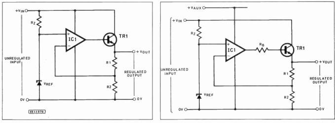
Fig. 2. Simple regulated linear p.s.u.
