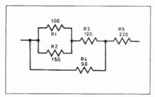
Fig. 2.8. What is the equivalent resistance of this circuit?
