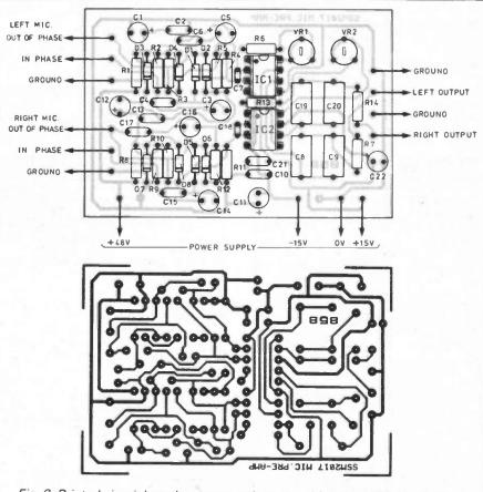
Fig. 8. Printed circuit board component layout and full size p.c.b. foil pattern.
