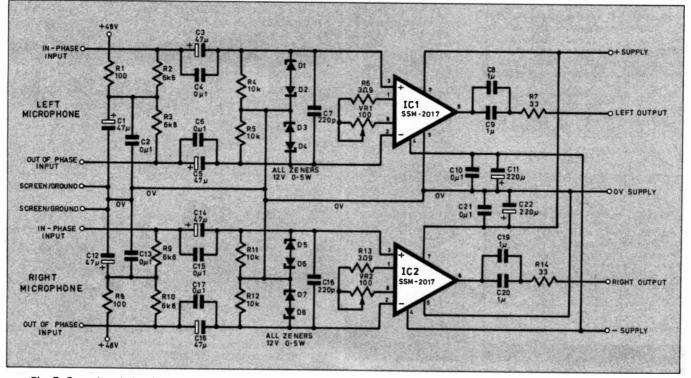
Fig. 5. Completed circuit diagram for the Balanced Stereo Microphone Preamplifier. The circuit gain is set by VR1/VR2.
