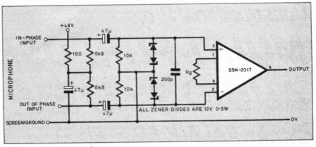
Fig. 4. Phantom powered microphone circuit diagram.
