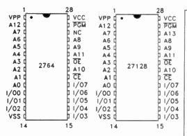
Fig. 1. Pinout details of the 2764 and 27128 EPROMs. Fig. 2. (right) Using a 14 store ring a counter to
