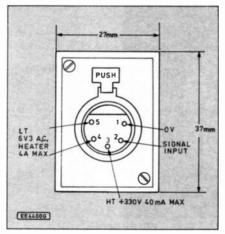
Fig. 16. Pinout details for the XLR socket.
