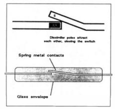
Fig. 1. A glass encapsulated reed switch.
