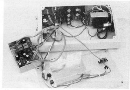
The preamplifier removed from the screening box showing the cable entry cut out.
