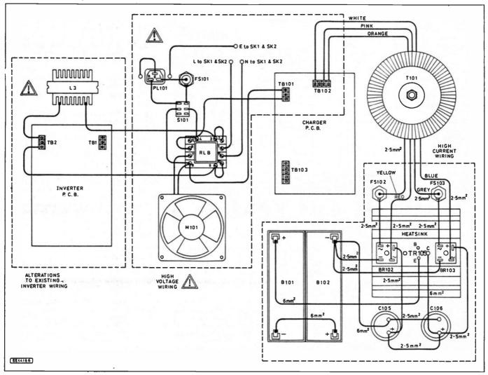
Fig. 11. High voltage and high current wiring for the U.P.S.
