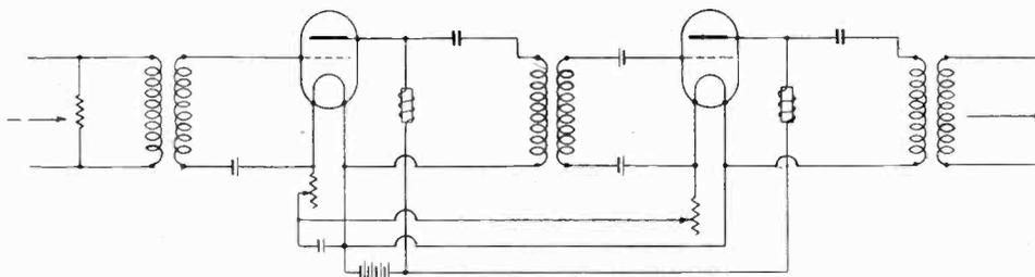
Fig. 1a. Circuit of amplifier employing tuned transformers.
