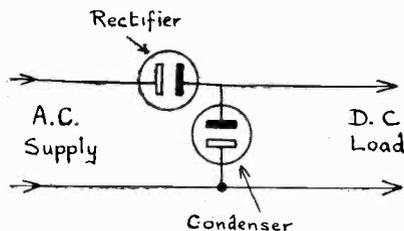
Fig. 5. Use of Electrolytic Condenser.
