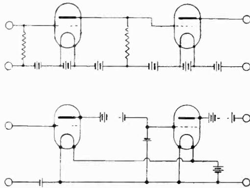
Fig. 2. Battery coupled amplifiers.
