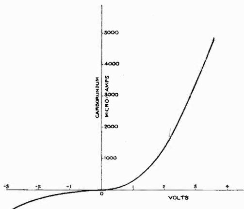
Fig. 5. (b.) Carborundum Crystal Rectifier.
