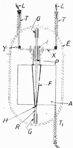
are bound at *Y* to the filament leads *L*, which are sealed into tubes *T*. The anode is shown at *A*, and the lead is taken through another tube *T*<sub>1</sub>, which is sealed in in the normal manner.
