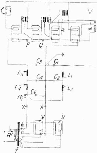
transformer. The secondary of this transformer is connected between the grid and the upper end of the aerial inductance, and it is stated that the valve functions as an ordinary low frequency amplifier. It is perfectly obvious that the scheme functions, and no doubt functions very well, but
