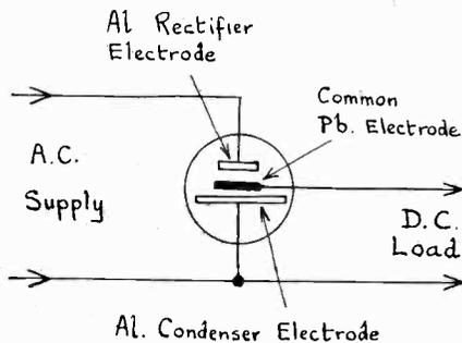
Fig. 6. Messrs. Siemens' Connection.
