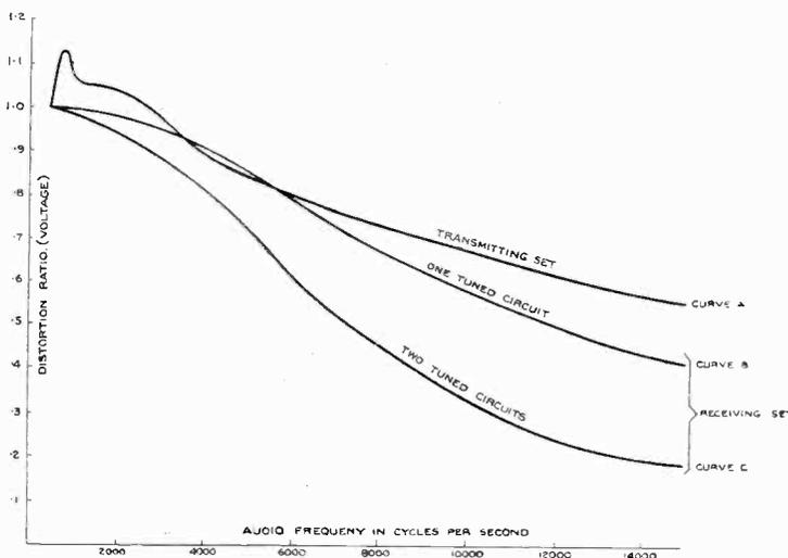
Fig. 3. Diagram indicating distortion in transmitting and receiving set due to tuning circuits.
