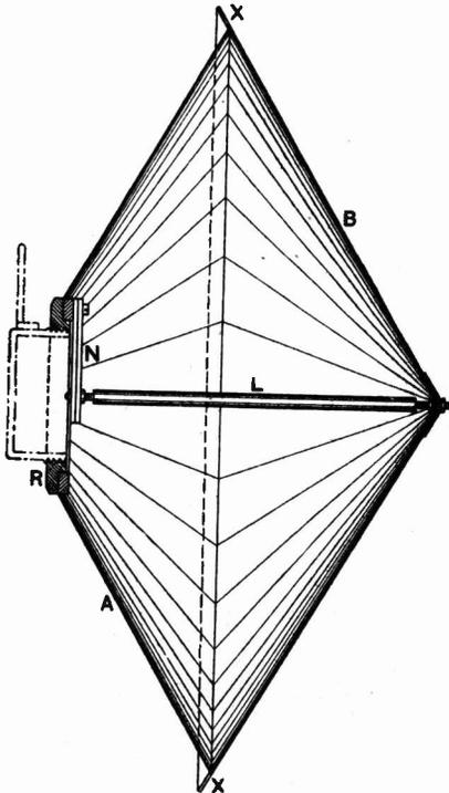
comprises two cones *A* and *B*, fixed together at their bases at *X*. The cone *A* is truncated and fixed to a ring *R*. The apex of the cone *B* is provided with a link *L*, the other end of which terminates in the region of the ring *R*, where it is connected to some actuating mechanism. This may either be an electro-magnetic device such as the diaphragm of an ordinary telephone receiver, or the link may be connected directly to a balanced armature. The specification also provides for
