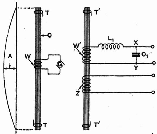
A suitable reception aerial and its associated circuits is shown on the right of the illustration. Similar short-circuited turns *T*<sub>1</sub> are shown for the purpose of tuning, and a similar winding *W*<sub>1</sub> is
