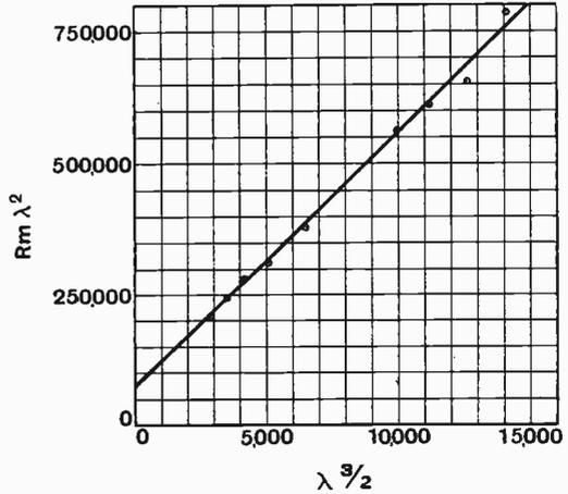
Fig. 5. Showing how  $A'$  and  $B'$  in the formula  $R_m = \frac{A'}{\sqrt{\lambda}} + \frac{B'}{\lambda^2}$  (26) may be found by plotting  $R_m \lambda^2$  against  $\lambda^{3/2}$  and finding the slope ( $A'$ ) and the intercept on the vertical axis ( $B'$ ) of the resulting straight line.
