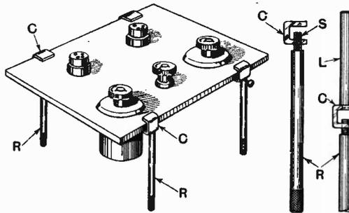
portion *S*, which co-operates with a thread in a small channel *C*. The legs are attached to the panel by placing the channel on the edge of the panel, and rotating the rod until the end of the screwed portion bites the under surface of the panel. Another modification of the leg consists in providing the channel *C* with another link or rod *L*, thereby enabling the panel to be inverted for the purpose of working on the opposite side.
