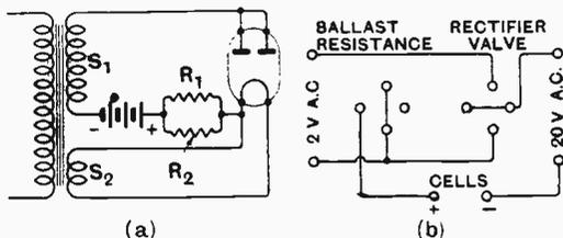
Fig. 3. The circuit and wiring diagrams for half-wave rectification.
