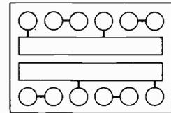
Fig. 12c. Three circuits in series, paralleled to the cups.
