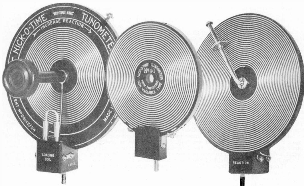
wound in spiral grooves cut in both faces of an ebonite disc. In the first three coils tuning is effected by a rotating arm carrying a small grooved wheel which runs on the wire, and as the arm is rotated the number of turns of the coil in circuit is altered. The arm and wheel are held in good contact with the wire by means of a fairly strong spiral spring concealed in the long bearing for the arm.
