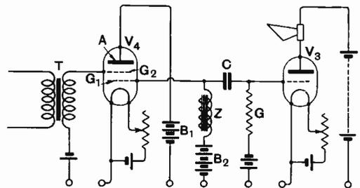
electrode valve, which is associated with the usual loud-speaker and batteries. The invention states that the overall magnification approximates to an inverse function of the frequency, and is very high for audio-frequencies. It is further stated that the
