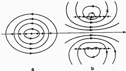
Fig. 4 (a) shows the symmetrical distribution of the lines of force about the central turn of a very short solenoid; (b) shows the distribution of the lines of force in a long solenoid when the central turn is present (upper part of figure) and when it is absent (lower part of figure).
