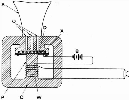
support and also tends to reduce any natural period. A central pole piece  $P$  is provided with a winding  $W$ , to which speech current is applied. The ends of the coil diaphragm are connected to a source of direct current in the form of a battery  $B$ . Thus it will be seen that there is a steady flux surrounding the actual diaphragm, due to the passing
