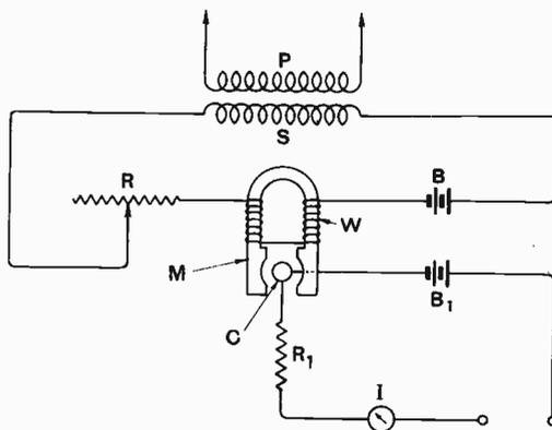
within the small air gap is a coil *C* made of bismuth or antimony alloys, the coil preferably being in the form of a ribbon. The coil is in series with another battery *B*<sub>1</sub>, an indicator *I* such as a telephone or galvanometer, and a resistance *R*<sub>1</sub>. It is stated that the passage of an oscillatory current through
