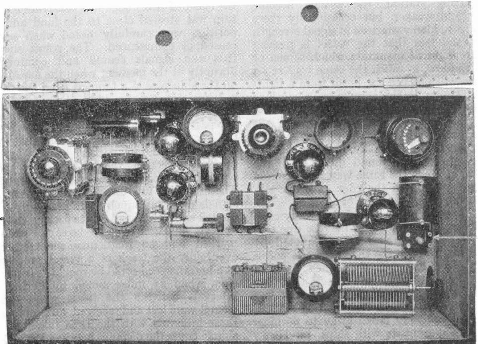
The photograph shows an American crystal controlled transmitting set. The master oscillator (driven by the crystal) operates at 209.4 metres, and the fifth harmonic (41.88 metres) of this is amplified in succeeding valves until the desired output is obtained.
