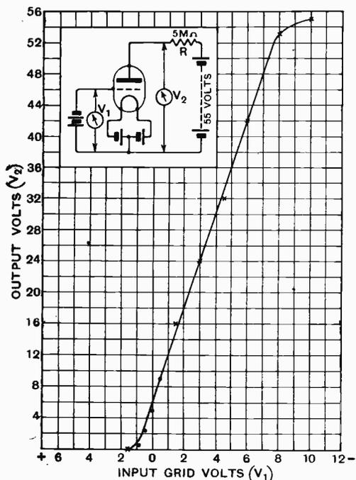
type of valve. The readings denoted by  $\times$  were taken on an electrostatic voltmeter while those with the circle were taken on a Moullin type voltmeter.
