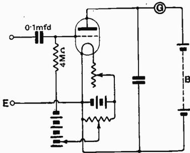
Fig. 32. Connections of the slide back voltmeter, Type V., using a grid condenser and leak.
