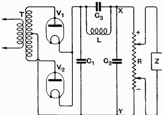
$V_1$  and  $V_2$ , the valves being used for full wave rectification in conjunction with a centre tap on the secondary of the transformer. The output of the rectifier is taken through a form of  $\pi$  filter comprising two condensers  $C_1$  and  $C_2$ , on either side of an inductance  $L$  shunted by a capacity  $C_3$ . Normally, the load, such as the current used by a
