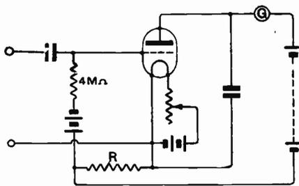
Fig. 35. Connections of a reflex voltmeter, using grid condenser and leak.
