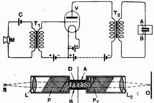
light to change in intensity. Since the rotation of the plane of polarisation occurs simultaneously with variation of voltage that is, there is no lag, the device is readily applicable to television purposes.
