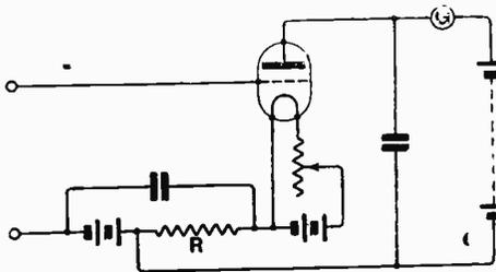
Fig. 33. Connections of the reflex voltmeter, Type VI.
