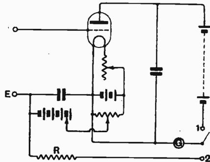
Fig. 25. Connections for measurement of the grid bias on the anode microammeter.
