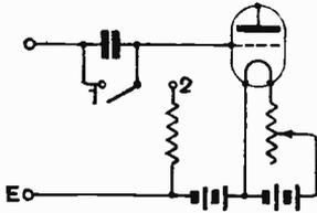
Fig. 31. A method of effecting a change over from the Type IV. voltmeter to Type I.
