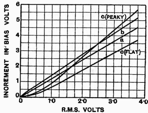
Fig. 28. Calibration curves of the Type III. voltmeter on wave forms (a), (b), (c).
