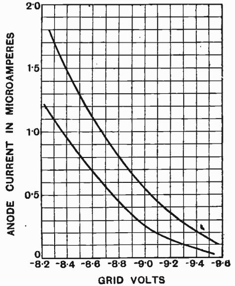
Fig. 27. Anode current—grid bias curves, in the region of zero anode current, for two slightly different A.C. voltages.
