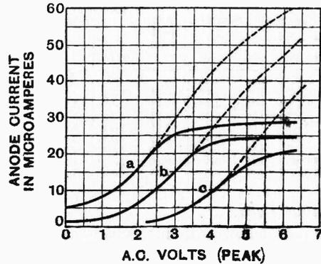
Fig. 30. Calibration curves of the Type IV. voltmeter.
