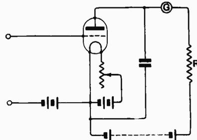
Fig. 34. The usual method of improving the degree of linearity of the scale of the Type I. voltmeter.
