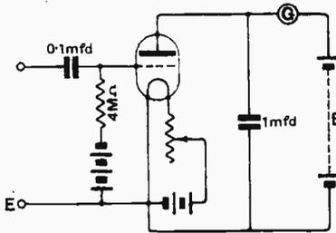
Fig. 29. Connections of the deflecting voltmeter, Type IV., rectifying on curvature of the anode characteristic but using a grid condenser and leak.
