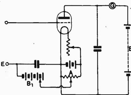
Fig. 24. Connections on the slide back voltmeter, Type III.
