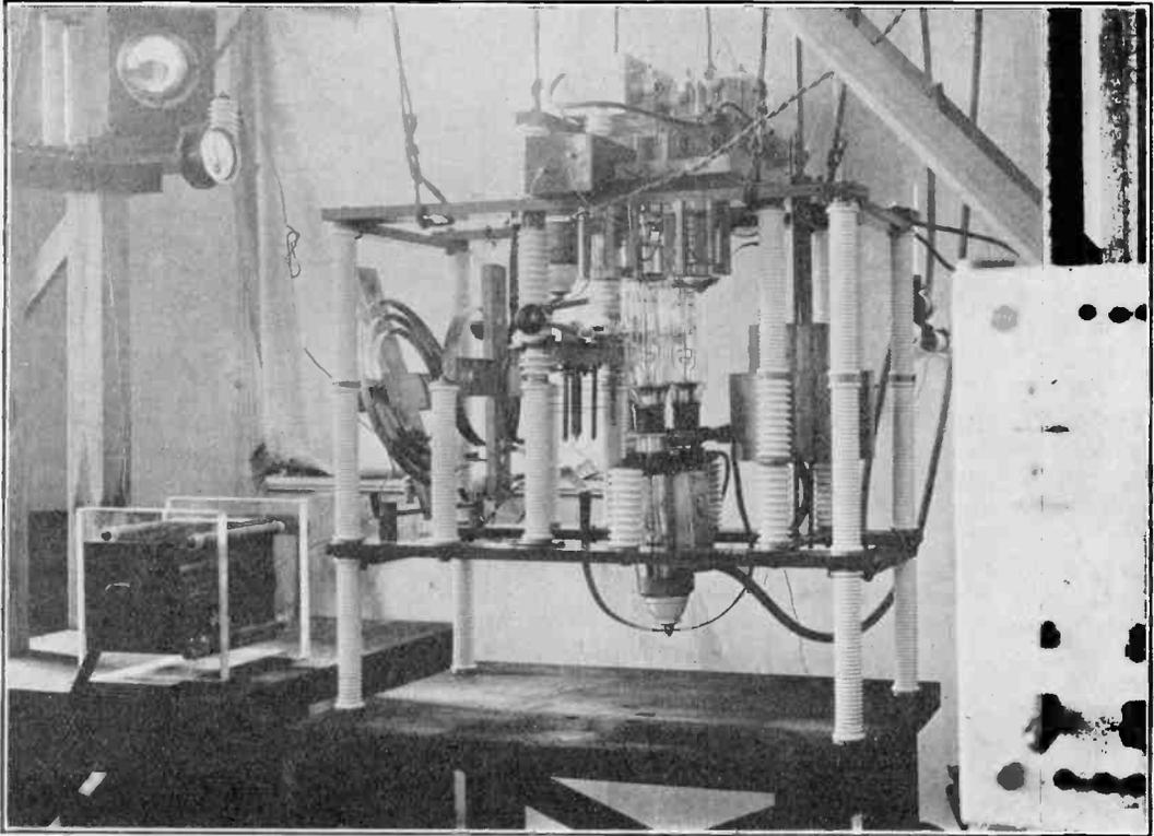
Fig. 11. Short-wave transmitter POW with two water-cooled valves.
