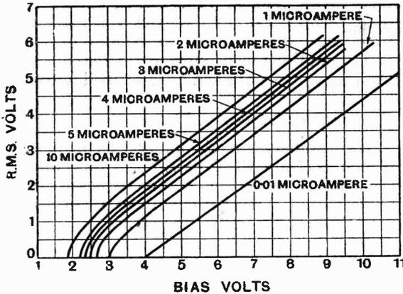
Fig. 26. Calibration curves of the slide back voltmeter, Type III.
