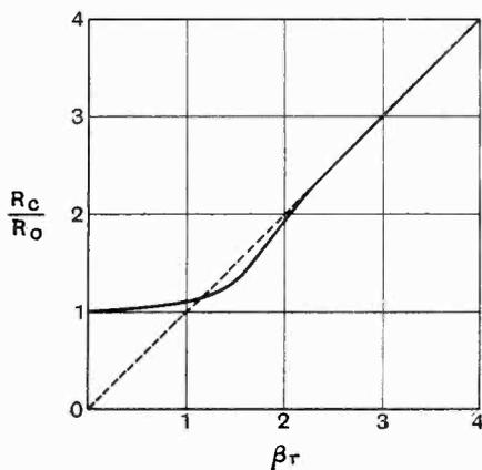
Fig. 12. Curve from Howe's paper on "The High Frequency Resistance of Wires and Coils."
