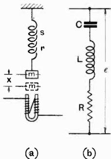
Fig. 6. (a) Mechanical analogy.
