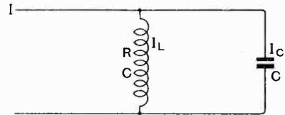
Fig. 2. Rough approximation to self capacity of inductance coil.
