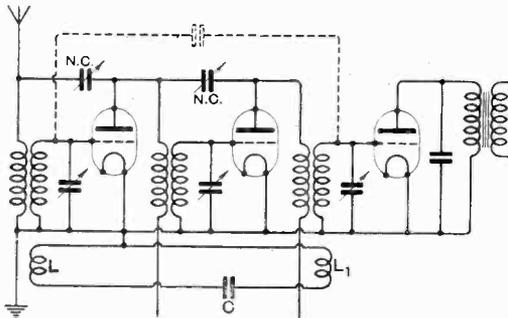
any other subsequent valve, so that at least two stages of valve amplification separates the two coils. The condenser  $C$  has a capacity of  $0.006\mu F$ . As shown the closed coupling-circuit is connected to the filament system.
