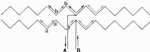
An element such as  $aa'$ ,  $bb'$  constitutes an antenna of one complete wavelength comprising two doublets of the same sign having the effect of increasing the directivity in the plane of the zenith. This system has been employed for communication between France and the Argentine on a wave of 14 metres 50 with favourable results.
