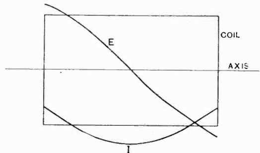
Fig. 8. Current and voltage distribution on a short coil forming part of a tuned circuit.
