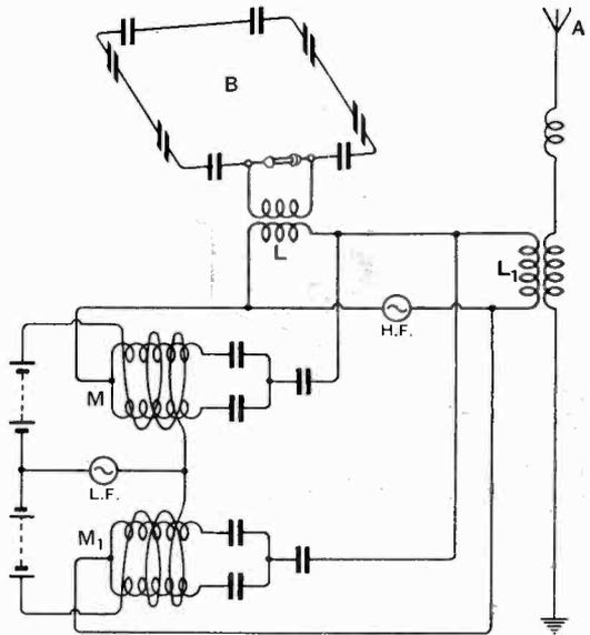
vertically polarised wave, and from a loop aerial  $B$  which produces a horizontally polarised wave. High frequency oscillations from the source  $H F$  are transferred alternately through a magnetic modulator  $M_1$  and coupling  $L_1$  to the aerial  $A$ , and through a second modulator  $M$  and coupling  $L$  to the loop  $B$ , the frequency of the change-over being controlled by a low frequency alternator  $L F$ .
