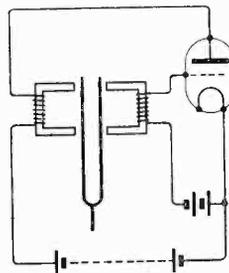
Fig. 1. Simple circuit of valve-maintained tuning fork.
