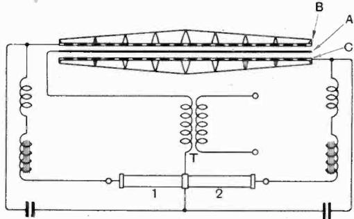
screens suitably supported, and are connected to the opposite poles of two dry piles 1, 2. The latter may be of the Zamboni type, formed of a number of adjacent paper discs coated on one side with black oxide of manganese and on the other with tin or silver foil.
