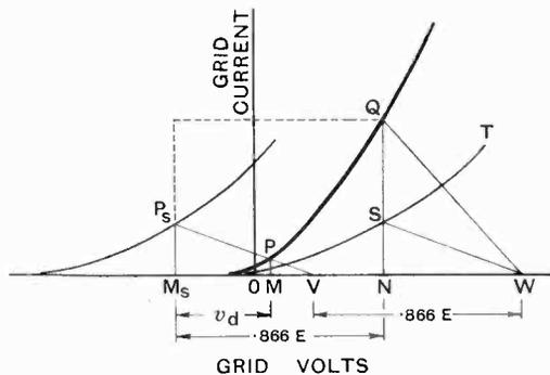
Fig. 7. Method of deriving mean grid signal voltage from the original characteristic. The length  $M_sM$  represents  $v_d$ , the grid voltage shift owing to rectification.
