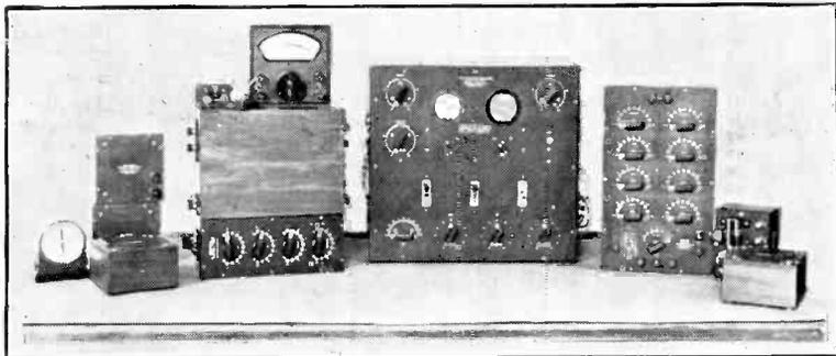
Three Inductance Standards; Left, Capacity Bridge with Decade Resistance; Centre, Vacuum Tube Beat Frequency Oscillator; Right, Decade Bridge; Extreme right, Audio Oscillator and another Inductance Standard.
