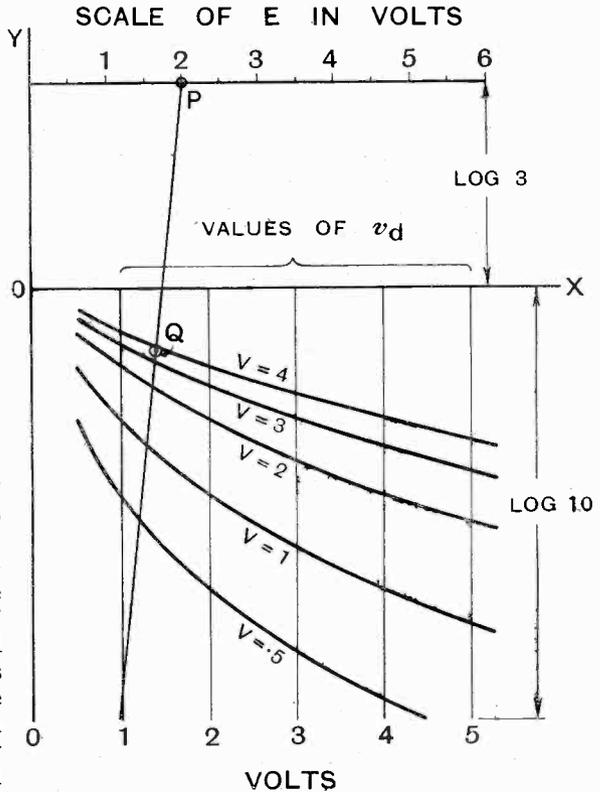
Fig. 12. Chart relating the quantities *E*, *V* and *v<sub>d</sub>* to *G*, the slope of the logarithmic characteristic. The point *P* corresponds to *E* = 2; the point *Q* corresponds to *V* = 3.88, *v<sub>d</sub>* = 1.34. The gradient of *PQ* is that of the characteristic shown in Fig. 9; the horizontal and vertical scales of Figs. 9 and 12 being in a fixed ratio.
