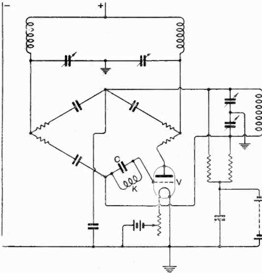
from this refinement, the general arrangement of the balanced bridge is identical with that described in a former patent No. 241,289 issued jointly to Mr. C. S. Franklin and the present inventor.
