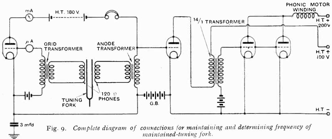
Fig. 9. Complete diagram of connections for maintaining and determining frequency of maintained-tuning fork.
