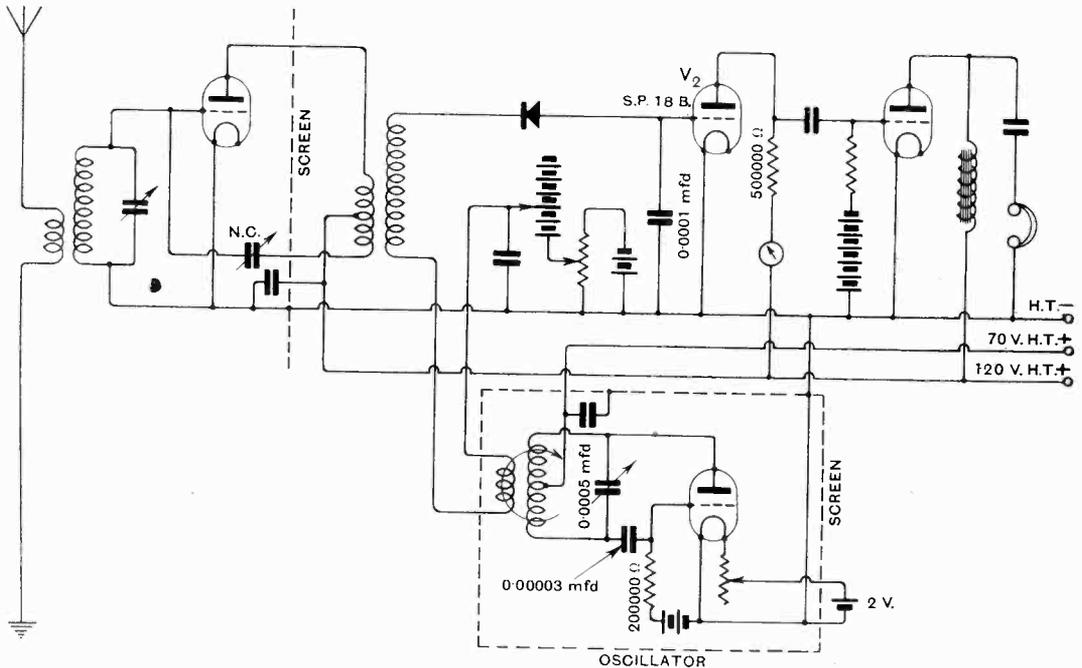
oscillations supplied produce a beat of infinite period with the carrier wave of the wanted station, audio frequency beats with its sidebands, and supersonic beats with the
