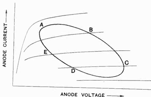
Fig. 2.—Illustrating static production of discontinuous changes in bulb-potential.
