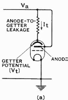
Fig. 5 (Right).—Determination of getter potential by "load-line diagram."
