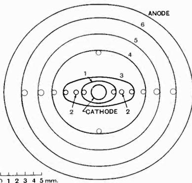
Fig. 1.—Cross section to scale of octode frequency changer valve type FC<sub>4</sub> (Mullard). The oscillator part consists of the cathode, grid one and grid two (oscillator anode). Grids three and five are interconnected and serve as screens. Grid four is the input signal grid. Grid six is a suppressor.
