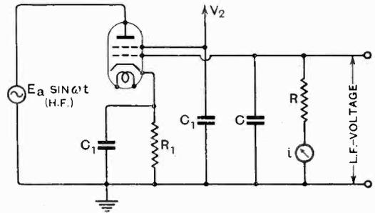
Fig. 8.—Circuit diagram for transit time detector.  $C_1$  are block condensers,  $0.5 \mu F$ .  $R_1$ , bias resistance, about 300 ohms.  $C$ , condenser of  $100 \mu \mu F$ .  $R$ , leakage resistance of about 1 megohm.
