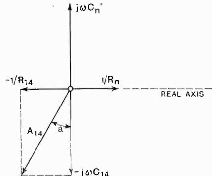
Fig. 2.—Vectorial diagram of admittances between grid one and grid four.
