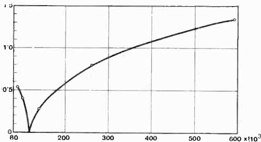
Fig. 4.—Curve for determining the neutralising resistance  $R_n$  of Fig. 3. Vertical: Volts on diode voltmeter  $D_2$  of Fig. 3. Horizontal: resistance values  $R_n$  of Fig. 3 (ohms).
