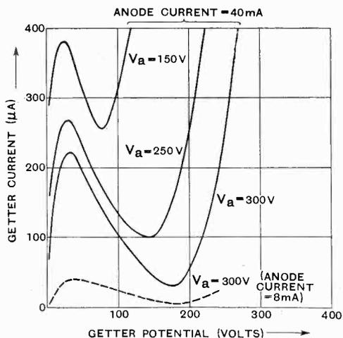
Fig. 4 (Above).—Relation of space-current versus voltage for getter on bulb of pentode.
