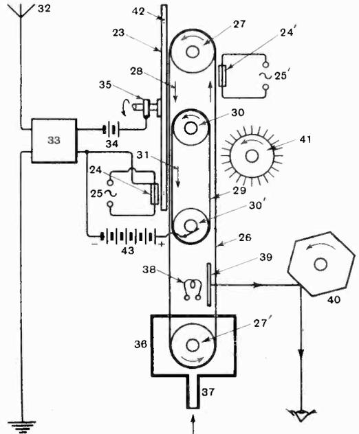
Fig. 5.—Principal arrangement of an electrographic television receiver.
