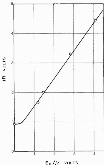
Fig. 9.—Detected volts (vertical), being current  $i$  multiplied by  $R$  of Fig. 8 as a function of the H.F. voltage (eff. volts) for a tetrode valve type RCA 35 with 60 volts on the screen. Wavelength 10 m.
