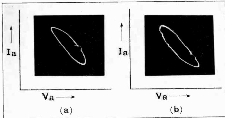
Fig. 1.—Oscillogram of load-curve, showing "Buzz Effect."
