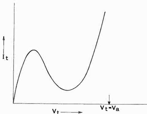
Fig. 3.—Current-voltage characteristic of a secondary-emitter in an electron stream.
