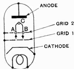
Fig. 6.—Diagram of electron path between grid two and anode of a tetrode valve, causing a transit time d.c. to grid one.
