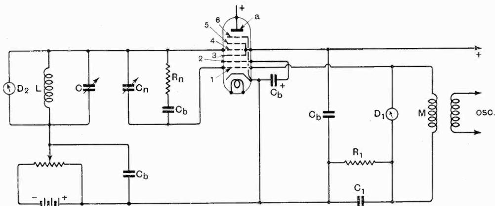
Fig. 3.—Connections of apparatus for measuring admittance between grid one and grid four.  $D_1$  and  $D_2$  are diode voltmeters (acorn type diodes).  $L, C$  parts of circuit tuned to the oscillator frequency.  $C_b$  are block condensers, 20 000  $\mu\mu\text{F}$ .  $C_n$  and  $R_n$  are neutralising capacitance and neutralising resistance.  $R_1$ , leakage resistance of 50 000 ohms.  $C_1$ , capacitance, 200  $\mu\mu\text{F}$ .  $M$ , coil of a few turns, coupled to oscillator.
