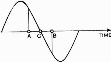
Fig. 7.—Alternating volts on anode of Fig. 6 (vertical) against time (horizontal).
