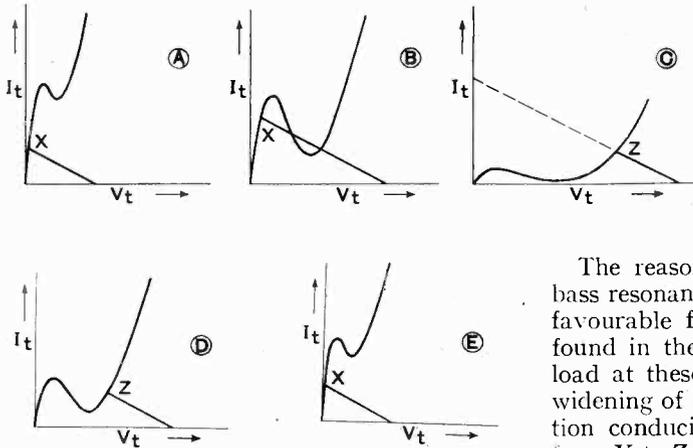
Fig. 6.—Variation of getter potential during an A.C. cycle.
