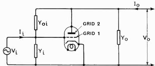
Fig. 5.—Equivalent circuit diagram for measuring the complex transconductance between grid one and grid two of octode.
