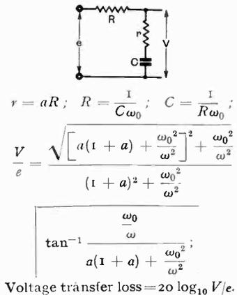
Fig. 6.—Circuit for increasing  $\pi$  attenuation with generalised attenuation and phase shift characteristics.
