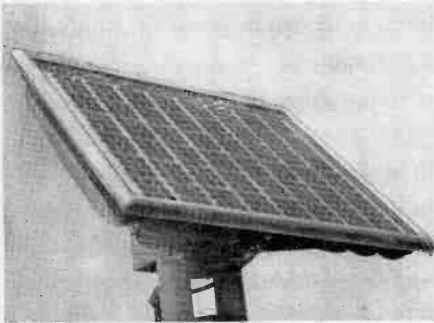
Experimental solar battery comprising 432 silicon discs linked together. Developed by Bell Telephone Laboratories, the individual discs have a diameter of about 0.9 in. and the battery can provide about 20 W output
