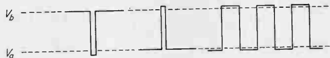
100-c/s signals of equal amplitude but with large, small and unity mark-space ratios
