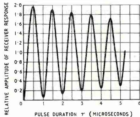
Fig. 4. Variation of amplitude with pulse duration.
