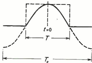
Fig. 4 (above). Pulse comprising one half-cycle of a cosine wave.
