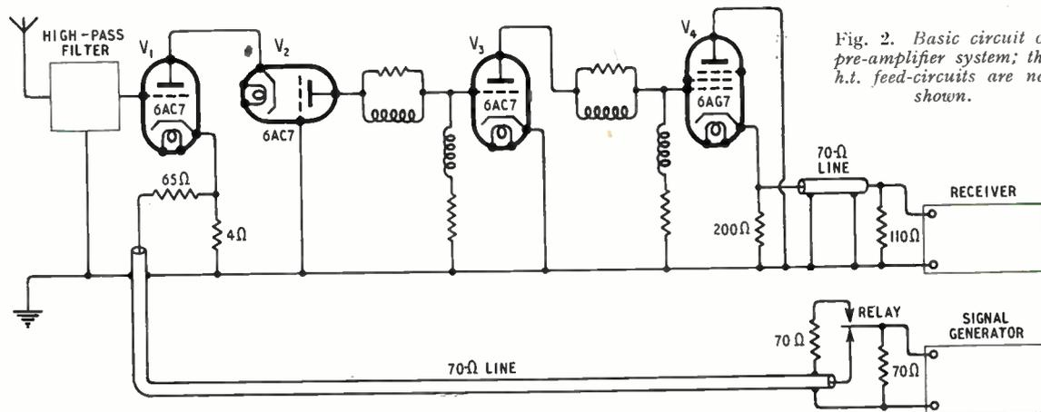
Fig. 2. Basic circuit of pre-amplifier system; the h.t. feed-circuits are not shown.
