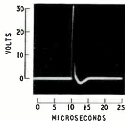
During the second phase of the flip-flop action the grid of  $V_2$  is driven positive, and the tuned circuit is highly damped. The action is the same as for the diode circuit illustrated in Fig. 1(c). The oscillatory
