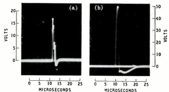
Fig. 7. Typical voltage pulses showing effects of varying coil inductance  $L$ .
