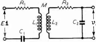
Fig. 2. Equivalent circuit of Fig. 1.
