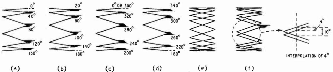
If either  $P_1$  or  $P_2$  is varied the c.r.o. trace changes through the various phases illustrated in the sequence 2(f), 2(e), 2(a), 2(e), 2(b), 2(c), etc. The change from the serpentine 2(a) to the symmetrically-looped figure 2(e) occurs at intervals of  $10^\circ$  phase shift. The change from 2(a) to 2(b) occurs at  $20^\circ$  intervals. In 2(f), a spike is shown superimposed on the figure. This is obtained by by-passing part of the locking spike on to the X-plates.
