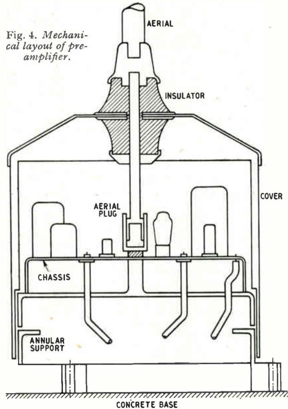
Fig. 4. Mechanical layout of pre-amplifier.
