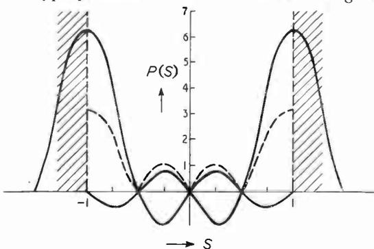
Fig. 12. Component patterns of the polar diagram of the aerial of Fig. 11.
