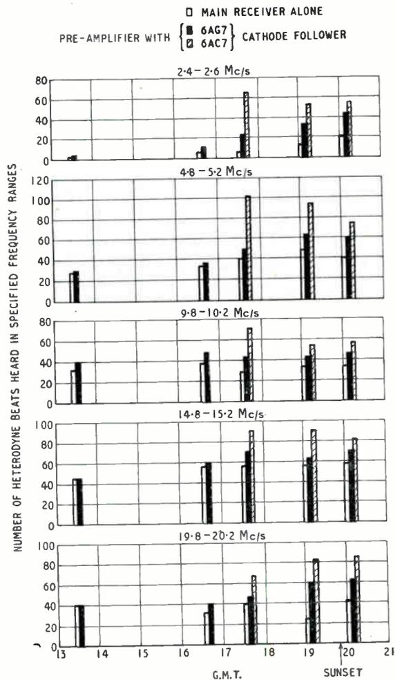
Fig. 6. Intermodulation tests on pre-amplifier.
