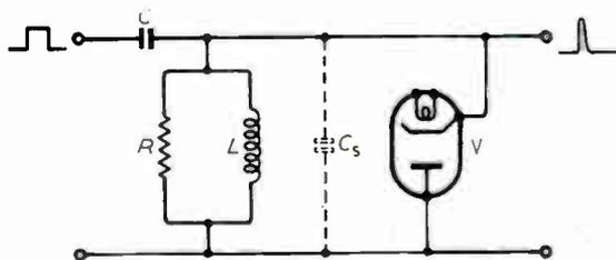
Fig. 1. Production of a short pulse from a sudden positive-going voltage change, with the aid of a highly-damped oscillatory circuit.
