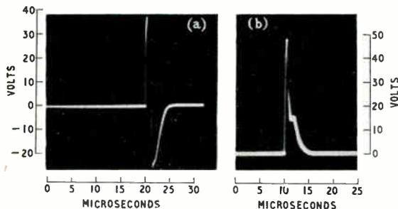
Fig. 6. Typical voltage pulses showing effects of varying cathode-bias resistance  $R_b$ .
