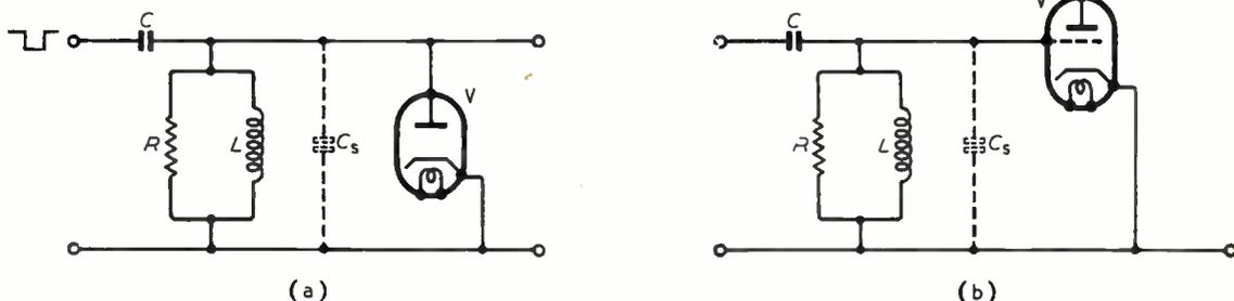
Fig. 4 (right). Circuit arrangement of cathode-coupled flip-flop pulse generator.
