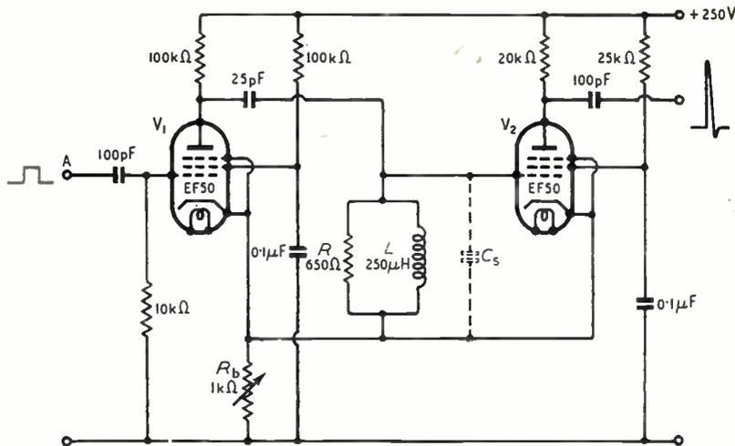
The steepness of the rise depends on the steepness of the input-voltage change, and the steepness of the fall and the duration of the pulse depend on the frequency of the  $LC_s$  circuit.
