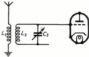
Fig. 1. Aerial tuning circuit of receiver.
