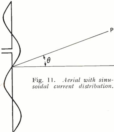
Fig. 11. Aerial with sinusoidal current distribution.
