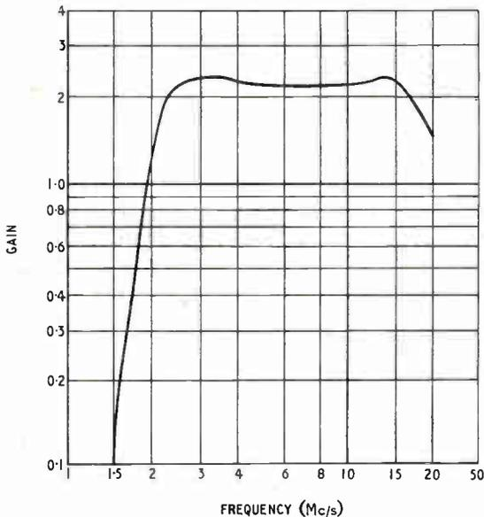
Fig. 5. Gain characteristic of pre-amplifier.
