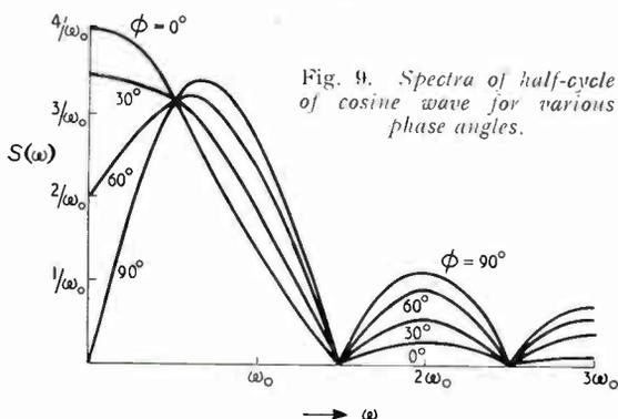
Fig. 9. Spectra of half-cycle of cosine wave for various phase angles.
