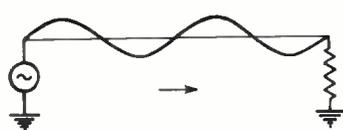
Fig. 14 (above). Two wavelength travelling-wave aerial.
