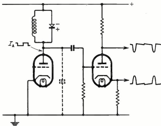
low-capacitance ringing choke and rectifier combination, such as that shown in the figure, will give a better output pulse in nearly all cases.
