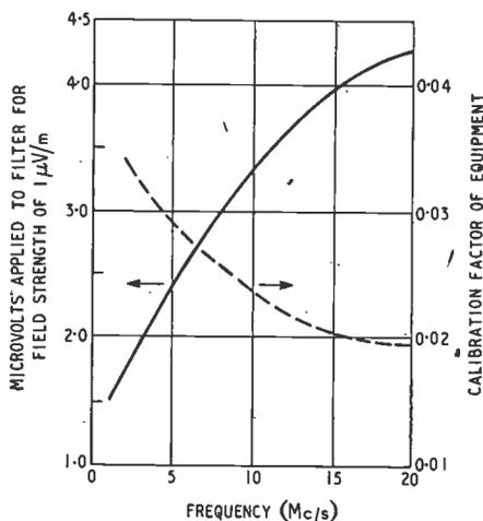
Fig. 3. Pick-up factor of aerial and calibration factor of equipment; aerial length 6.1 m.
