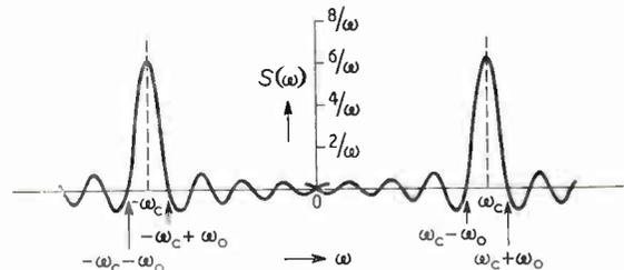
Fig. 2 (above). Pulse modulated by a cosine wave.
