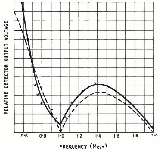
Fig. 5. Variation of receiver output with tuning.
