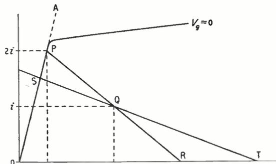
Fig. 6. Basic pentode characteristic.
