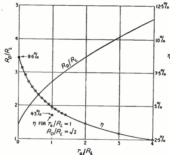
Fig. 4. Optimum  $R_D/R_L$  versus  $r_a/R_L$  and corresponding efficiency  $\eta$ .
