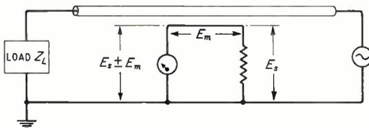
Fig. 4. This diagram illustrates the action of a directional coupler.  $E_s$  and  $E_m$  are the voltages produced by the e.s. and e.m. waves.
