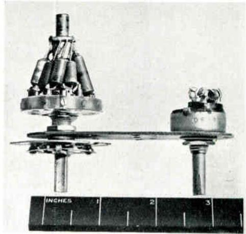
Fig. 9. Turret mounting of resistors.
