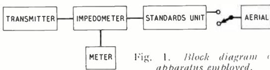
Fig. 1. Block diagram of apparatus employed.
