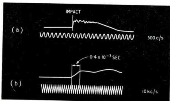
Fig. 4. (a) A reproduction of the photographic trace, showing the velocity-time curve; (b) an enlargement of the part of the trace near the impact.
