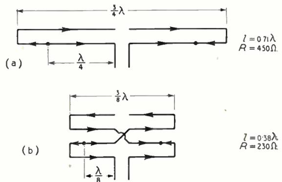
experiments were made with the dipoles horizontal and only about 25 ft above the ground; as  $\lambda/2$  was about 35 ft, it is probable that the results were appreciably affected by the proximity of the ground. The input resistances are from 20 to 30% above the calculated values; the high-frequency resistance of the wires constituting the dipoles is only about 1% or less of the measured values and can be ignored.
