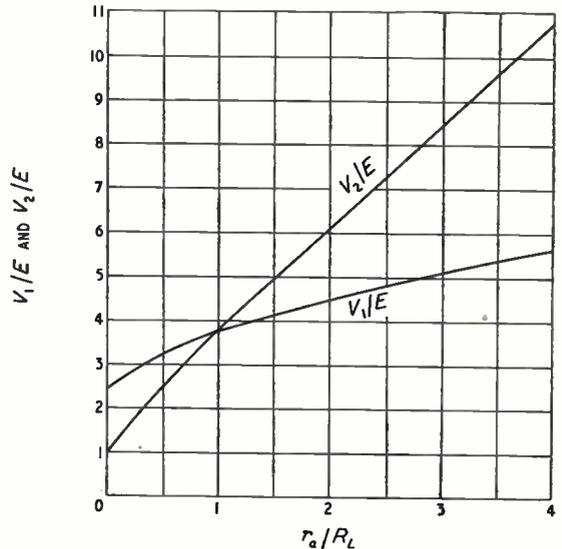
Fig. 5. Optimum  $V_1$  and  $V_2$  versus  $r_a/R_L$ .
