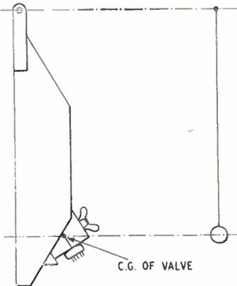
The effect of the inertia of the beams can be eliminated by placing the valves at the centre of percussion of the system. When this is done, the motion of the valve is again that of a small free mass and the size of shock again is  $g/f$ . The easiest way to check the adjustment is to hang the frame from its hinges, as shown in Fig. 2, and verify that the periodic time is the same as that of the bob pendulum shown at the side.
