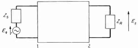
Fig. 5. This diagram defines the notation used in obtaining the insertion ratio.
