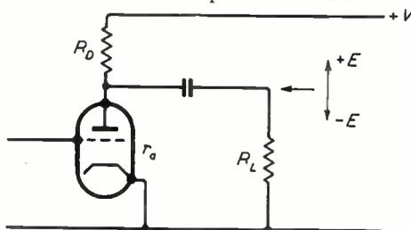
Fig. 1. RC-coupled stage.
