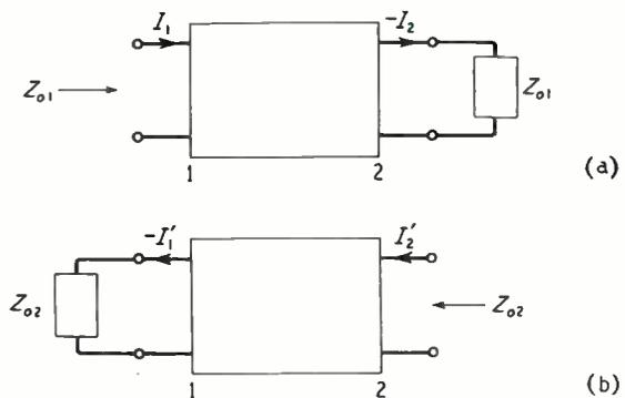
Fig. 2. Iterative propagation function of network driven at end 1(a), and driven at end 2(b).
