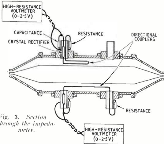
Fig. 3. Section through the impedometer.
