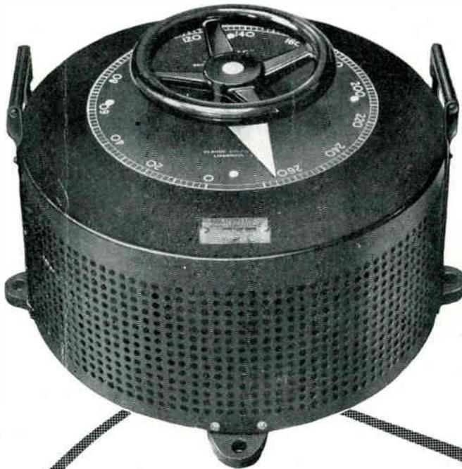
With a 'VARIAC' voltages are instantly and minutely adjustable from 0-Line Voltage, or in some cases up to 17% above line voltage. Type 50-B 'VARIAC,' as illustrated left, is often operated in a 3-gang assembly on 3-phase work to control 21Kva.
