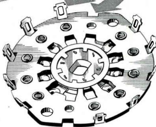
**N**OTE how the NSF/Oak switch contacts are positively located and secured by the locking slots around the edge of the wafer. Only NSF/Oak rotary wafer switches are available with this unique feature, which definitely eliminates the misalignment of contacts loosened by heat during soldering, and therefore only NSF/Oak switches, with the 'D' feature, provide a satisfactory solution to a troublesome problem.
