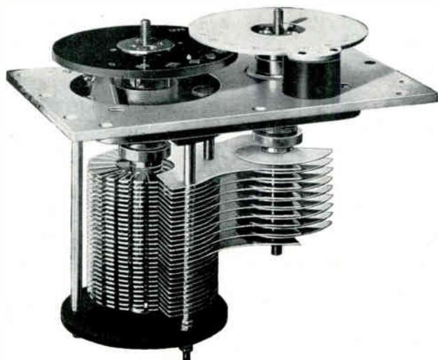
introduced in a manner such that small angular movements, due to a possible uncertainty of click positioning, produce only very small edge capacitance changes on one sector only—in no position is there the slightest change of coincident active plate area.
