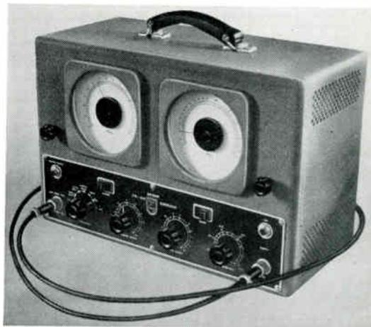
Philips FM-AM generator, type GM 2889, covering 5-225 Mc/s. On f.m. a deviation up to 10 Mc/s is obtainable. A marker oscillator is included and the apparatus is suitable for use with an oscilloscope to depict the bandpass curve of a television receiver.
