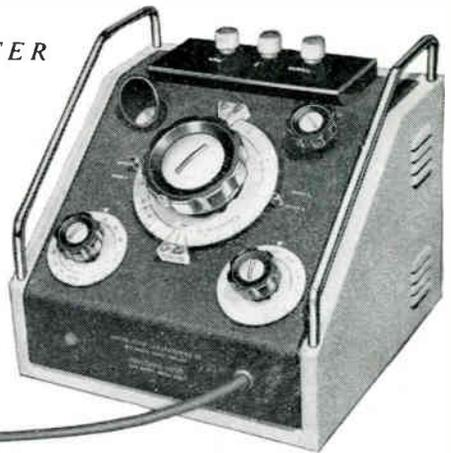
*The Wayne Kerr* Inductance Meter uses a stable variable frequency oscillator to resonate the unknown inductance with a known capacity. Calibration and scale reading accuracy are sufficient to give direct reading within  $\pm 2\%$  for values above  $1 \mu\text{H}$  and relative measurements can be made with even greater accuracy.
