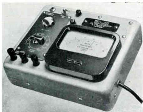
(above) Cossor model 1433 voltage calibrator for oscilloscopes.
