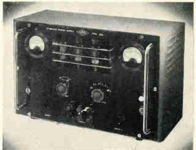
**THIS** unit provides a stabilised direct voltage, continuously variable from 200-350 volts, which may be used with either the positive or negative lines earthed, or with the output floating. An unstabilised alternating supply of 6.3 volts, the centre top of which may be strapped to earth, is also available.
