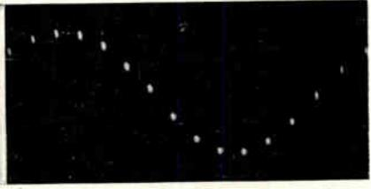
Fig. 4. Trace obtained with a 10-kc/s input signal, frequency-modulated at 1 kc/s with 56-c/s deviation.
