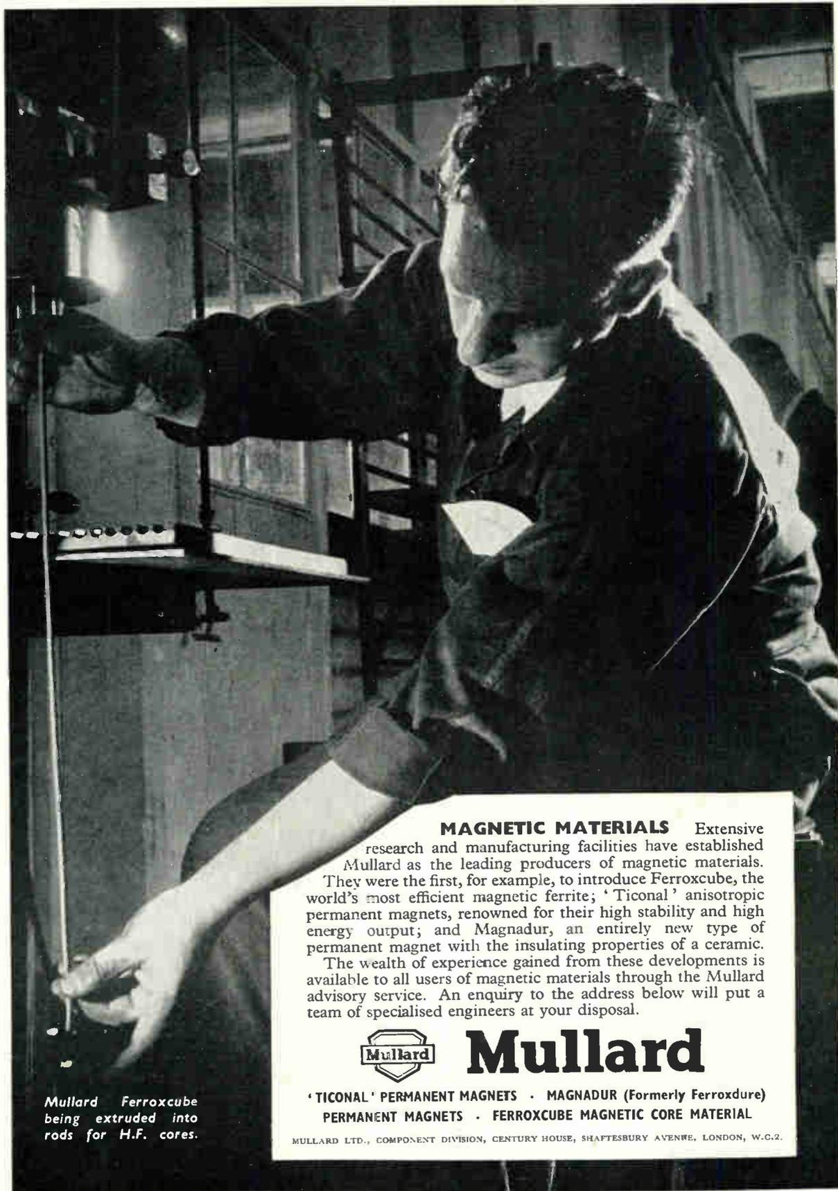
Mullard Ferroxcube being extruded into rods for H.F. cores.
