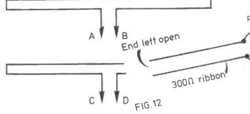
2 seperate feeders, 3000 ribbon, or open AB wire of identical length to switching unit in FIG. 11
