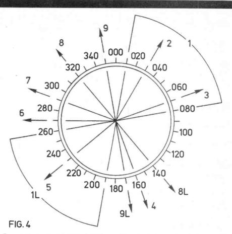
Approximate great circle bearings, from the UK, to principal areas of amateur activity. Check the number on the bearing and locate that number on the appropriate table against time of year and time (GMT) to find optimum propagation period for that area. Remember that the 28MHz band is subject to large variations linked to the sunspot cycle.
