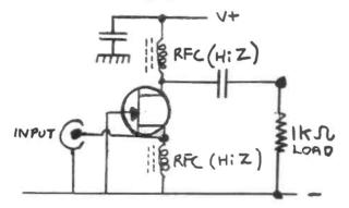
What is the effective input impedance at its source terminal: a. 10 ohms, b. 20 ohms, c. 50 ohms, d. 100 ohms
