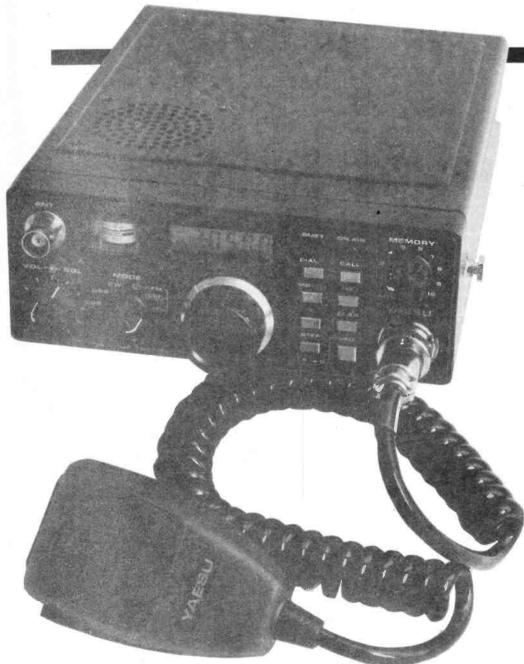
Actually, 'all-mode' is a slight misnomer — multimode would be more appropriate as the 790R does not provide AM (or FSK). What it does give you is SSB (upper and lower), CW and FM, together with a lot of facilities to help you find the activity on the wide open plains of 70cm.
