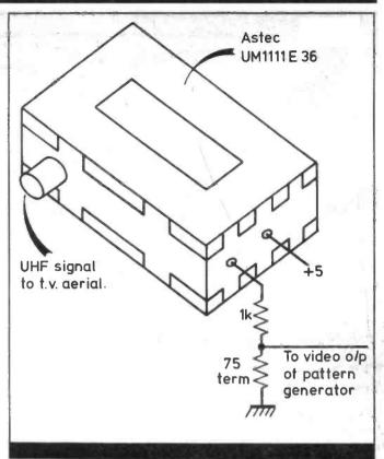
Although the module shown here in many ways forms the basis of an ATV station — the sync function is fundamental to operation — it can be used as an independent piece of test gear by hooking the video output into a UHF modulator of the home computer type. It also enables testing of the board with a domestic TV
