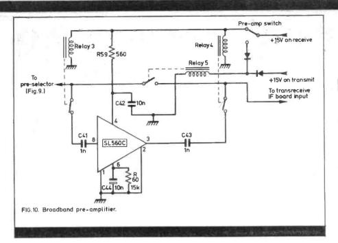
The maximum frequency tunable with the arrangement as shown is about 35MHz.
