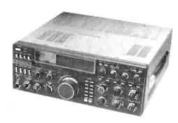
**TS 930.** Superb high performance, all solid state HF transceiver, capable of operating in the SSB, CW, FSK and AM modes, on all amateur bands (160 to 10 metres). Incorporating a general coverage receiver. Built-in ATV is an optional extra.
