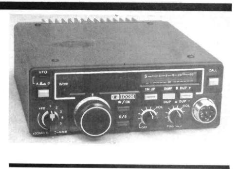
144MHz, with the other response removed by the receive helical filter. Three stages of driver amplification follow, thence to a hybrid PA stage, delivering a stated 25W to the antenna via diode TR switch and low pass filter. While a hybrid stage is convenient for the manufacturers, it may not be such a good idea in the event of it needing replacement.
