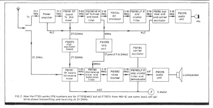
3.18MHz dependent on which sideband has been selected. These two sidebands are applied to PB1183 where the wanted side band is amplified, the unwanted sideband being suppressed by the crystal filter.
