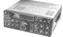
TS 930. Superb high performance, all solid state HF transceiver, capable of operating in the SSB, CW, FSK and AM modes, on all amateur bands (160 to 10 metres). Incorporating a general coverage receiver. Built-in ATV is an optional extra.
