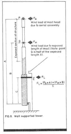
the structure due to the wind loads. This would have been taken into account and a suitable safety factor allowed by the manufacturer. However, as long as the specified head loads etc., are not exceeded and the correct procedure followed force will still affect the wall. The simplified formula:
