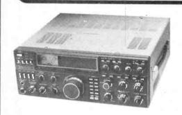
**TS 930.** Superb high performance, all solid state HF transceiver, capable of operating in the SSB, CW, FSK and AM modes, on all amateur bands (160 to 10 metres). Incorporating a general coverage receiver. Optional extras:—Built in A.T.U.
