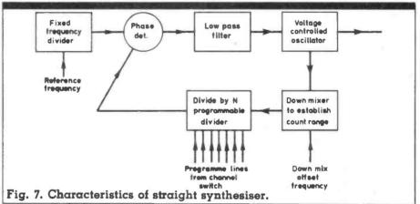
455kHz receiver IF. This is now derived by programming the device to read 91 steps which at 5kHz intervals is 455kHz and then mixing this slight tweak to the 10.240 crystal then brings the resultant frequency to within 1-200 cycles of 27.60125. Similar techniques will permit the
