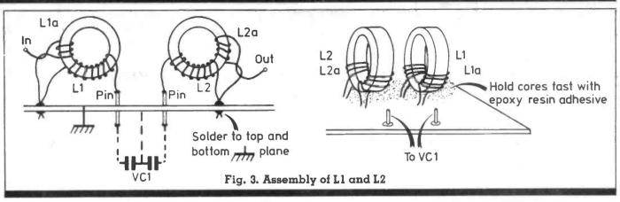
round the rest of the board, soldering up one oscillator section at a time. Again keep leads as short as possible, and orientate bodies of vertical mounting resistors in the positions shown.
