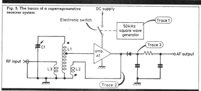
oscillator and the second is a means of detecting the presence of RF oscillations in the system. In practice, the quenching may be done by a secondary oscillatory loop switching on and off the first one. Similarly an RF oscillatory state may be detected by the non-linearity of the oscillator transistor itself, ie looking for a change in collector current with oscillation.
