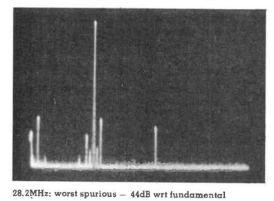
Spectrum analyser photos showing spurious outputs on each band at nominal rated output power. Vertical deflection 10dB/ div; horizontal deflection 10MHz/ div.
