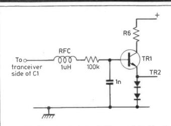
Fig. 5. Modification for full switching with the FT290
