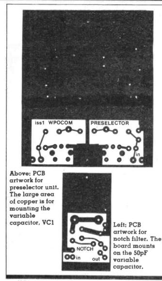
VCl goes in last. The lugs at the rear of the stator plates are inserted through the large holes in the PCB until they just protrude from the underside, then soldered, making sure that the capacitor is exactly at right angles to the board. A still piece of 18 or 20 swg wire then links the earth terminal on VCl to the hole provided on the PCB.
