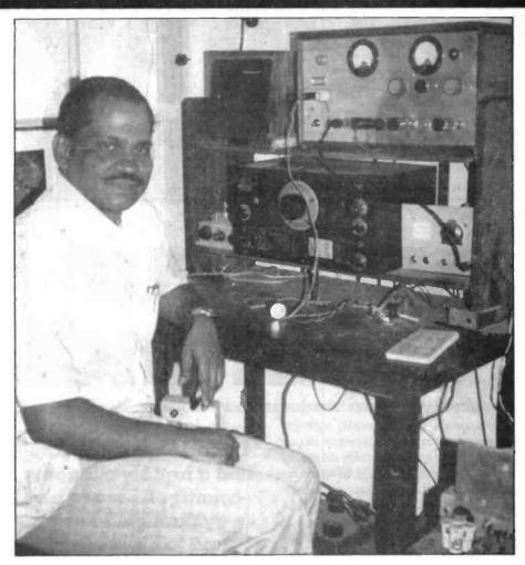
The vast majority of amateur radio stations in India use converted military receivers and homebuilt transmitters such as this setup in Kodaikanal
