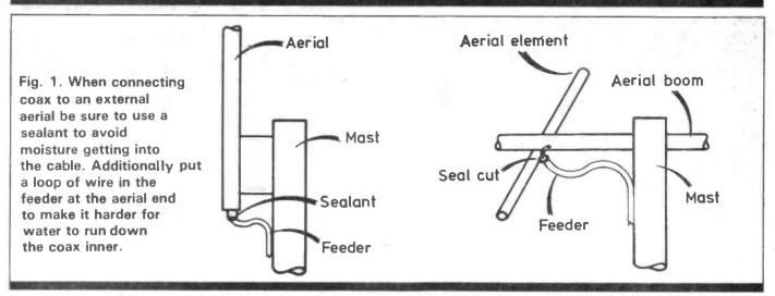
moisture enter the feeder as comparatively small amounts accumulating over the years will slowly but steadily build up the losses to a point where the cable becomes unuseable and has to be replaced which can become very expensive if some of the low loss types of feeder are used. If these precautions are observed then not only should events like those that I have just recounted be avoided but also the life of the feeder should be extended.
