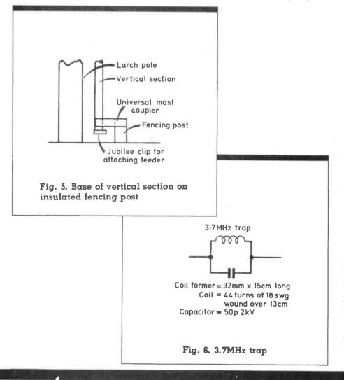
at the base of the larch pole, the vertical section of the aerial was walked upright and the halyard pulled taut. The halyard was then wound in spiral fashion around the vertical section and larch pole, about ten times, and secured at the base of the larch pole. This arrangement stood three seasons of spring gales before being dismantled still intact.
