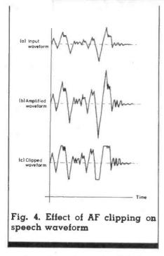
As well as harmonic distortion, there is intermodulation distortion produced whenever two or more signals of different frequencies are passed through a non-linear stage. Sometimes in-band components can be generated from intermodulation between an in-band and an out-ofband component, or from two out-ofband components. For example, an 8kHz and a 6kHz signal could mix to produce a 2kHz intermodulation product. This is one reason for filtering the input as well as the output.
