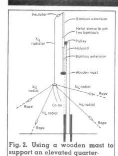
mended and the top of the aerial can be anchored to a strong bamboo extension drawn up by a halyard attached to the top of the wooden mast. The writer uses two 5m bamboo's inserted into a 2m long aluminium tube to give an effective
